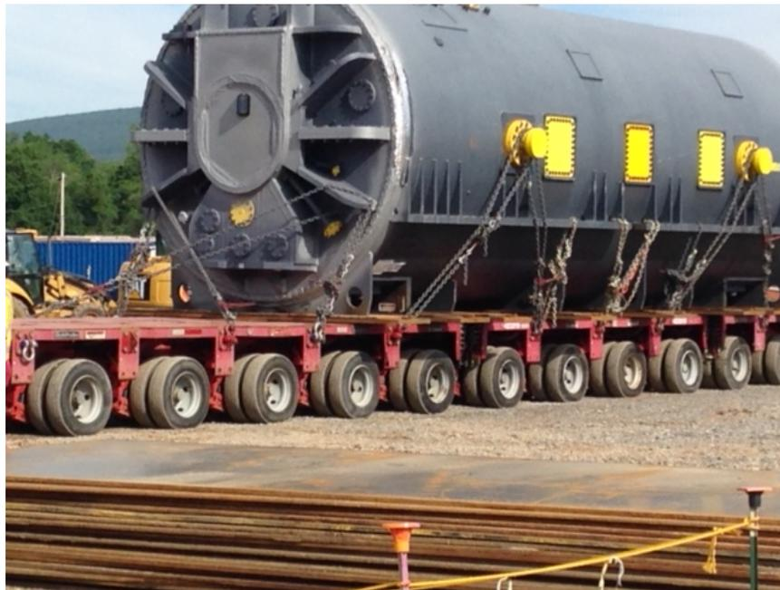
SPMT loaded with power generator ex. of heavy move
