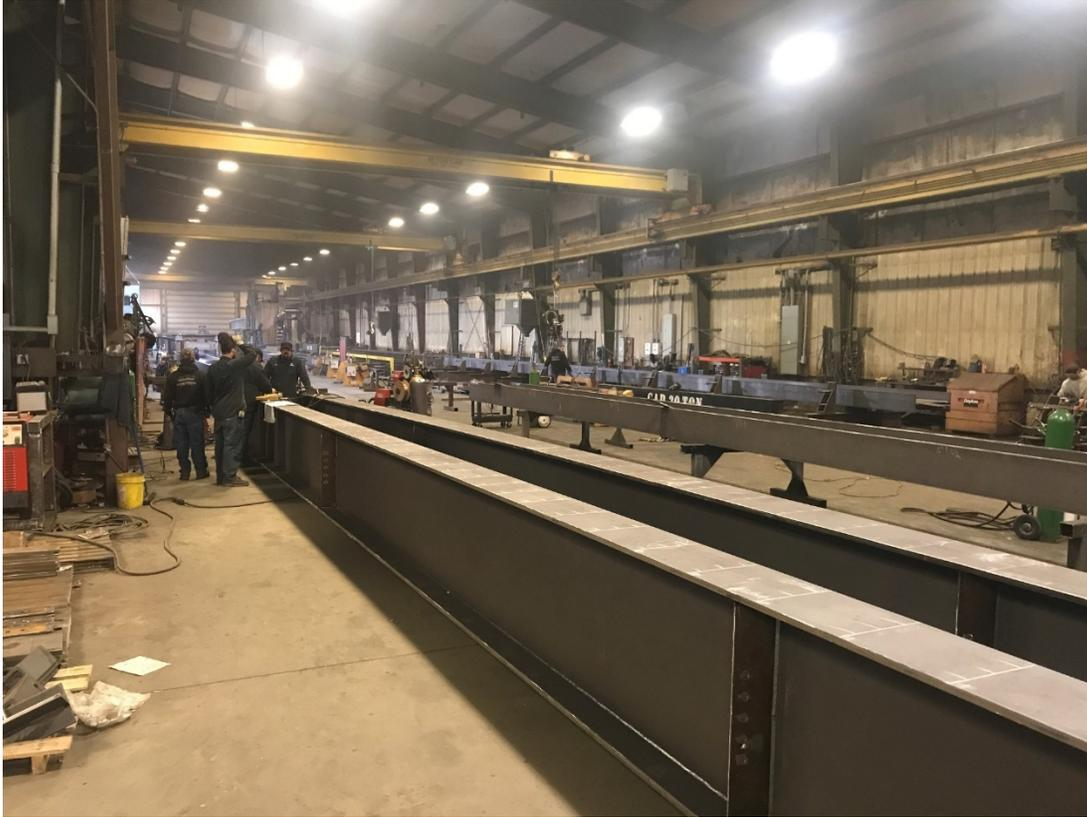
The raw steel will be delivered to the fabrication yard. The pieces will be brought into the shop for cutting, welding, and cleanup. Each piece will be given a distinct piece mark and erection/bolt up drawings will be provided to detail the sequence and layout each piece must be placed in the structure to ensure proper fit. Protective and architectural coatings will be shop applied as a last step in the fabrication process.
