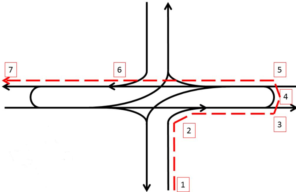
Figure 24. Example of experienced travel time at an RCUT intersection
