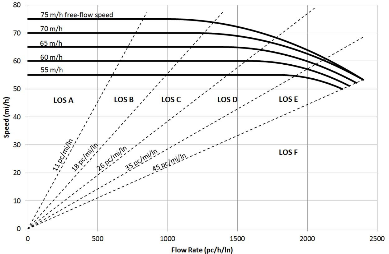
Figure 9. Basic Freeway Segment Speed-Flow Curves
