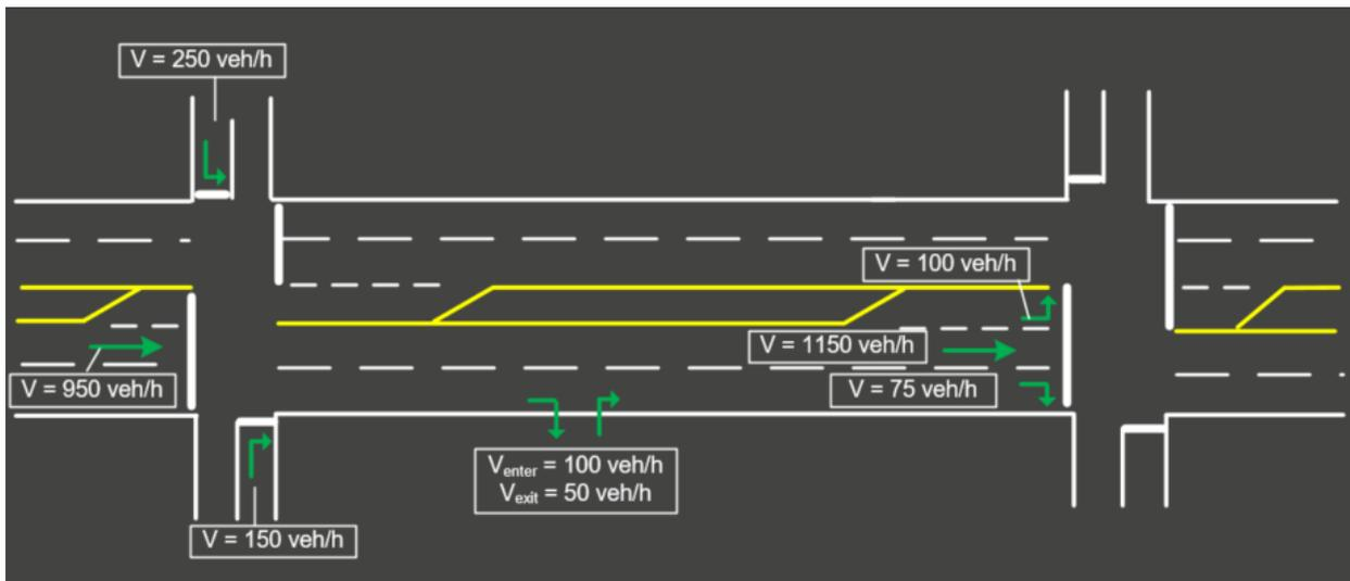
Figure 18. Right-turn-on-red vehicles incorporated into volume-balancing method
