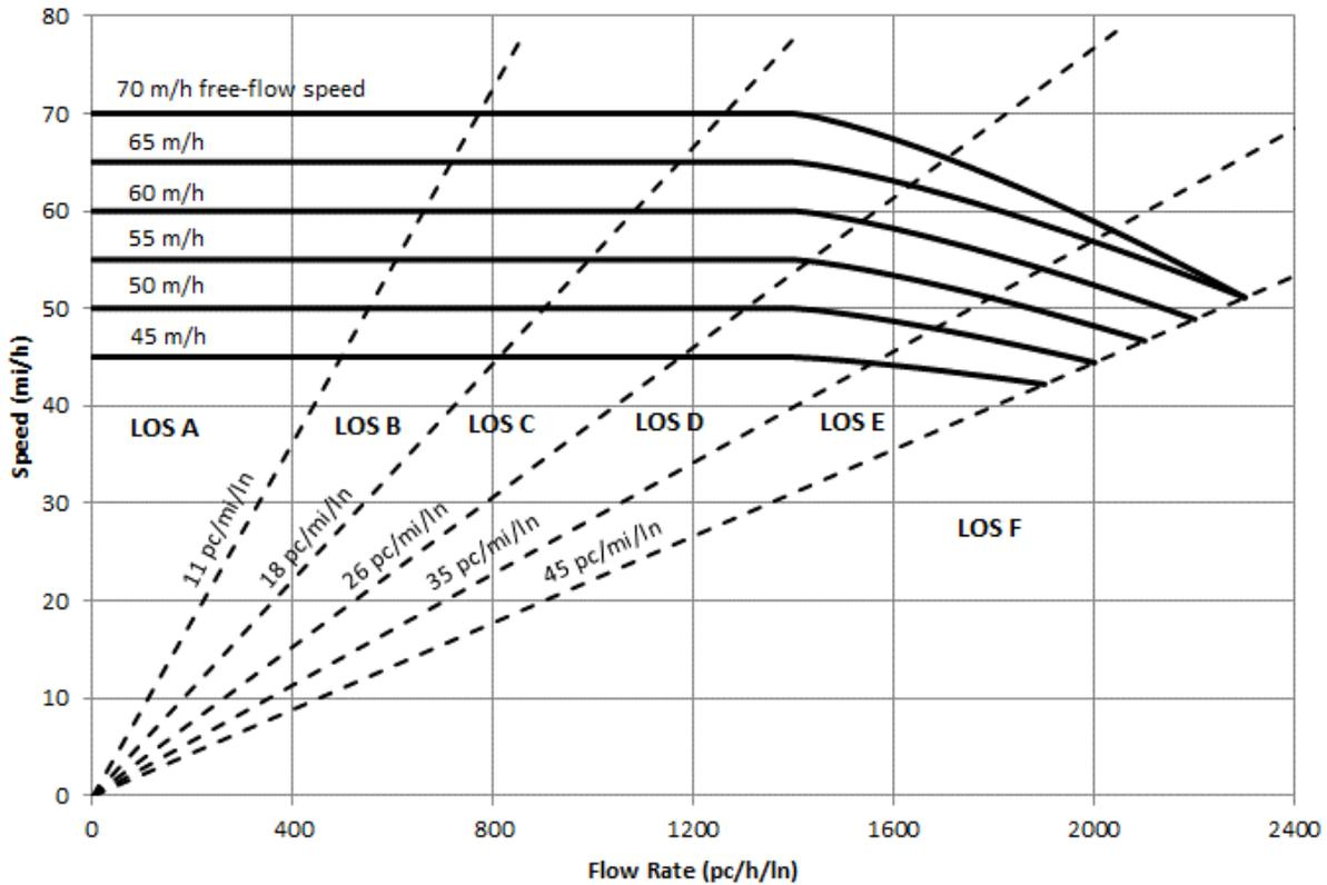
Figure 10. Multilane Highway Segment Speed-Flow Curves
