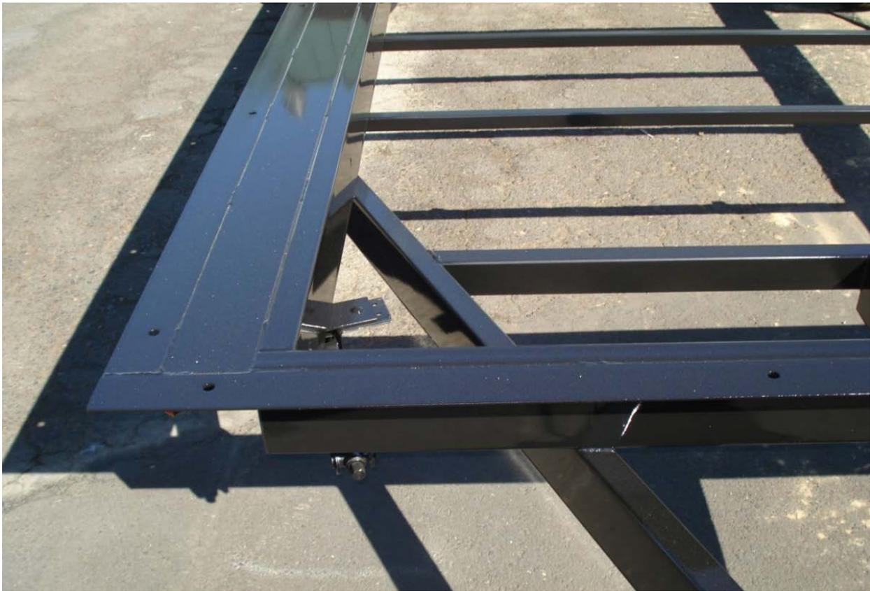
**You can see large structural members on the perimeter, pre-drilled holes for connecting walls to the trailer frame, small interior structural members, and room for floor framing below trailer deck. The steel angles welded to the steel tube(s) forming the perimeter frame are great for placing the exterior walls on, but there is one negative tradeoff – plumbing drains must go through the floor adjacent to the exterior walls, not in the walls as they normally would.**
