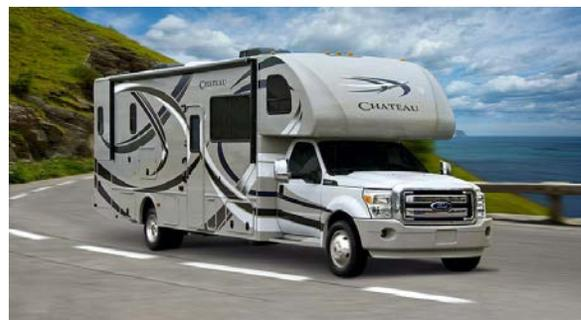
**Right: Class C motorhomes are built on a truck chassis and have living space that extends over the cab of the truck (Credit: Motorhomes/Wikimedia Commons/CC-BY-SA3.0)**
