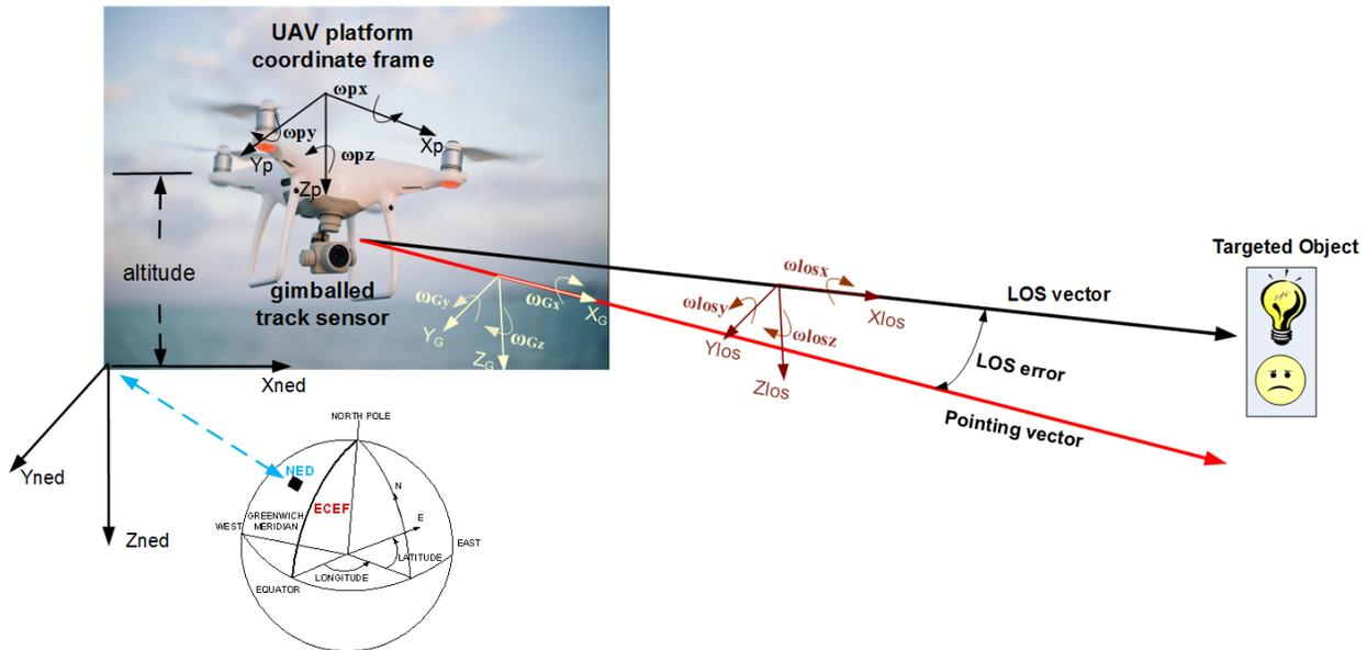
Figure 9.0 Typical coordinate frame geometry for geo-location
