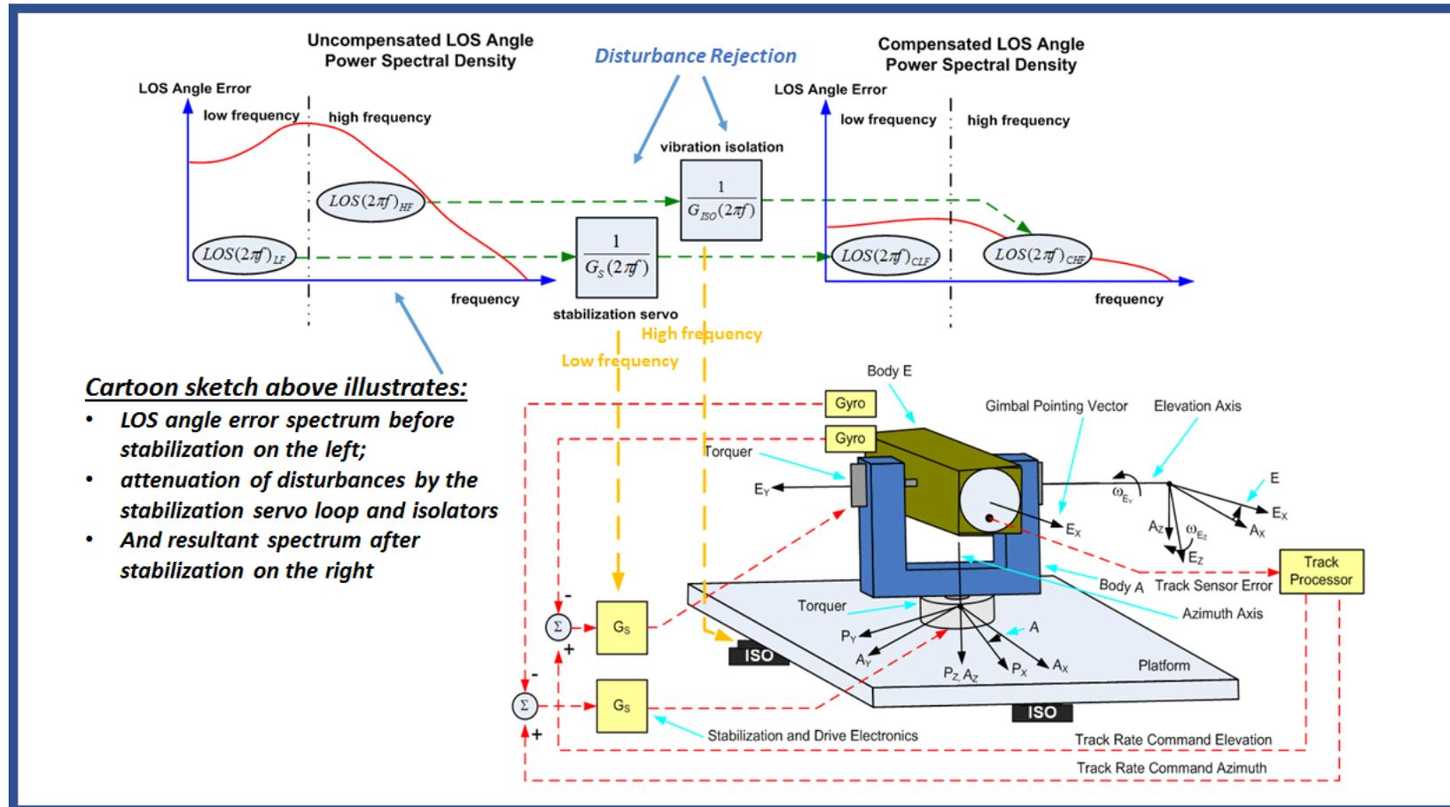
Figure 5.0 SLC System Disturbance Rejection
