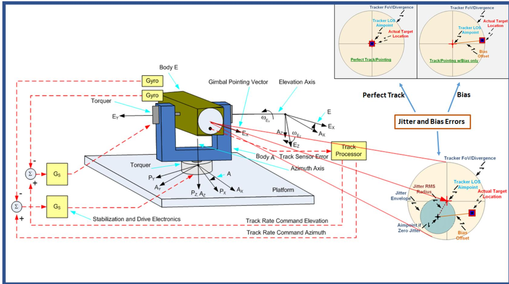
Figure 6.0 Illustration of Jitter and Bias Pointing Error
