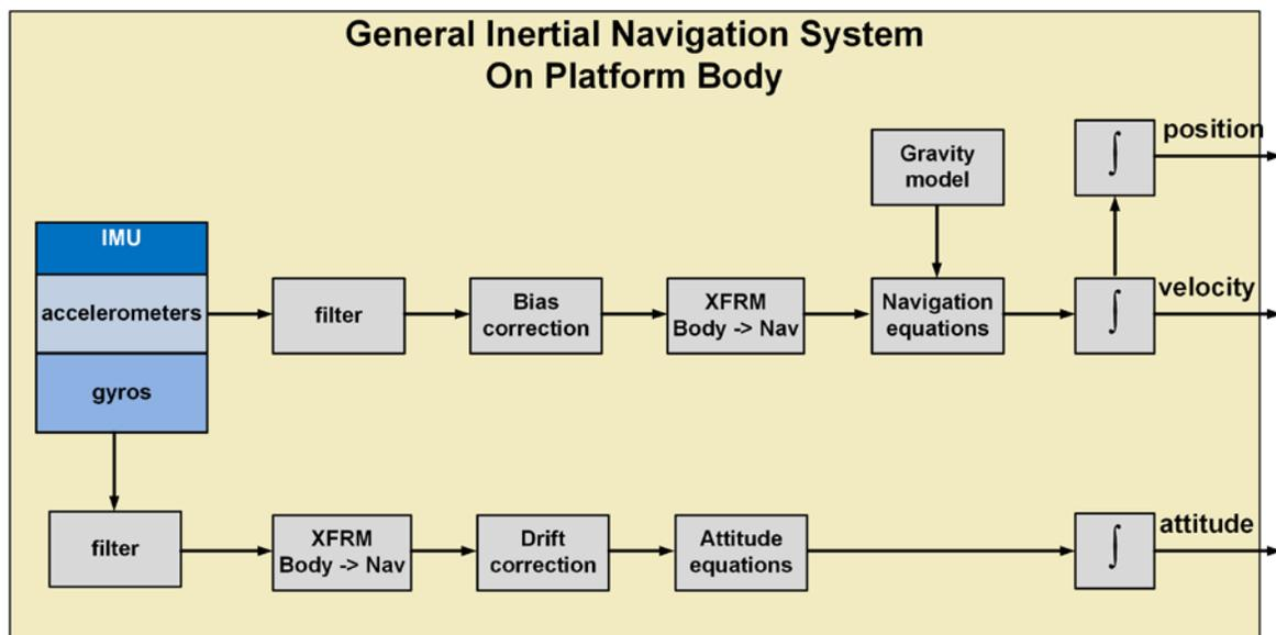
Figure 8.0 INS Simplified Block Diagram
