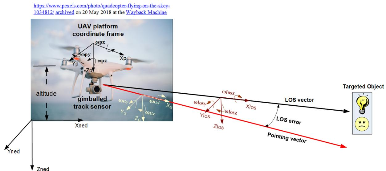
Figure 1.0 LOS Pointing Geometry
