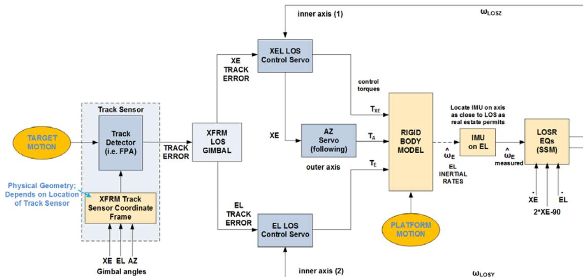
Figure 4.0 Typical Three Axis Gimbal Control Architecture
