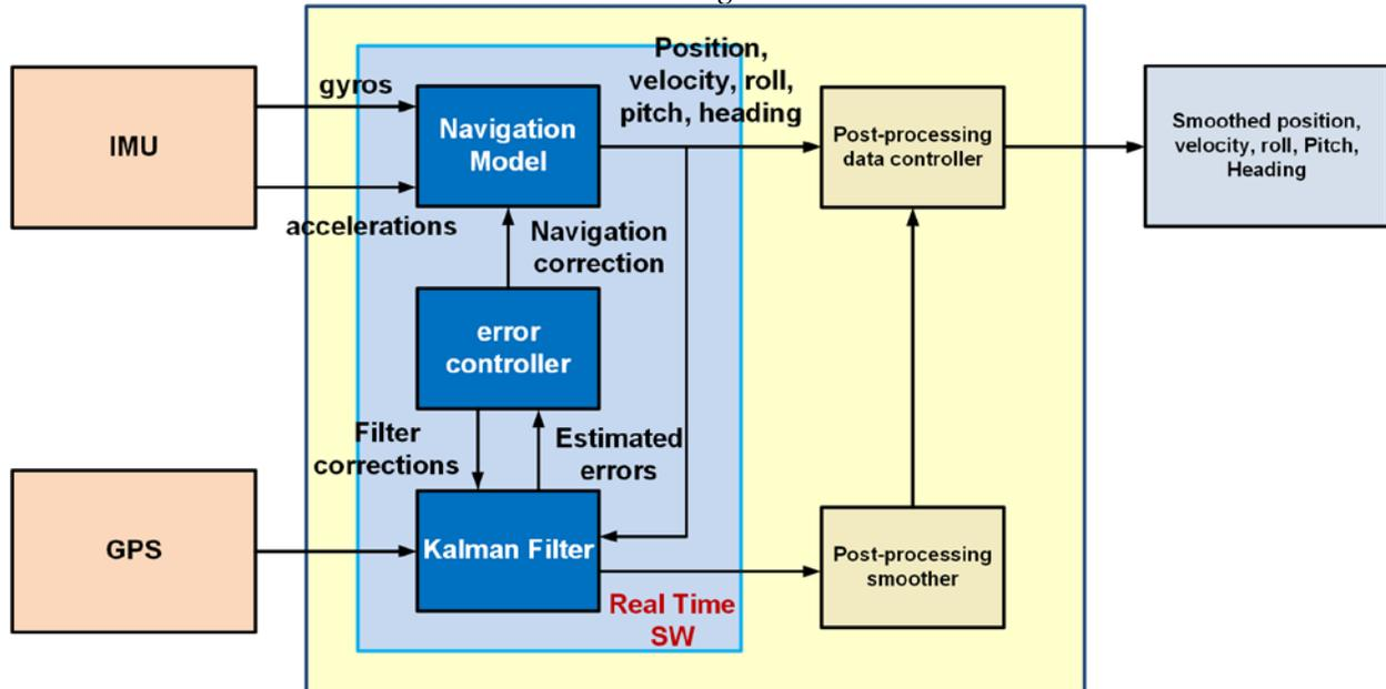
Figure 11.0 [7] High Accuracy Inertial Data for Direct Geo-registration
