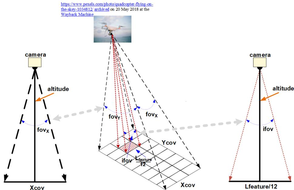
Figure 5.0 Ground Sampling Geometry
