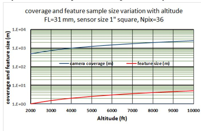
Figure 6.0 Feature sample size (nominal design 1 m) and coverage variation with altitude
