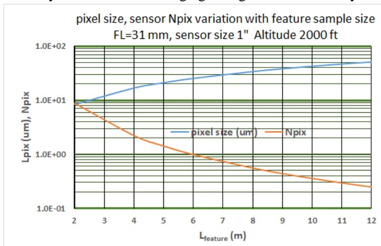
Figure 8.0 Pixel size and Npix variation with feature sample size
