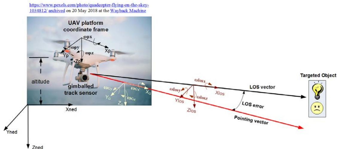
Figure 1.0 LOS Pointing Geometry
