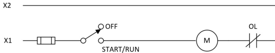
*Figure 3: Two-Wire Control Circuit*
