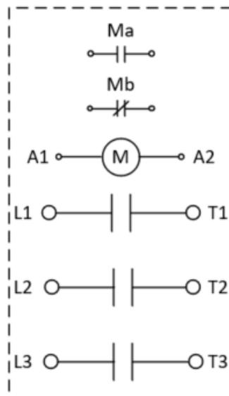
*Figure 2: Contactor Terminal Identification*
