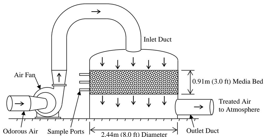
Figure 8: Schematic diagram of the activated carbon system.
