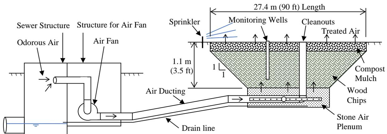
Figure 9: Schematic diagram of the biofilter bed system.
