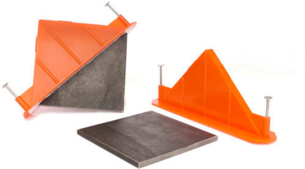
Fig. 30b - Square dowel to be placed at a construction joint placed in insert that was set into first concrete pour, with second concrete pour to follow (<https://www.pna-inc.com/products-designs/diamond-dowel-system>)
