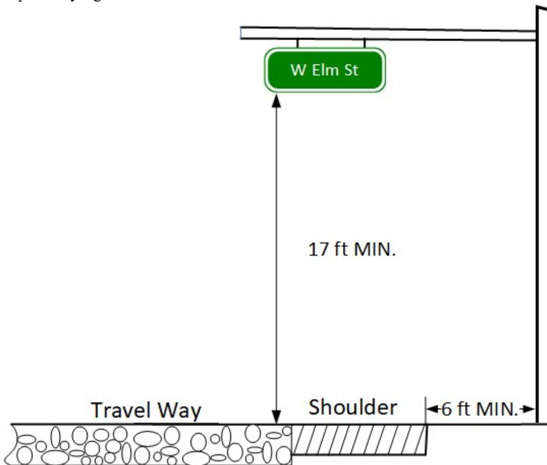
Figure 17. Overhead sign support lateral placement
