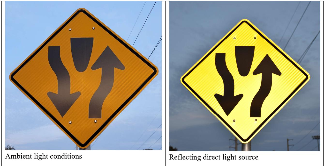
Figure 4. Example of retroreflection sign material
