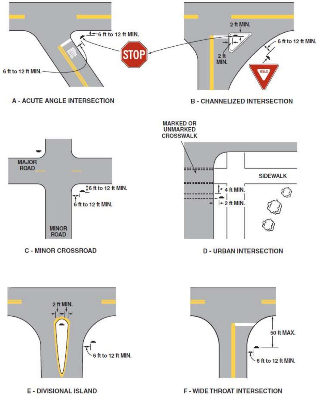
Note: Lateral offset is a minimum of 6 feet measured from the edge of the shoulder, or 12 feet measured from the edge of the traveled way. See Section 2A.19 for lower minimums that may be used in urban areas, or where lateral offset space is limited.
