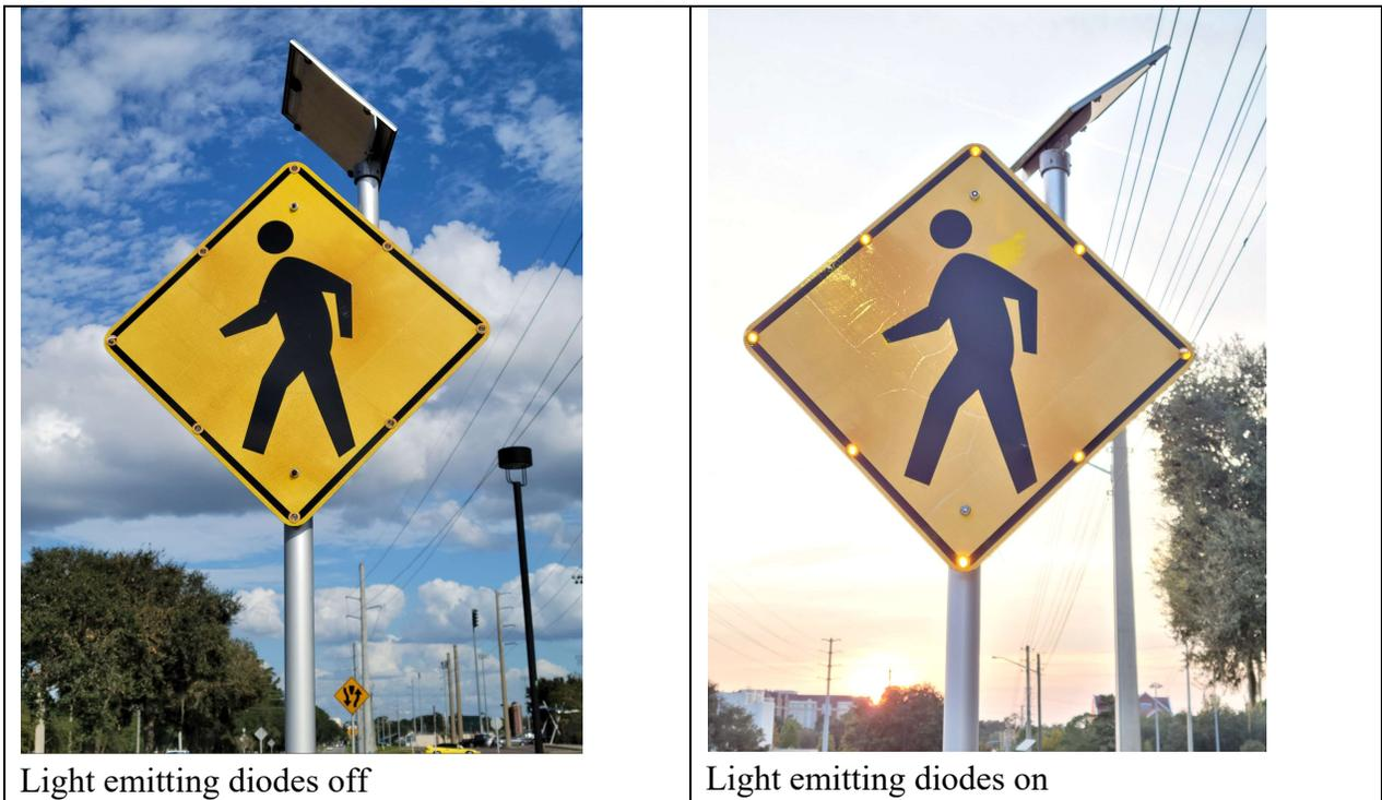
Figure 10. Flashing light emitting diode (LED) units
