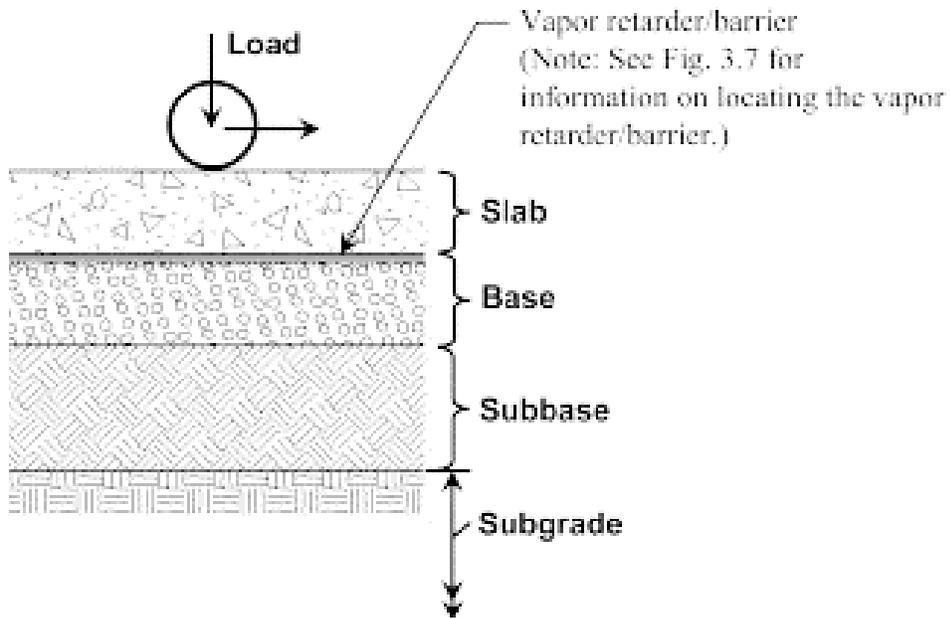
Fig. 29 – Slab-on-grade profile with soil– ACI 360
