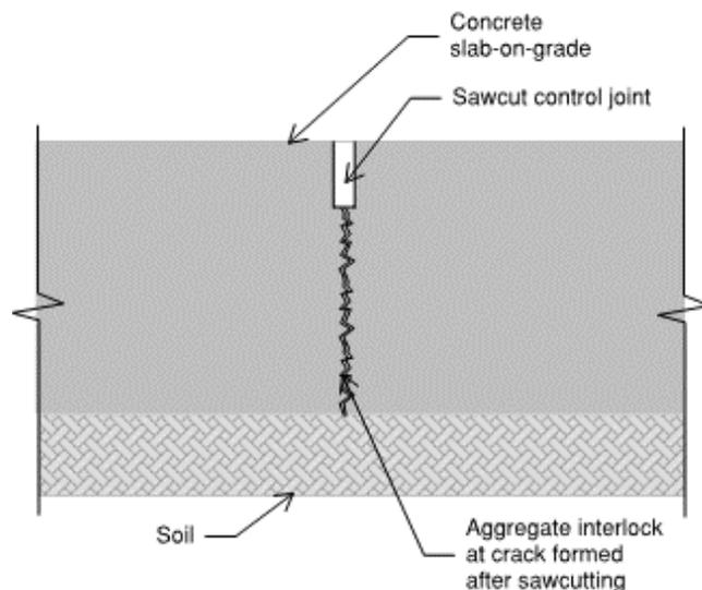
Fig. 34 – Aggregate interlock
