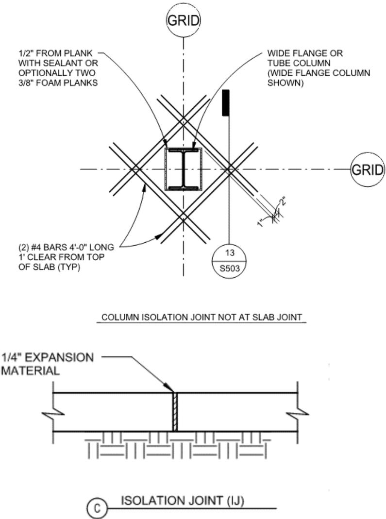
Fig. 49 - Details for typical isolation joints
