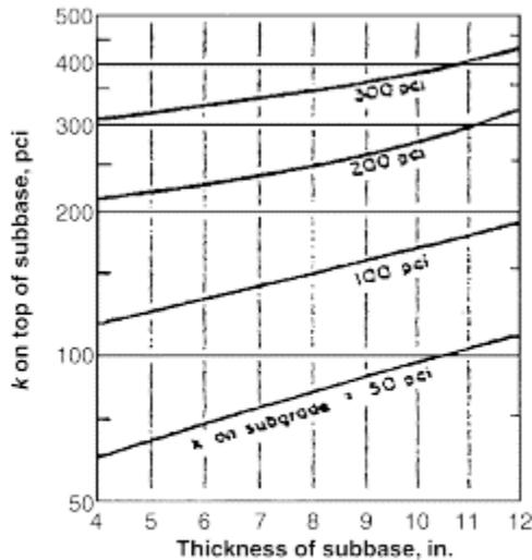
Fig. 3.6—Effect of subbase thickness on design modulus of subgrade reaction. (Note: 1 pci = 0.2714 MN/m<sup>3</sup>; 1 in. = 25.4 mm.)
