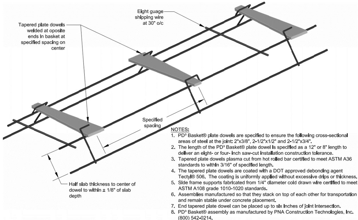
Fig. 43 - Tapered dowels by PNA (PD<sup>3</sup> Basket dowels)
