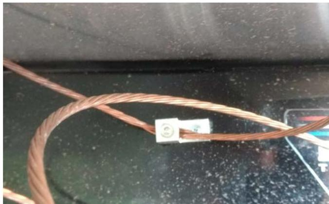
**An aluminum lug attached to steel trailer frame. The ground wire passes through the lug.**
