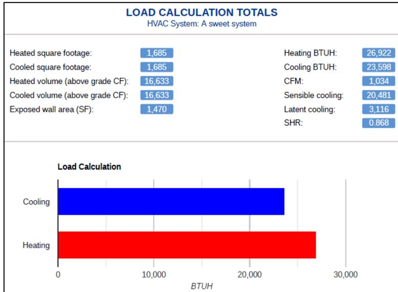
**Figure 1: Excerpt from Sample Manual J Report from a 1,685 ft<sup>2</sup> house (from coolcalc.com)**
