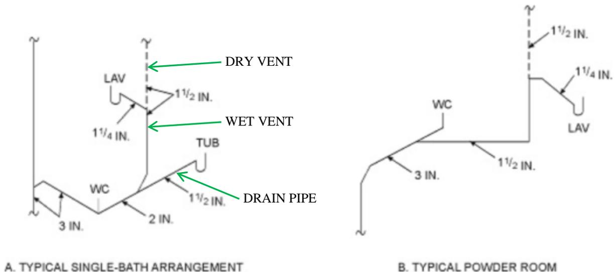
**Figure 4: Two typical bathroom DWV isometric drawings (from 2018 IRC Appendix N)**
