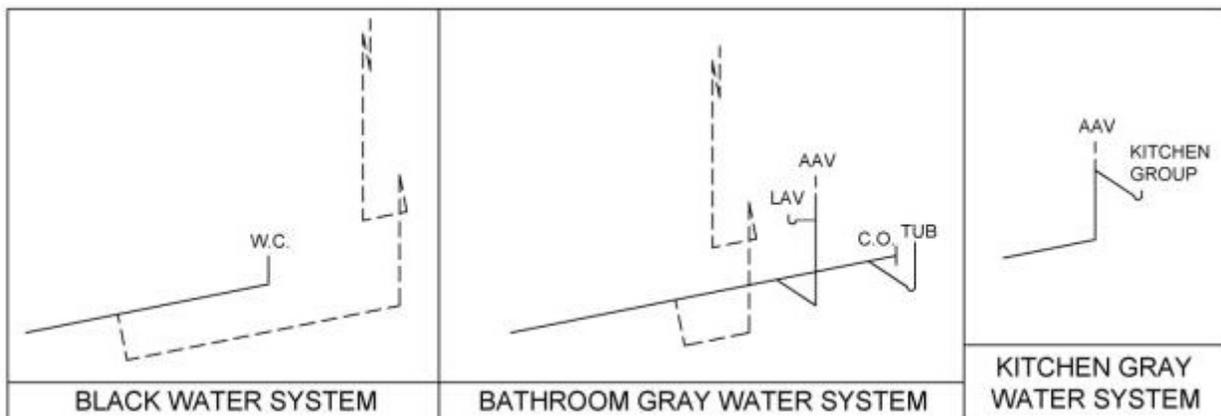
**Figure 5: DWV Sizing Example Isometric Layout**
