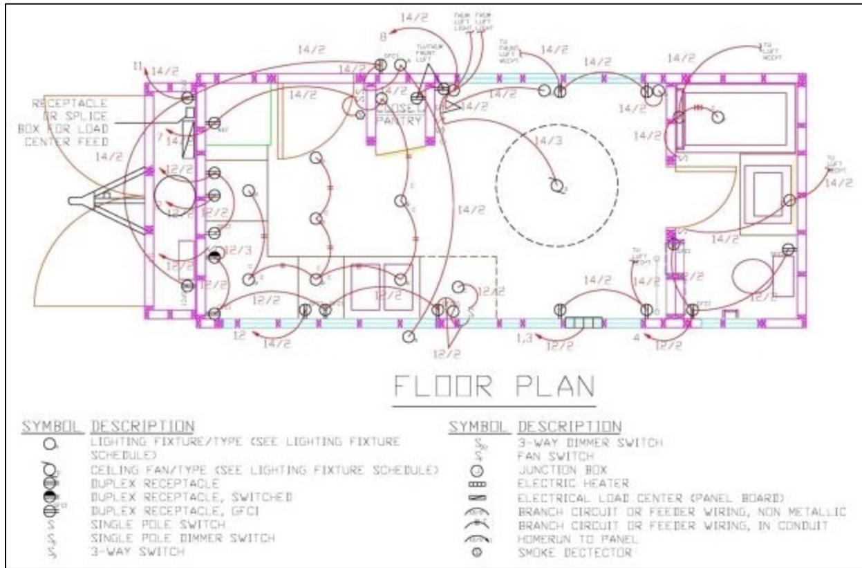
**Figure 10: First floor electrical plan for a THOW**
