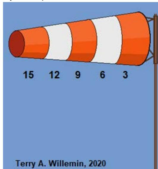
**Figure 11**, A windsock in a 15 knot or higher wind. The numbers represent windspeed estimates needed to inflate the corresponding section.
