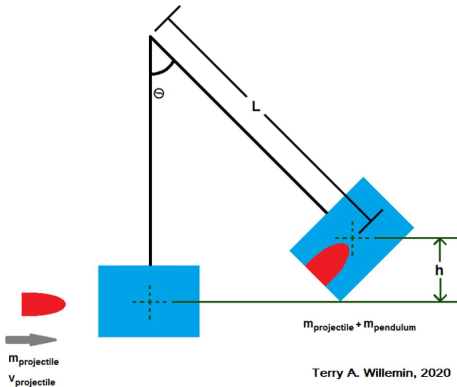
**Figure 21**, Simplified schematic of a ballistic pendulum
