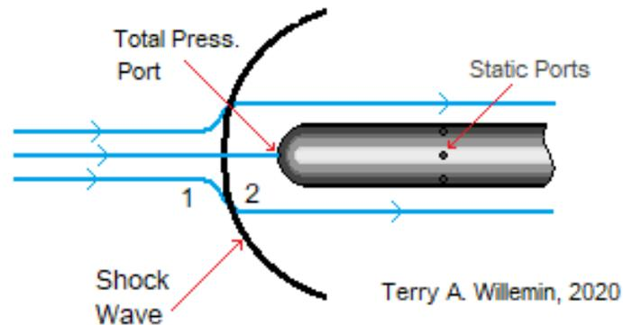
**Figure 10**, A pitot-static tube in a supersonic flow. A detached bow shock forms upstream of the probe tip. The streamlines are shown to approximate flow paths through the shockwave. The pressures located at points 1 and 2 are referenced in Equation 6 below.
