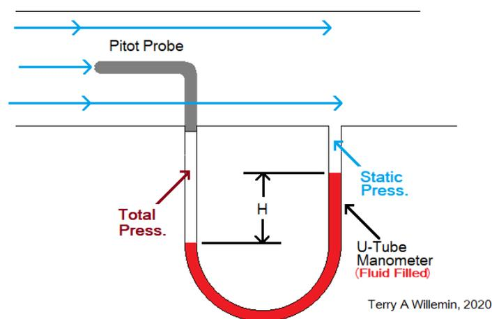
**Figure 8**, U-tube manometer example when used to measure pressure difference between static and pitot/total/stagnation pressures. The stagnation pressure is obtained from the pitot tube. H is the height difference in the manometer created by the pressure difference.
