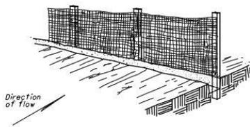
**Silt Fence Installation**
