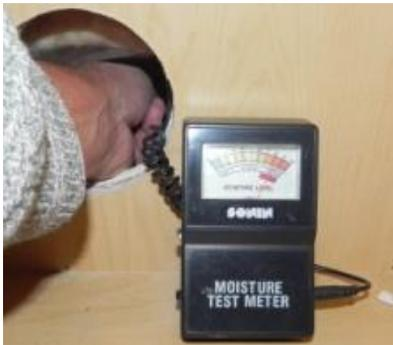
The major contributors to the intolerable condition were the improper installation of the window sill and the window flashing. The window flashing was reverse lapped over the bottom flange of the window. This error allowed water to literally flow behind the water resistant barrier and directly on to the face of the plywood sheathing. This condition allowed rain water to soak the sheathing every time it rained.
