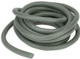
Caulk joints use backer rod to keep the depth of the caulk from exceeding its maximum workable depth into the masonry joint. The sealant does not bond to the backer rod which insures that the sealant adheres to only two sides during the compression and tension of the joint (drawing on the right). Doing so allows the caulk to expand and contract to its maximum ability. The caulk, if adhered on three sides, will not expand properly under tension – it will likely tear.
