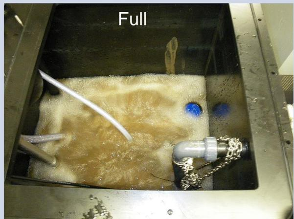
Figure 27: Example of a small industrial submerged membrane bioreactor. The pretreatment & storage tank is on the left and the aerated membrane tank is on the right. Flow is recirculated between these tanks.
