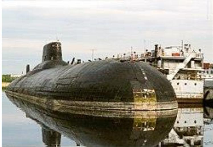
Figure 35: Russian Typhoon Class Ballistic Missile Submarine. Only one of these is still in operation, and a replacement class is now being designed. This has a side-by-side double pressure hull design which makes her very difficult to sink and provides luxurious living space for the crew; it even includes a sauna with sunlamps!
