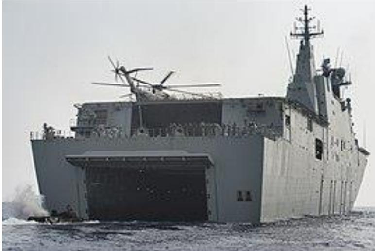
Figure 7: Stern view of Australian amphibious assault ship HMAS Adelaide. Note the large stern door, helicopter hangar, and landing craft entering the well deck,
