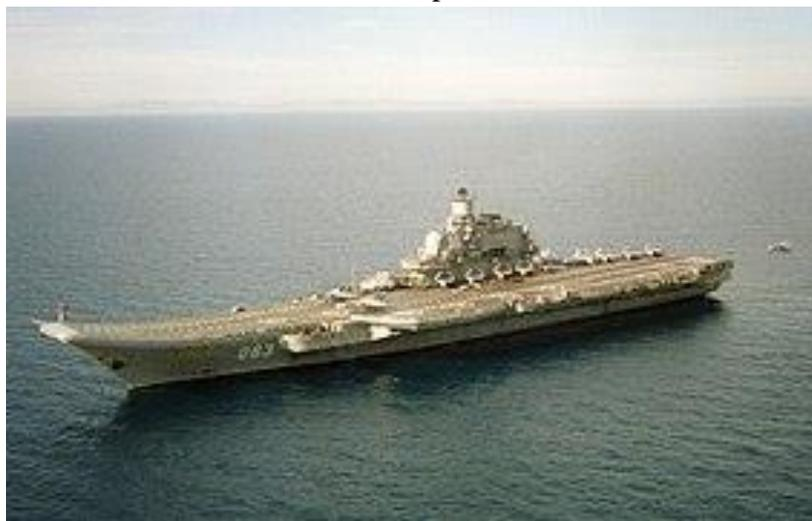
Figure 3: Russian Admiral Kuznetsov with ski-jump bow. This is an old Soviet-era ship that has a poor mechanical reliability record.
