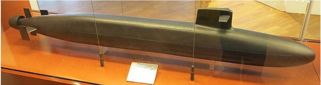
Figure 33: Model of a French Nuclear Ballistic Missile Submarine. Note the nozzle around the propeller.
