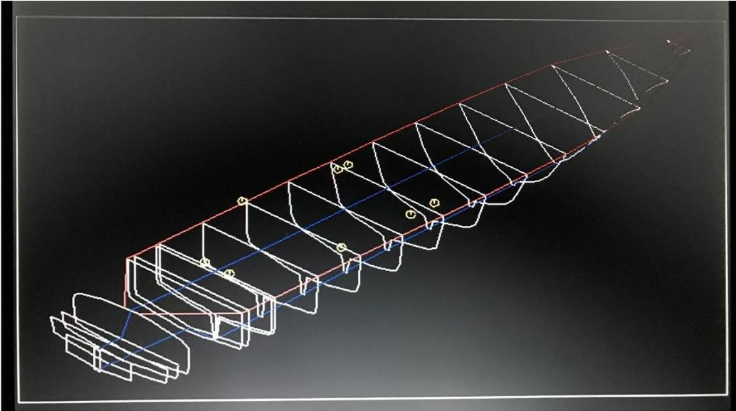
Figure 2: Wireframe hull model of a modern yacht with a swim platform
