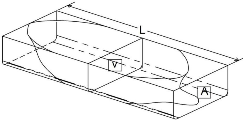
Figure 5: Prismatic Coefficient
