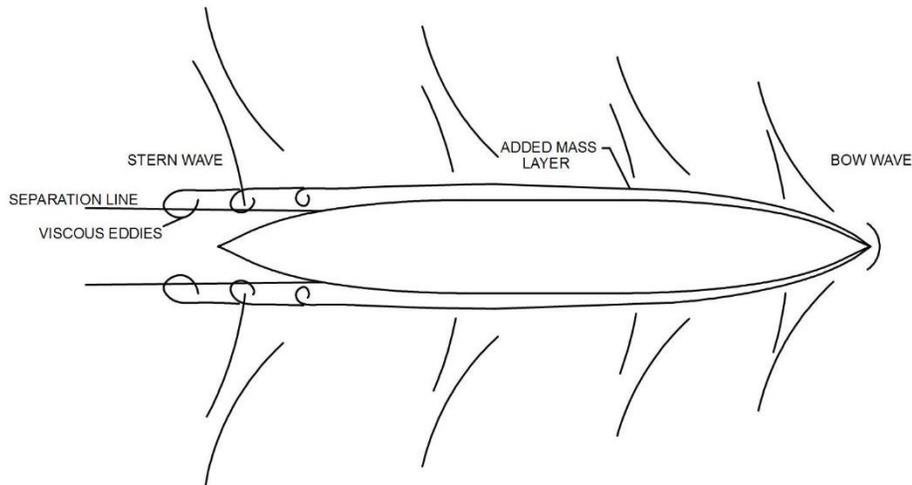
Figure 10: Typical Ship Wake Pattern
