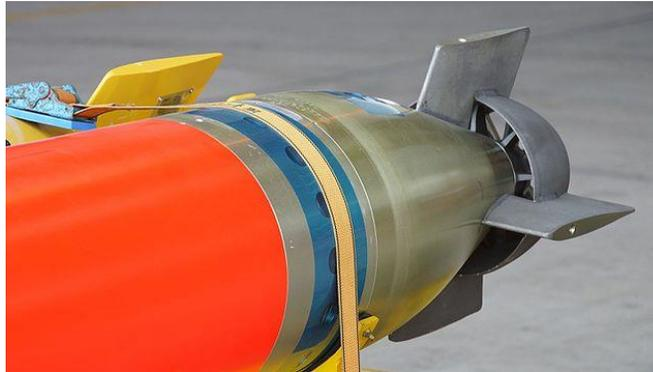
Figure 17: Pumpjet on a torpedo
