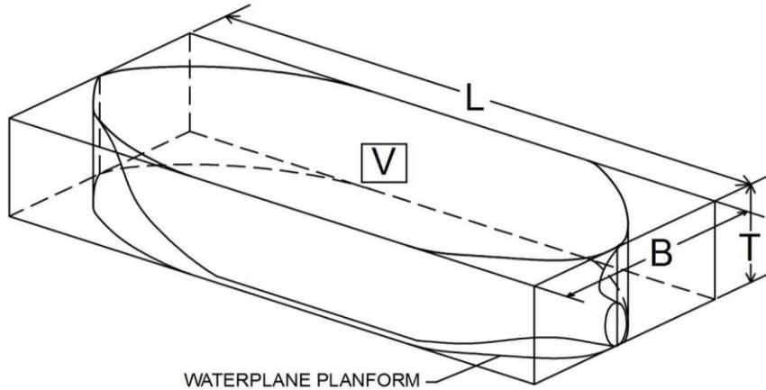
Figure 7: Vertical Prismatic Coefficient
