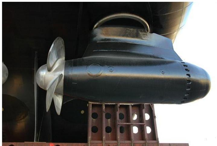
Figure 9: Azipod Thruster
