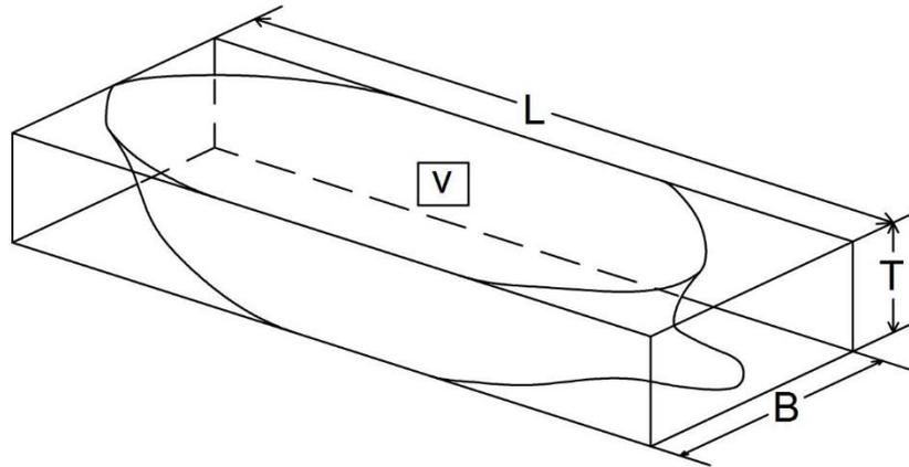
Figure 2: Block Coefficient
