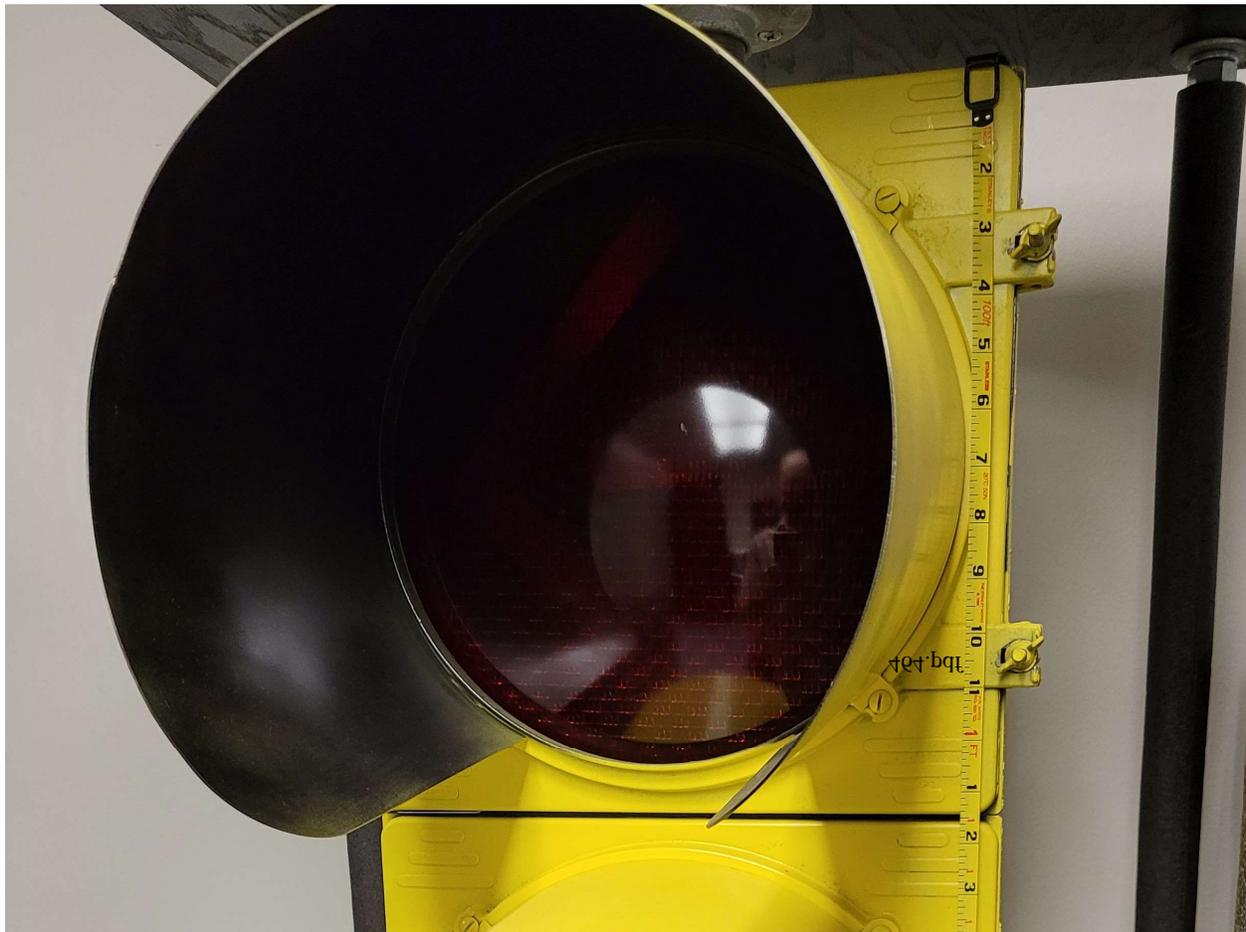
Figure 8. 12-inch lens within 14-inch enclosure
