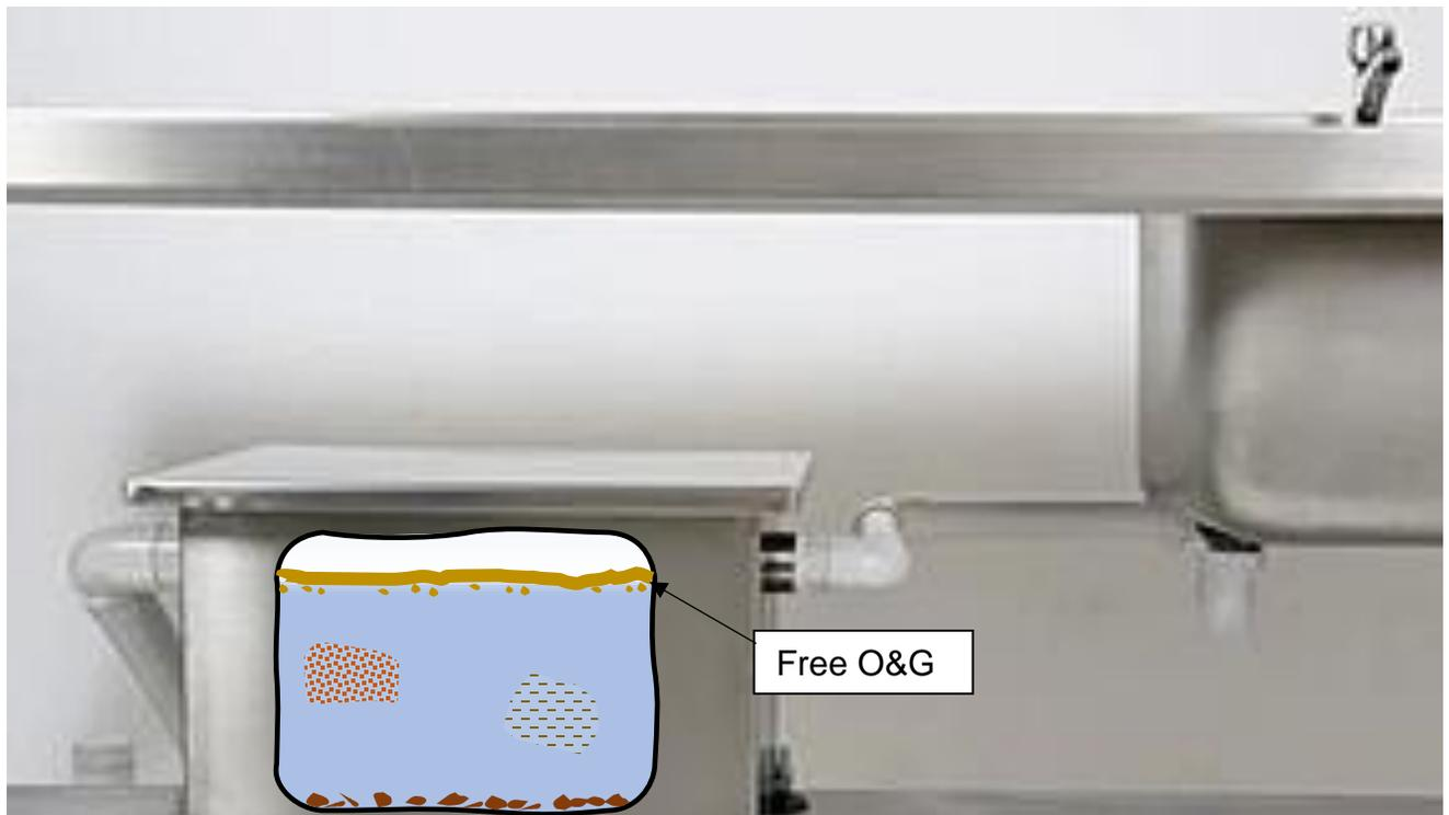
Figure 7: View inside a grease trap with free O&G at the top.
