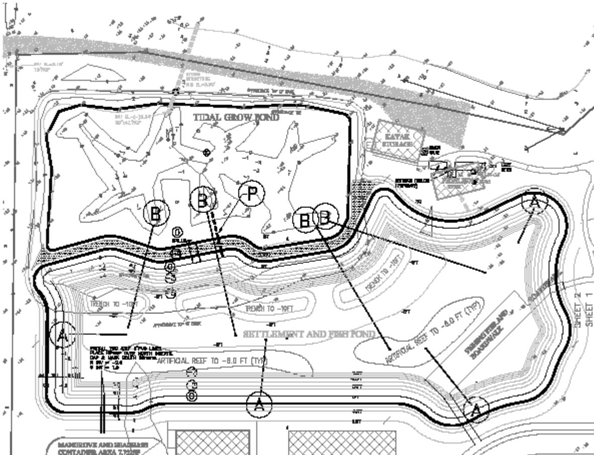
Figure 6 – Tidal Pond Piping – 24” Culvert (P), Bi-directional flow pipes (B), Air Lifts (A)
