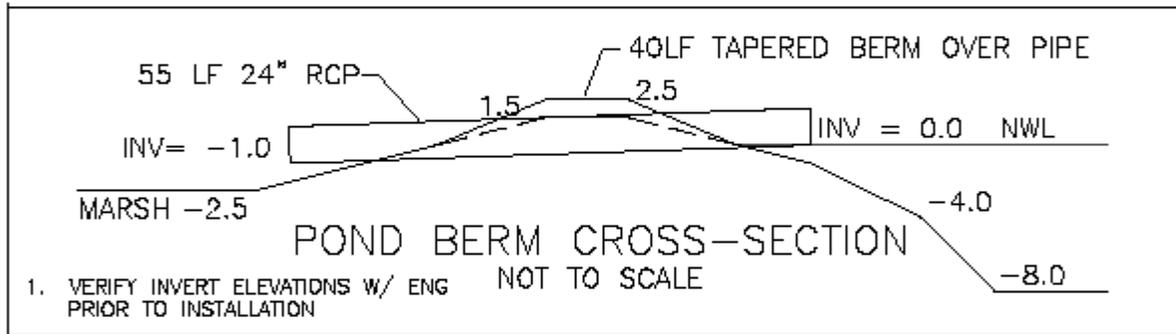
**Figure 7** – Pond cross-section at culvert crossing
