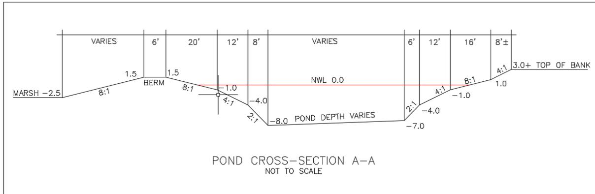
**Figure 14 - Cross-section of Pond Side Slopes**
