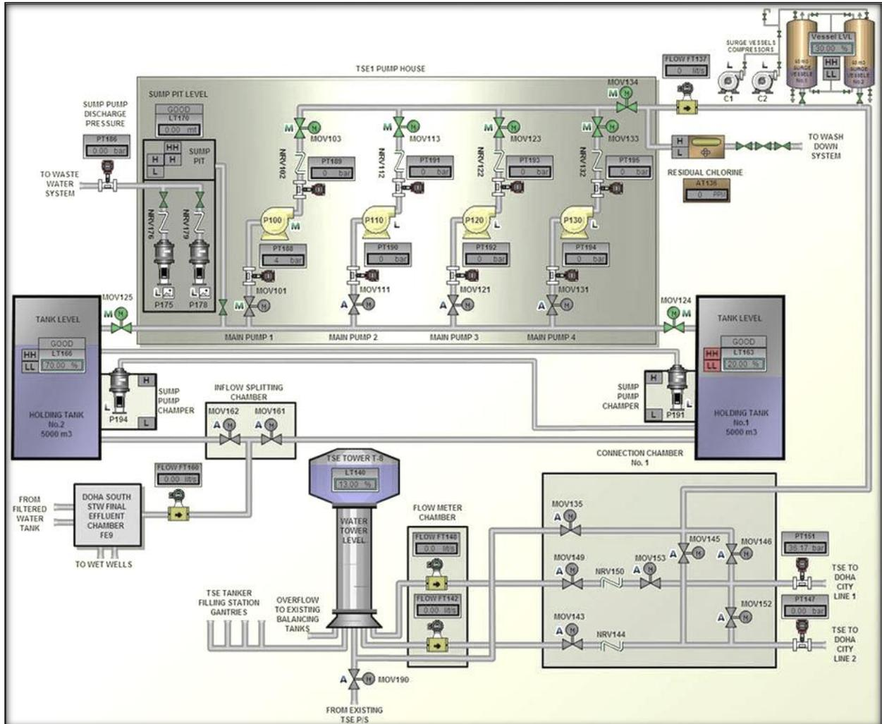
Figure 8: Example SCADA screen showing meter and instrument readings. A historian records these readings on regular intervals. This data helps with performance evaluations and water quality problem troubleshooting.
