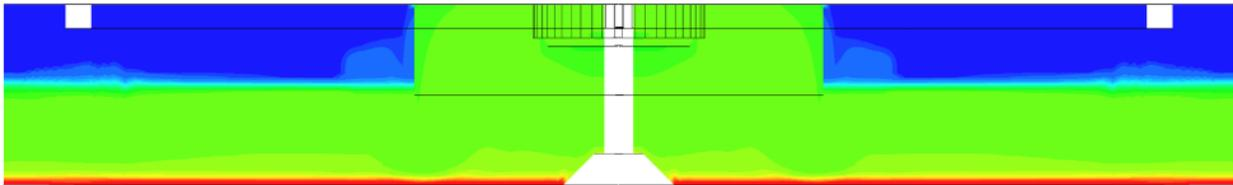
Figure 11: CFD model results for solids concentration of a clarifier.
