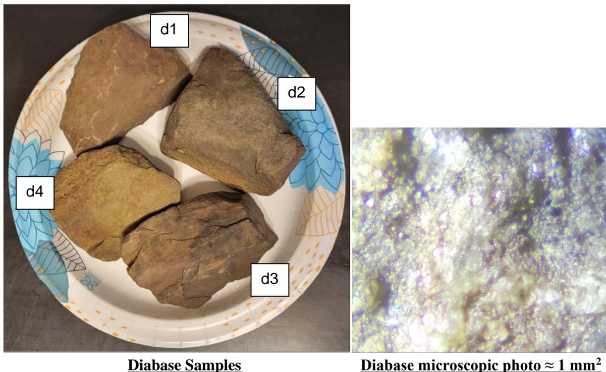
**Figure 2.8: Dike (Diabase) Rock Samples**
