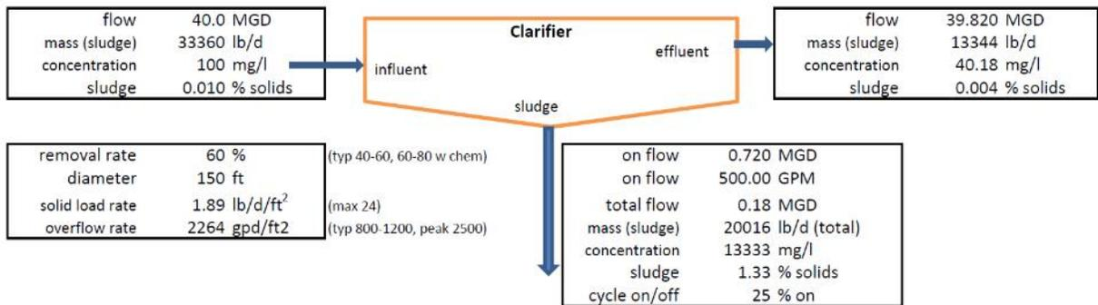
Figure 9: Example mass balance for a clarifier at peak flow. Note the mass of sludge entering the clarifier (33,360 lb/d influent) equals the mass leaving the clarifier (13,344 lb/d effluent plus 20,016 lb/d sludge).
