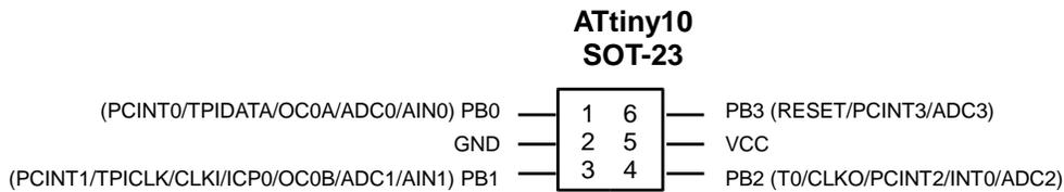
**Figure 2 - ATtiny10 pinout**
