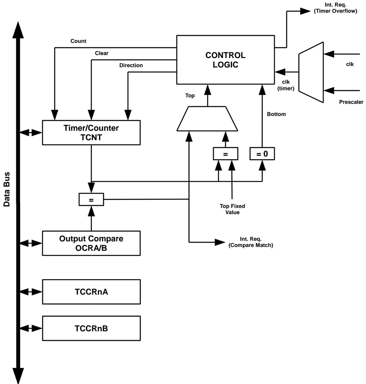
**Figure 6 - Block Diagram of Timer Peripheral**
