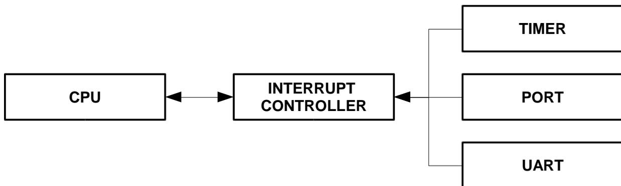
**Figure 5 - Interrupt Controller, Processor and Peripherals**
