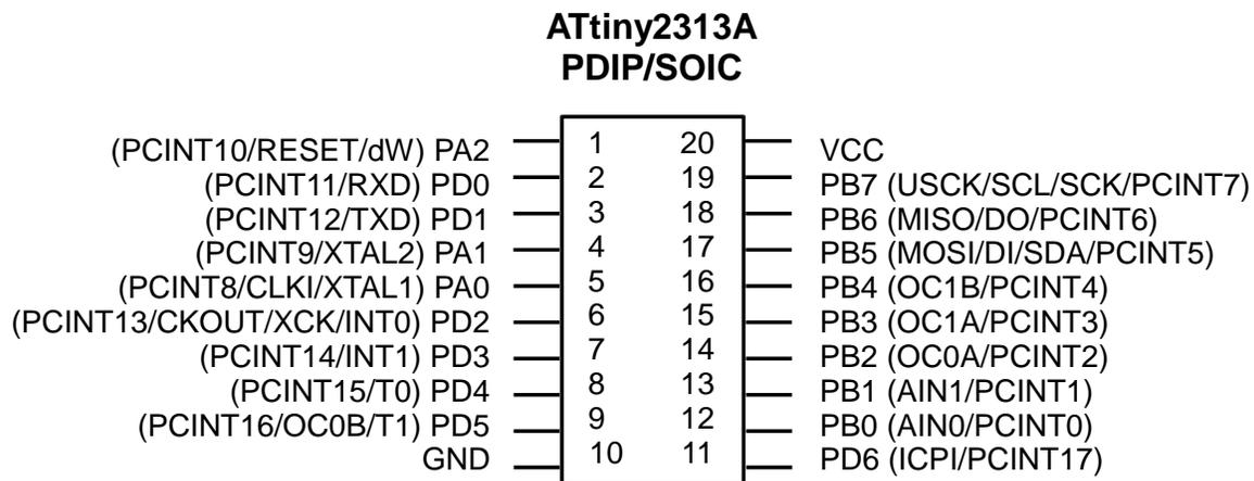
Figure 1 - ATtiny2313A pinout
