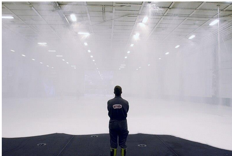
Figure 4: Testing of Aqueous Film Forming Foam (AFFF) sprinklers.
