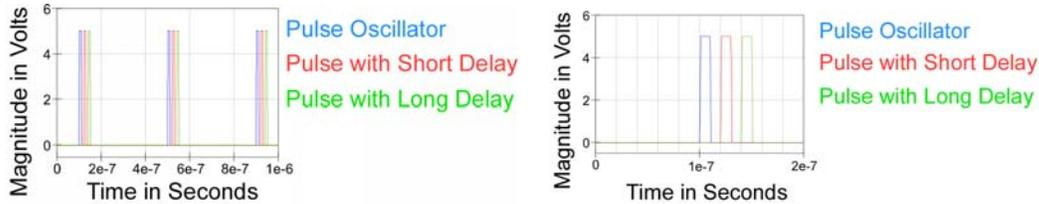
**Figure 16.1 The 2.5MHz Pulse Oscillator with Two Delayed Replicas**
