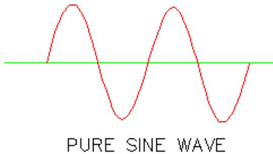
Ideally, we want our inverter to produce power that replicates this wave as close as possible for our use in the structure to avoid problems.
