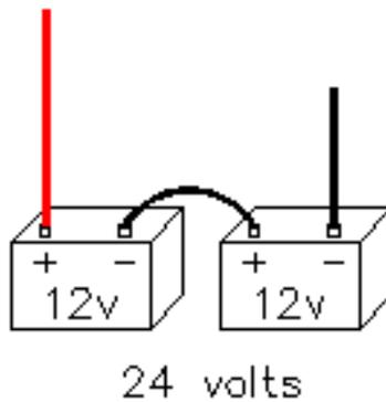
**Remember: Series wiring → Current stays the same and Voltage is additive.**
