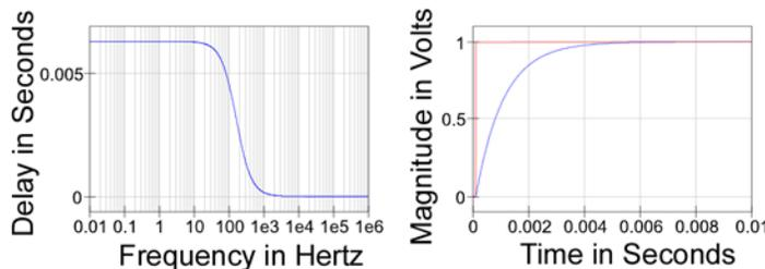
**Figure 5.1 Group Delay of  $H(f)$  System and Step Response**
