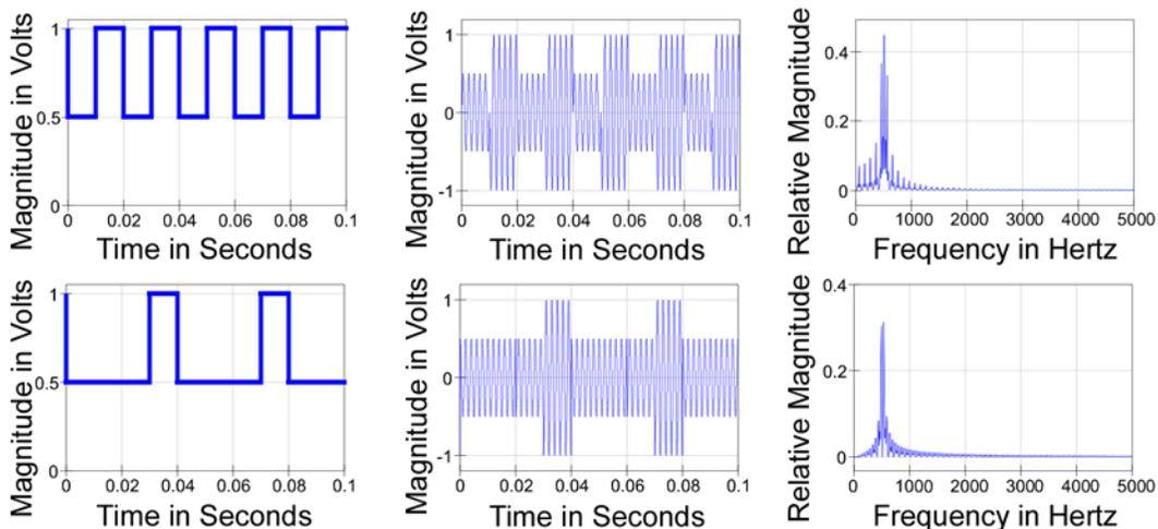
Figure 15.2 The VAI and VAq Sequences, the VChi and VChq Signals, and Spectra
