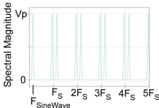
Figure 7.1 Multiple Spectral Lines from the Sampled “Sine Wave” Source
