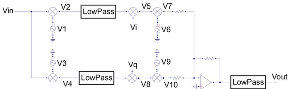
**Figure 13.0 Weaver Architecture with  $V_i$  and  $V_q$  Phase Modulation**
