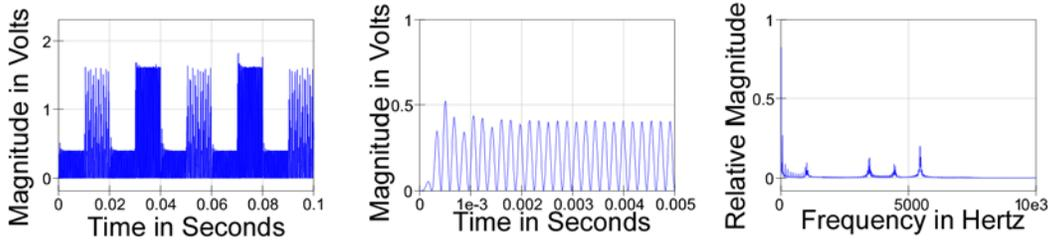
Figure 16.2 *Vout* Squared, a Detail, and the Spectrum
