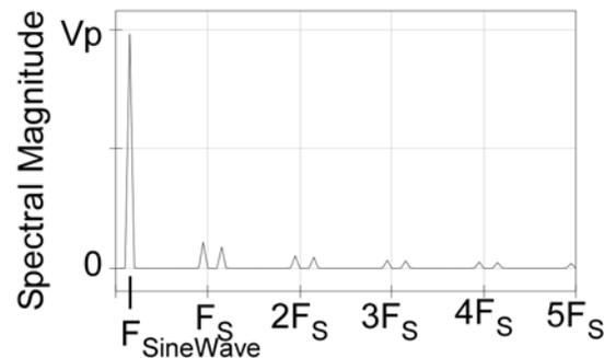
**Figure 9.2 Spectrum of the Sampled “Sine Wave” with a Zero-Order-Hold Filter**
