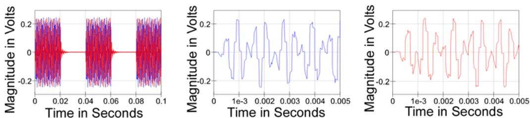
Figure 12.1  $V_7$  &  $V_{10}$  Burst Waveform,  $V_{10}$  Burst Detail, and  $V_7$  Burst Detail
