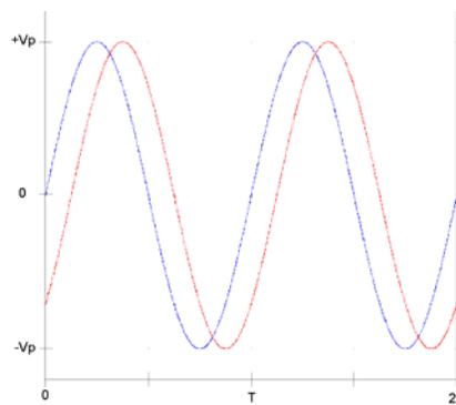
**Figure 3.0 Two Sinusoids with the same Period and a Phase Difference**
