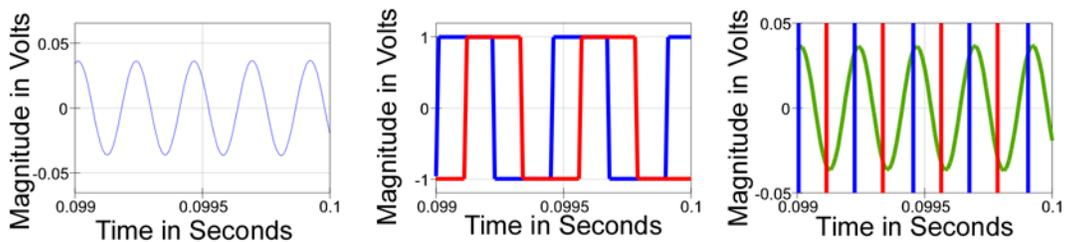
Figure 16.4 Band pass Filtered *Vout* Squared, *VRec\_i* and *VRec\_q*, and the Compare
