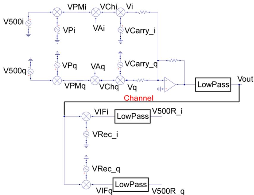
**Figure 15.0 Weaver Modulator Modified to Carry Amplitude and Phase Data**
