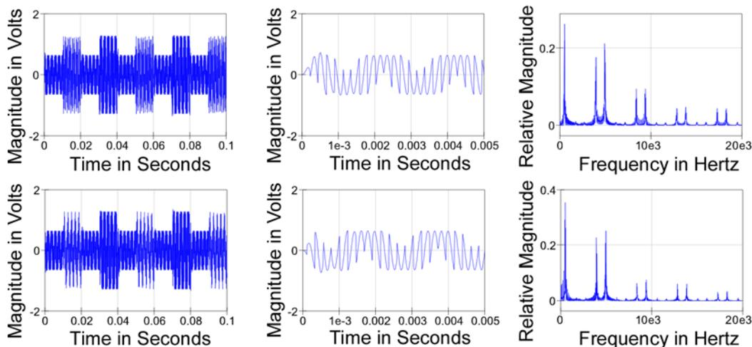
**Figure 16.5 *VIFi* above *VIFq* below, Details, and Spectra**
