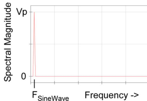
Figure 7.0 Single Spectral Line from the “Sine Wave” Source
