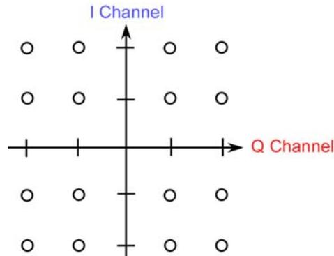
**Figure 15.3 The I Channel and Q Channel Bit Constellation**
