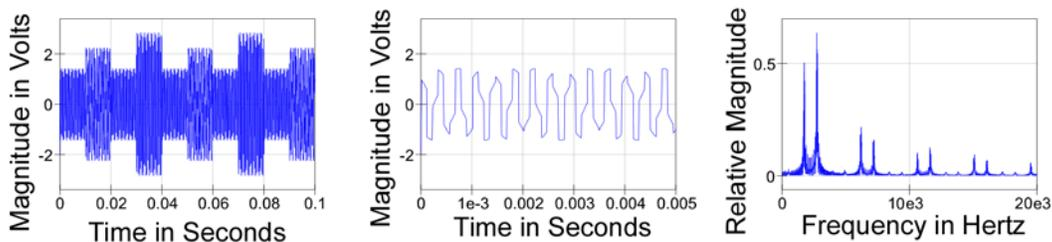
**Figure 15.4 The Sum of  $V_i$  and  $V_q$  Signals, The Sum Signal Details, and Spectrum**
