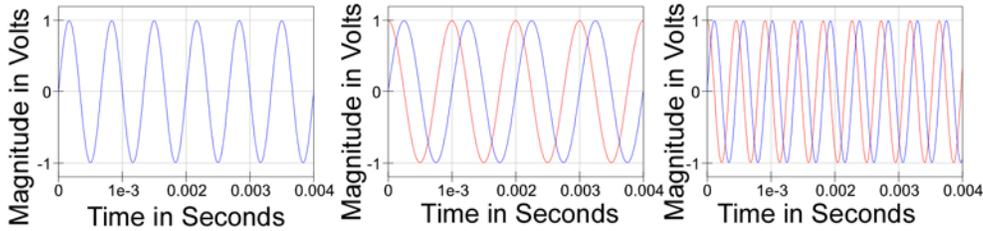
**Figure 11.1  $V_0$  at 1500 Hz,  $V_1$  &  $V_3$  at 1000 Hz, and  $V_6$  &  $V_9$  at 2200 Hz**
