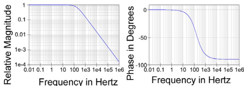
**Figure 5.0 Bode Plot of a Single-Pole Low Pass  $H(f)$  System Response**
