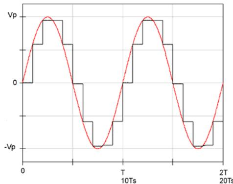
**Figure 9.0 Sampled “Sine Wave” with a Zero-Order-Hold Filter Waveform**
