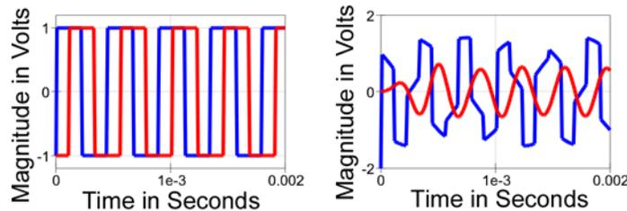
**Figure 16.1  $V_{Carry\_i}$  and  $V_{Carry\_q}$  Square Waves, Filtered and Un-Filtered  $V_{out}$**
