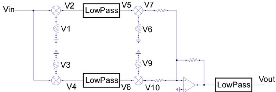
Figure 12.3 Weaver Architecture with Harmonic Suppression Low Pass Filter
