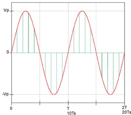
**Figure 6.2 Example “Sine Wave” and Sampled Output**
