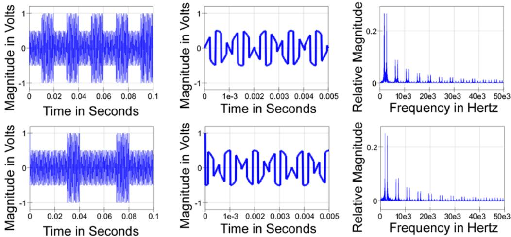
**Figure 15.3 The  $V_i$  and  $V_q$  Signals,  $V_i$  and  $V_q$  Signal Details, and  $V_i$  and  $V_q$  Spectra**
