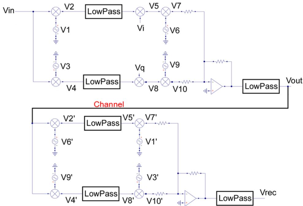
**Figure 14.0 Communicating Interconnection of Weaver Modulators**
