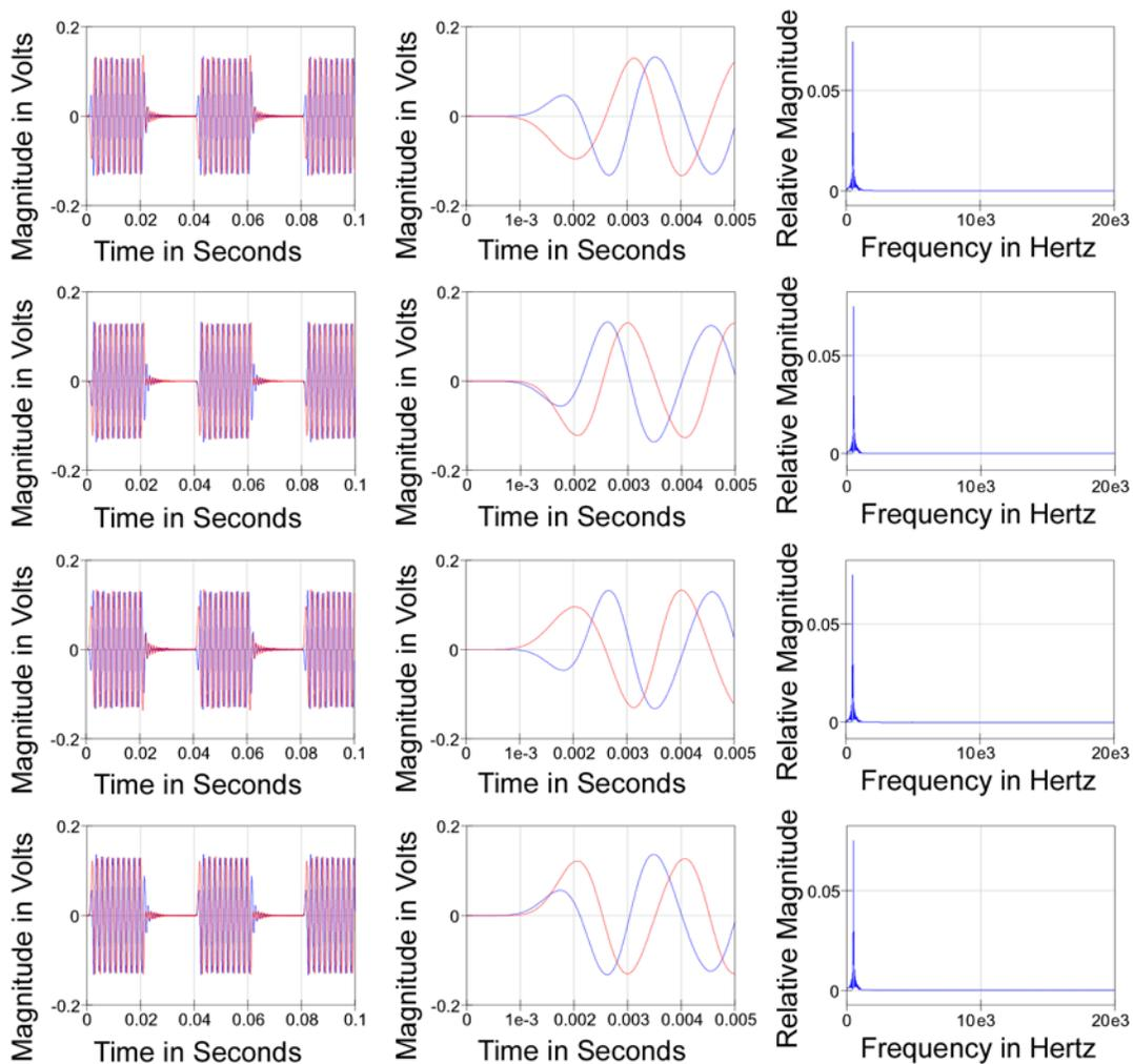
Figure 14.2  *$V_2$  &  $V_4$  Burst.  $V_2$  &  $V_4$  Burst Detail, and  $V_2$  &  $V_4$  Spectra Detail*
