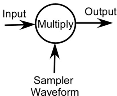
**Figure 6.0 Sampling a Continuous-Time Signal**
