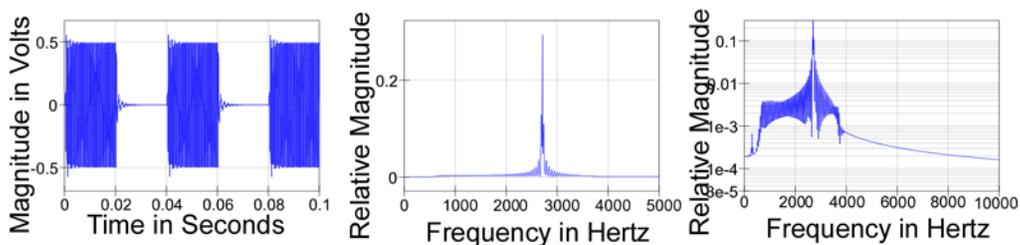
Figure 11.7  $V_{out}$  Burst.  $V_{out}$  Spectra, and  $V_{out}$  Spectra Logarithmic
