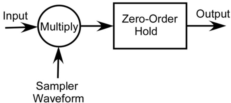
**Figure 9.1 Sampler with Zero-Order-Hold Filter System**
