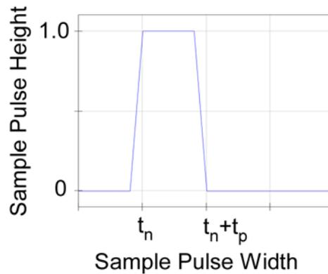
**Figure 6.3 A Single Pulse from the Periodic Sampling Waveform**
