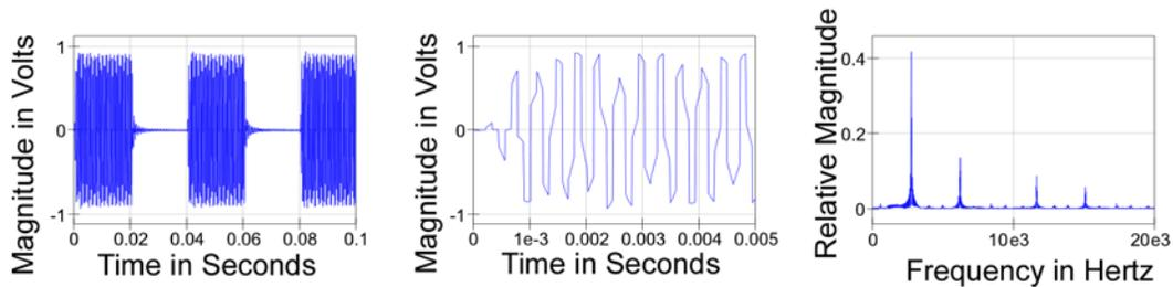
Figure 12.7  $V_{out}$  Burst.  $V_{out}$  Burst Detail, and  $V_{out}$  Spectra
