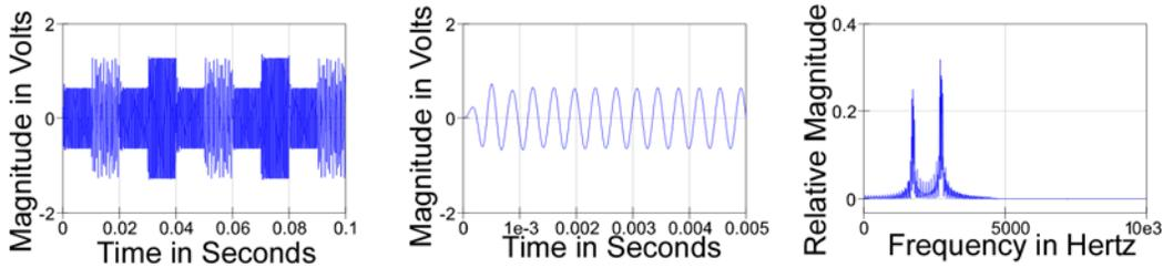
**Figure 15.5 The  $V_{out}$  Filtered Signal, The Signal Detail, and its Spectrum**
