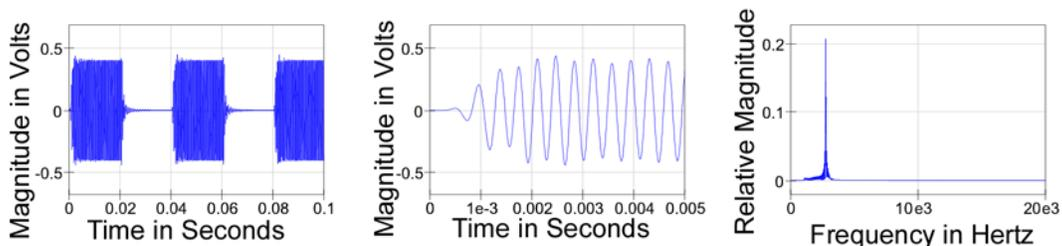
Figure 12.4 Filtered  $V_{out}$  Burst. Filtered  $V_{out}$  Burst Detail, and Filtered  $V_{out}$  Spectra
