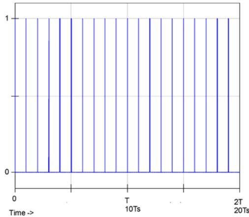
**Figure 6.1 Unit Magnitude Periodic Sampling Waveform**
