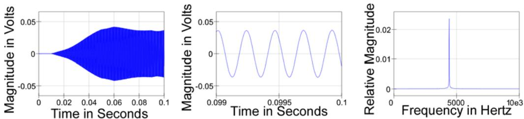
Figure 16.3 Band pass Filtered *Vout* Squared, a Detail, and the Spectrum
