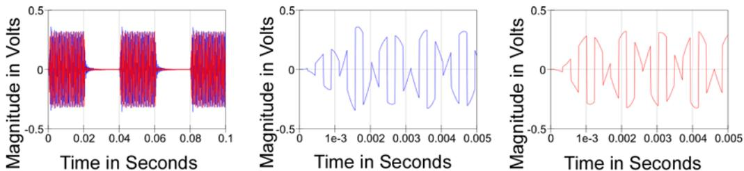
**Figure 12.6  $V_7$  &  $V_{10}$  Burst Waveform,  $V_{10}$  Burst Detail, and  $V_7$  Burst Detail**
