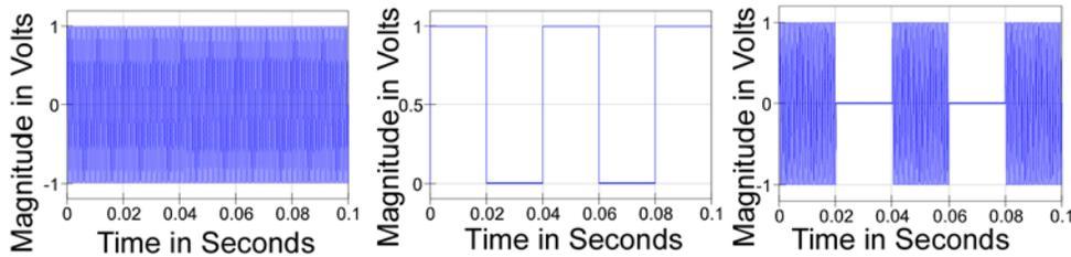
**Figure 11.2  $V_0$  at 1500 Hz, 25 Hz Square Modulation, and  $V_{in}$  Tone Burst**
