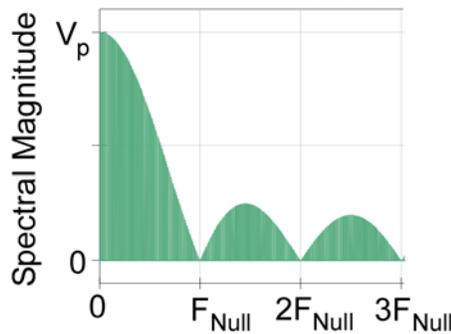
**Figure 7.2 Broad Spectral Lines from the Sampled “Sine Wave” Spectrum**
