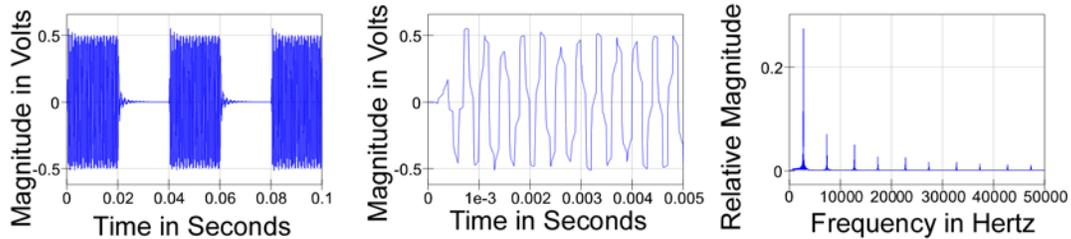
Figure 12.2  $V_{out}$  Burst.  $V_{out}$  Burst Detail, and  $V_{out}$  Spectra
