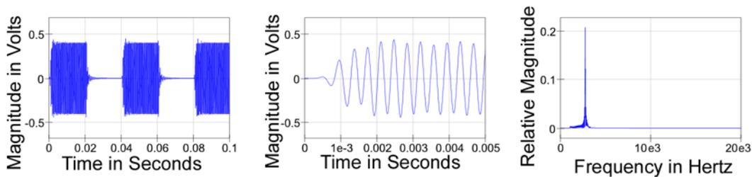
Figure 12.8 Filtered  $V_{out}$  Burst. Filtered  $V_{out}$  Burst Detail, and Filtered  $V_{out}$  Spectra
