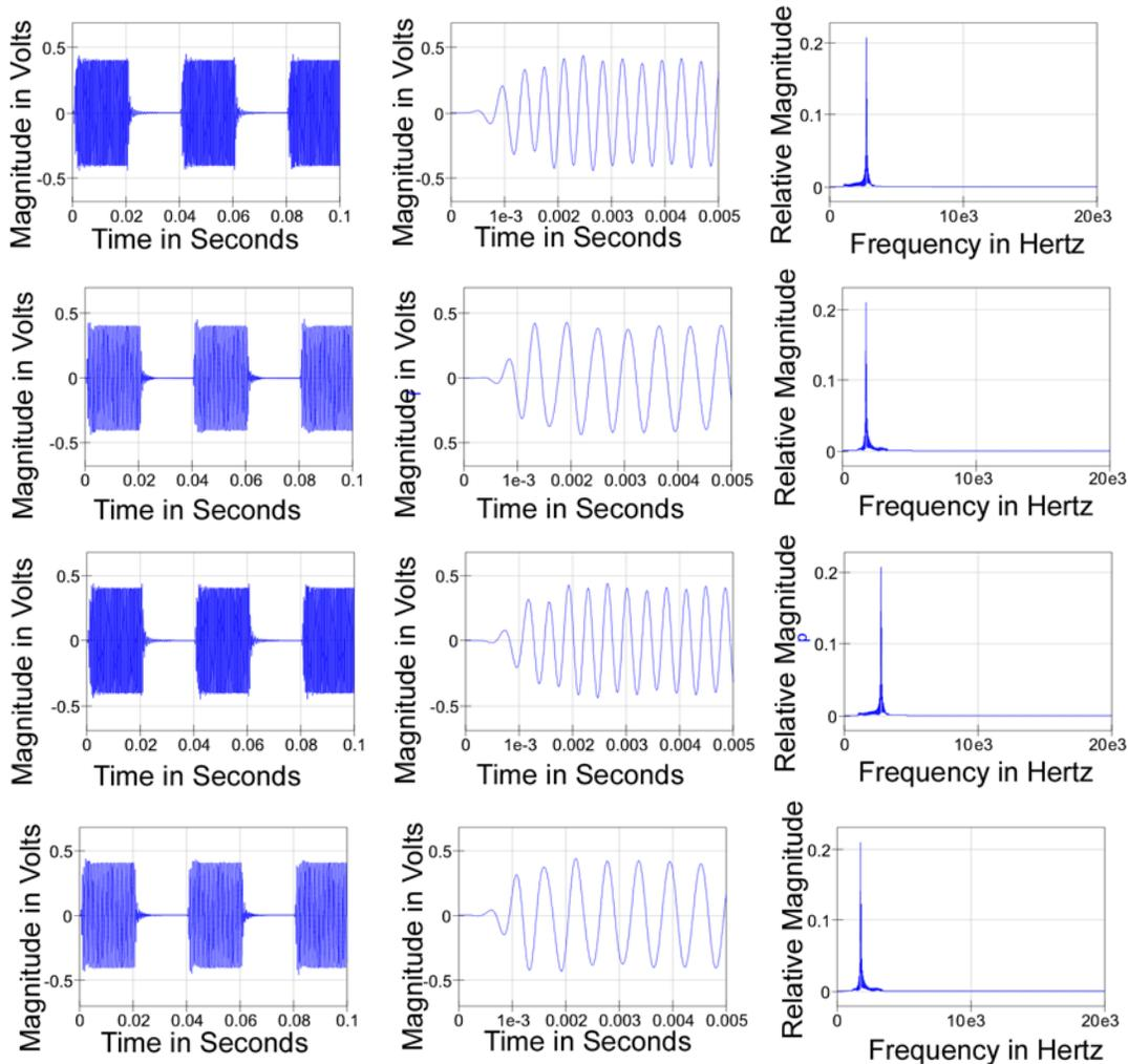
**Figure 13.3 Filtered  $V_{out}$  Burst. Filtered  $V_{out}$  Burst Detail, and Filtered  $V_{out}$  Spectra**
