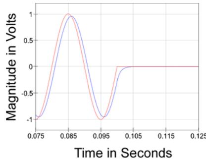
**Figure 5.2 Tone Burst Response of  $H(f)$  System**
