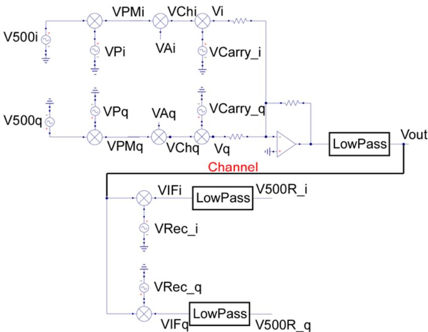
**Figure 16.0 Weaver Modulator Modified to Receive Amplitude and Phase Data**
