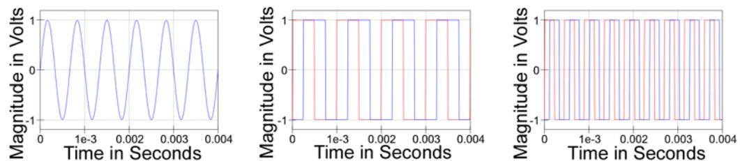
Figure 12.9  $V_0$  at 1500 Hz, Square  $V_1$  &  $V_3$  1000 Hz, and Square  $V_6$  &  $V_9$  at 2200 Hz
