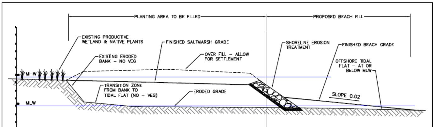
Figure 18: Cross section of the course example wetland restoration project using a rock revetment as a protection system in the “coastal bank” area of highest erosion and wave energy dissipation.
