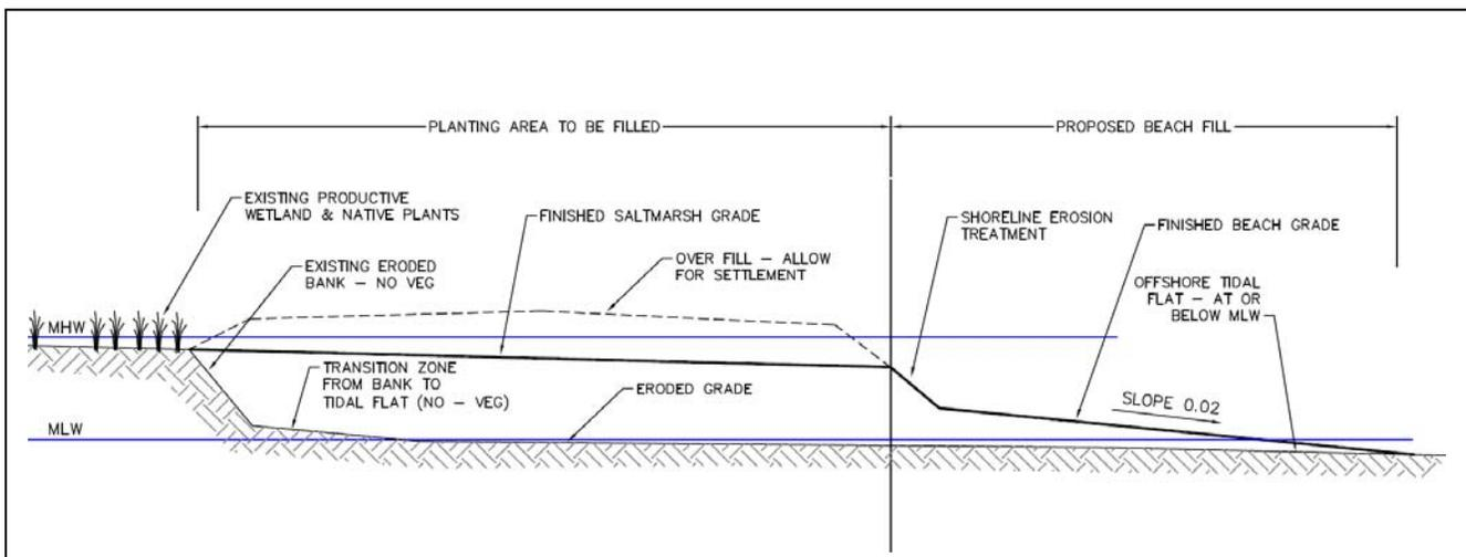
Figure 15: Conceptual profile of existing & proposed wetland restoration fill.
