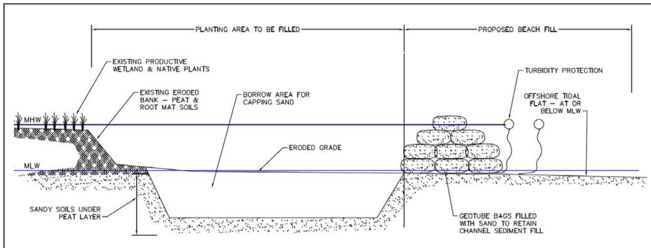
Figure 16: The same proposed wetland habitat shown in Figure 15 with the finished wetland & beach construction removed. The limits of the proposed restored wetland and beach are shown at the top of the figure for reference. The eroded marsh is primarily peat and root mat, but is underlain with sandy soils.
