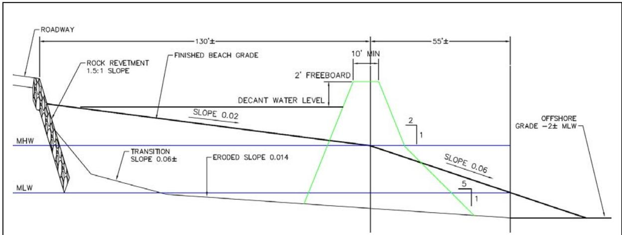
Figure 7: The outboard dike is shown in green, note 2:1 slope on the outboard side above high water line, and 5:1 slope in the intertidal zone. Placement of the dike should be reasonably close to the outside limit of the beach fill area.
