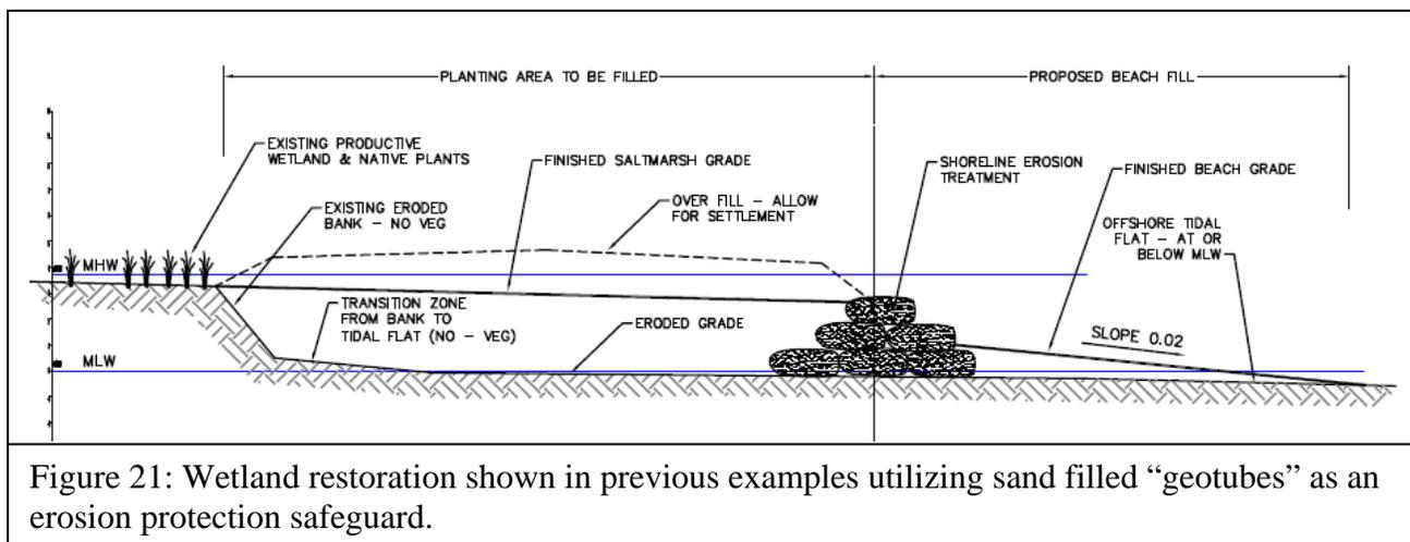
Figure 21: Wetland restoration shown in previous examples utilizing sand filled “geotubes” as an erosion protection safeguard.
