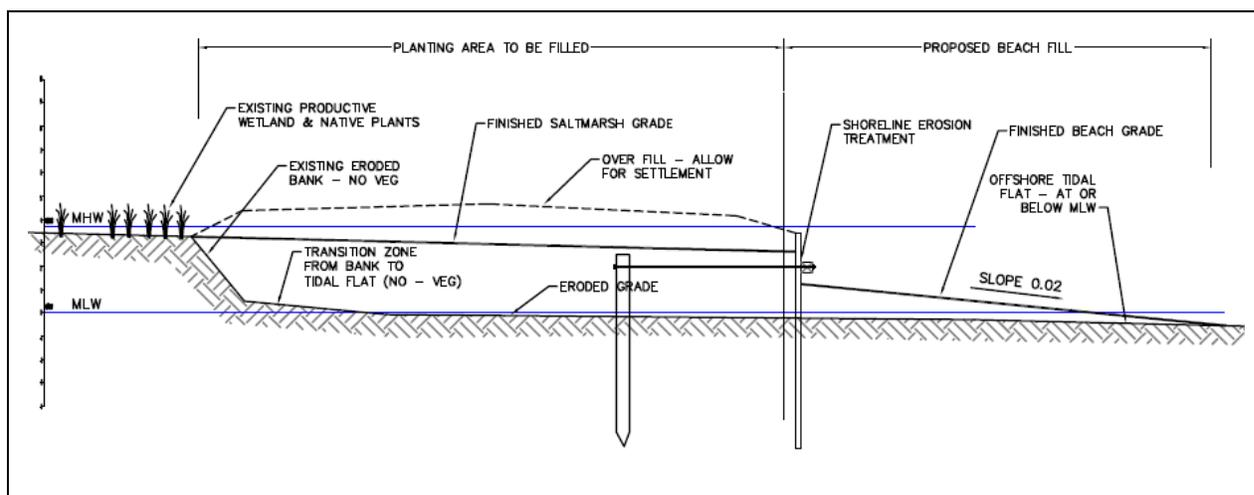
Figure 20: Wetland restoration shown in previous examples utilizing a wood bulkhead as an erosion protection safeguard.
