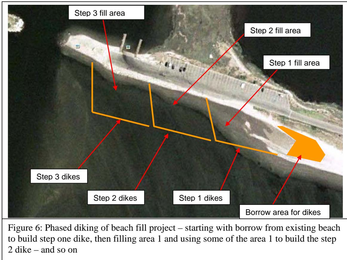
Figure 6: Phased diking of beach fill project – starting with borrow from existing beach to build step one dike, then filling area 1 and using some of the area 1 to build the step 2 dike – and so on
