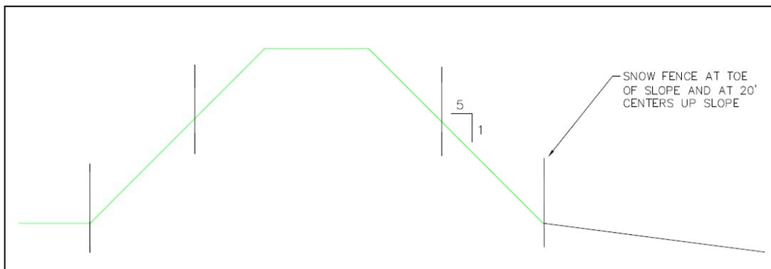
Figure 9: Basic dune cross section, with 5:1 slope shown. Also snow fence at toe and up slope at 20 to 30 foot centers
