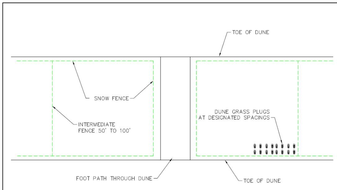
Figure 10: simple dune layout, with cross path, snow fence lines and planting.
