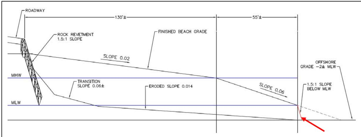
Figure 8: The completed fill template, showing the offshore areas that usually need to be manually graded to meet the uniform offshore grade.
