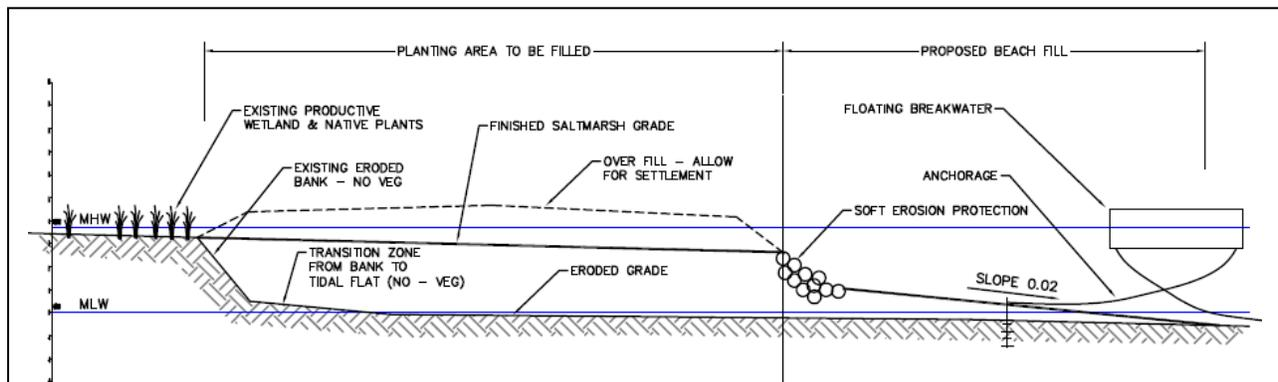
Figure 21: Wetland restoration shown in previous examples utilizing an offshore floating breakwater as an erosion protection safeguard. Also note the used of a “soft” shoreline protection system at the new “coastal bank”.
