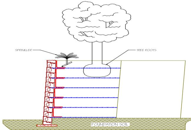
Landscaping above the geosynthetic-reinforced zone should be controlled. The wall designer should be consulted before excavating through layers of reinforcement for the planting of trees and shrubs. As a minimum, small shrubs should be located 5-feet from the MSE facing system and trees located 10-feet from the MSE facing system.
