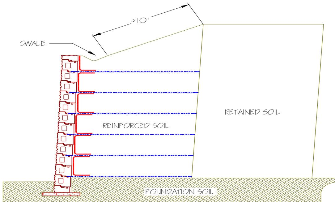
If a backfill or crest slope is to be graded at the top of a MSE wall or slope and the backfill or crest slope length exceeds 10-feet, then a drainage swale must be constructed behind the wall crest. To provide room for the swale, the wall height must be increased accordingly based on the swale width and depth as determined by the civil engineers hydraulic study. The grading and drainage plan must also reflect the presence of a swale.
