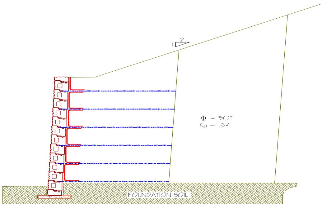
If a mechanically stabilized earth (MSE) wall or slope is to be constructed, it is preferred to locate the wall or slope on top of the toe slope. This type of geometry results in significantly less stress, both internally and externally, on the geosynthetic-reinforcement and the MSE facing system. As shown in the example above assuming a friction angle of 30-degrees.
