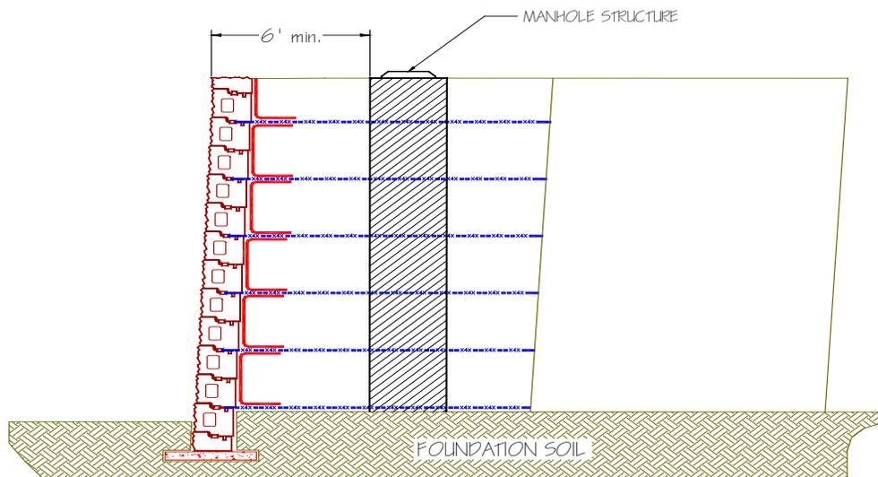
If a vertical storm water riser is placed within the geosynthetic-reinforced zone, it should be located such that there remain at least 6.0-feet between the edge of the riser and the back of the MSE facing system. This amount of space allows for proper compaction of soil. However, it is strongly recommended that all utilities, i.e., storm pipes, electrical, gas, catch basins, drop inlets, etcetera be located outside the geosynthetic-reinforced zone.
