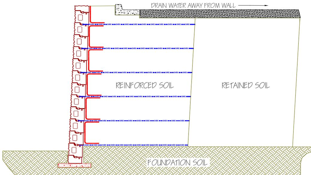
Where parking lots or roadways are constructed behind the crest of a MSE wall or slope, it is important to make sure surface water or sheet flow is directed away from the wall and collected in drop inlets located outside of the geosynthetic-reinforcement zone.
