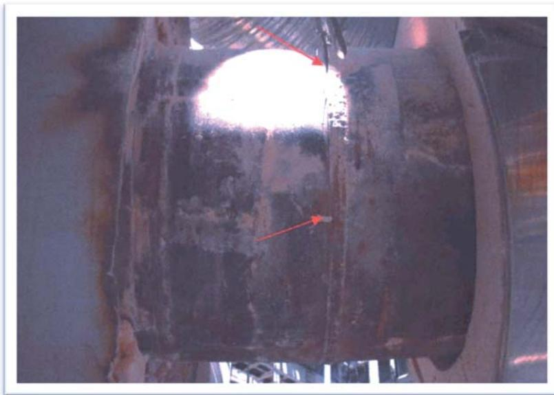
This through wall failure of a high temperature steam line luckily did not cause any injuries, but it took several hundred MWe off the power grid during the hottest part of the summer. A strong contributing cause of the failure was malfunctioning pipe supports.
