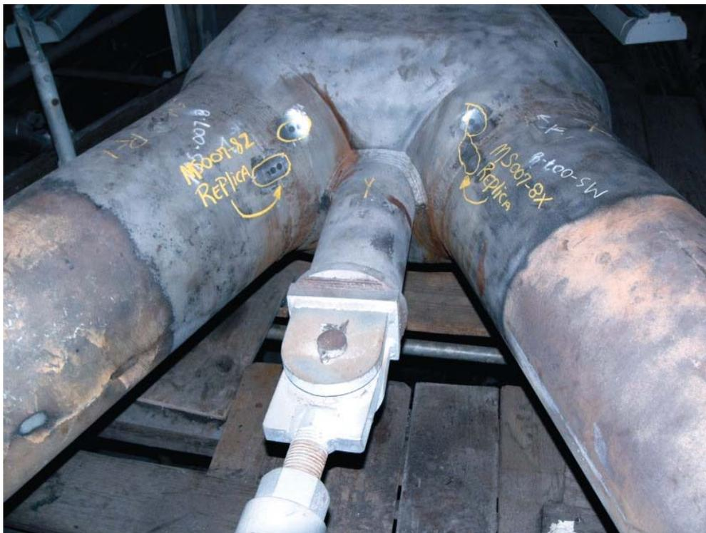
General Photo that shows the orientation, some of the weld numbers, and even the exact replica locations. With this general view and the weld numbers readable on the photos, there will be clear identification to any future observers of the orientation and location of the welds.
