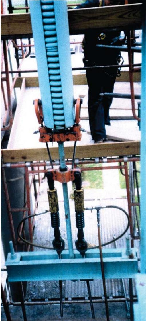
An example of a test set-up to measure the load on a variable spring hanger: The orange yokes and yellow hydraulic cylinders are arranged to unload the rod below the spring as the hydraulic cylinders are shortened, the load is transferred from the rod into the hydraulic cylinders. When the rod is unloaded, the force in the hydraulic cylinders times the area of the cylinders equals the load that the spring is carrying.
