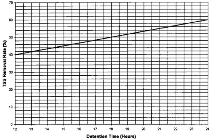
This TSS removal rate is not as high as many other stormwater control practices, such as infiltration basins, sand filters, constructed wetlands, bioretention systems, and others. Therefore, it is often necessary to provide some form of pretreatment upstream of the extended detention basin in order to achieve the desired TSS removal rate.
