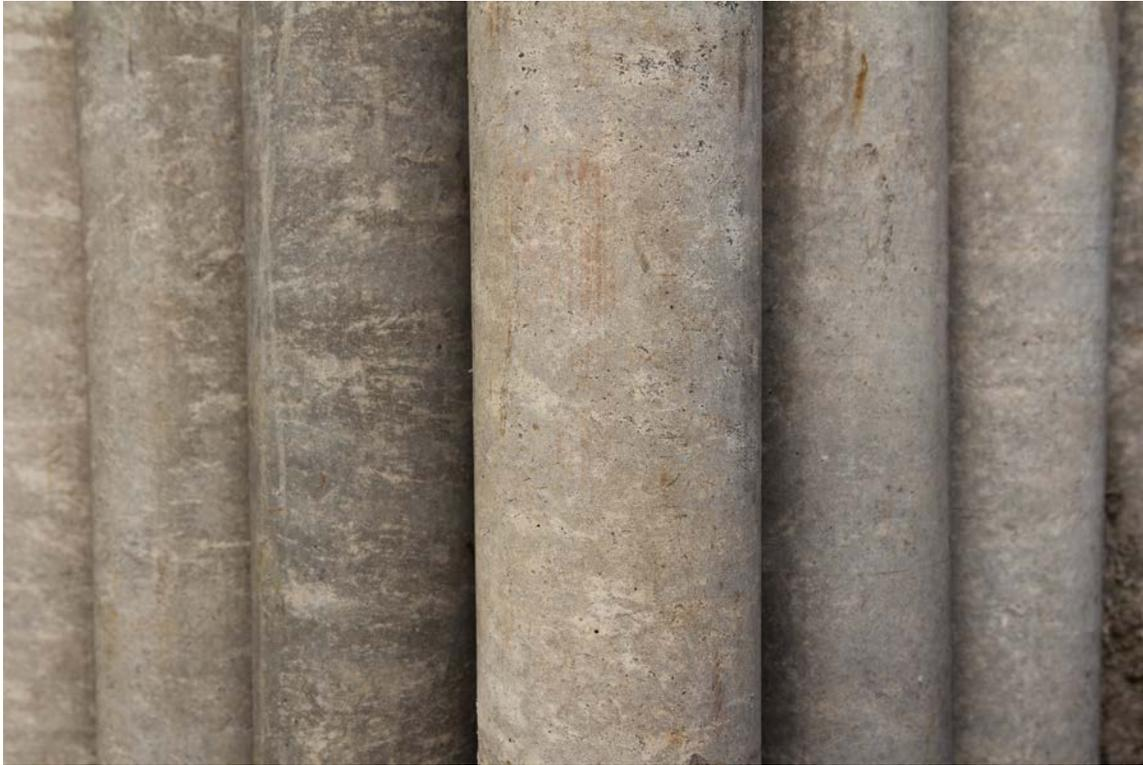
Picture No. 11 by [www.canstockphoto.com](http://www.canstockphoto.com) Asbestos Cement Pipes (ACP) or Transite Pipes
