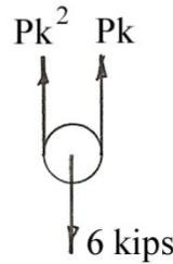
$$\begin{aligned} P(k + k^2) &= 6 \text{ kips} \\ P &= \frac{6}{k + k^2} \\ P &= \frac{6}{.96 + .96^2} \\ P &= 3.19 \text{ kips} \end{aligned}$$
