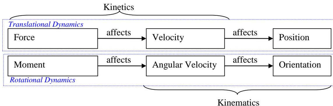
**Figure 1.6: Kinetics vs. Kinematics**
