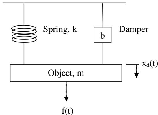
**Figure 3.3: The Mass-Spring-Damper**
