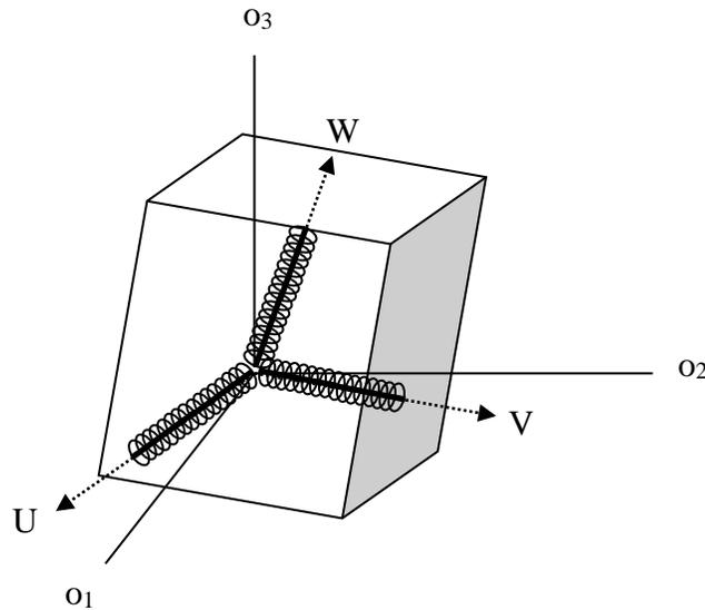
**Figure 3.13: Magnetic – Torque Rod Configuration**
