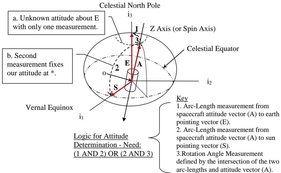
Figure 2.9: Single-Axis Attitude Measurements
