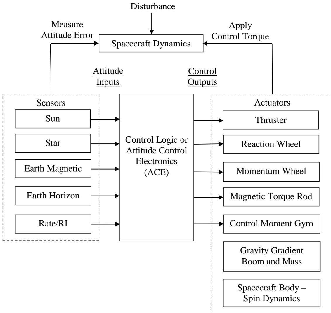
**Figure 3.2: Attitude Control Subsystem (ACS) Functional Diagram**
