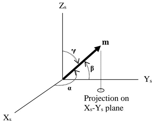
**Figure 2.5: Sensor Coordinate System – Earth Magnetic**
