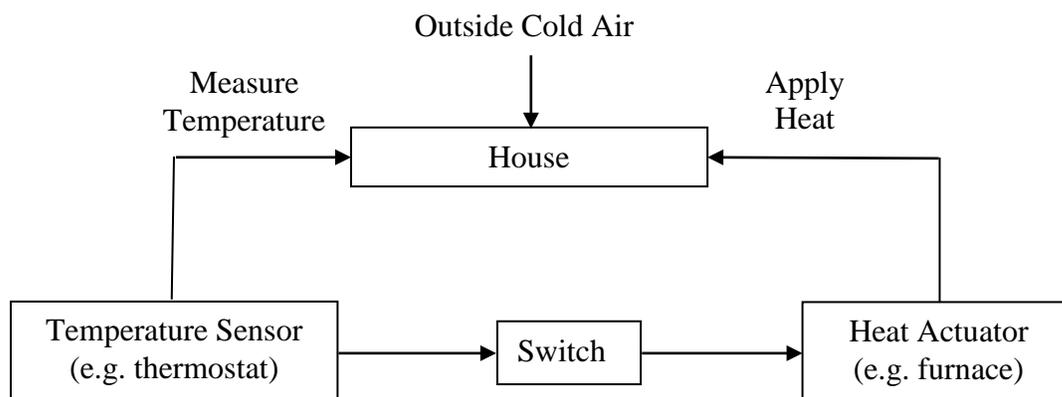
Figure 3.1: Home Heating Control System Functional Diagram
