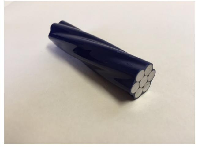
Strand may be coated or uncoated with a smooth or abrasive PVC sheath for added corrosion protection and increase bonding for grout.
