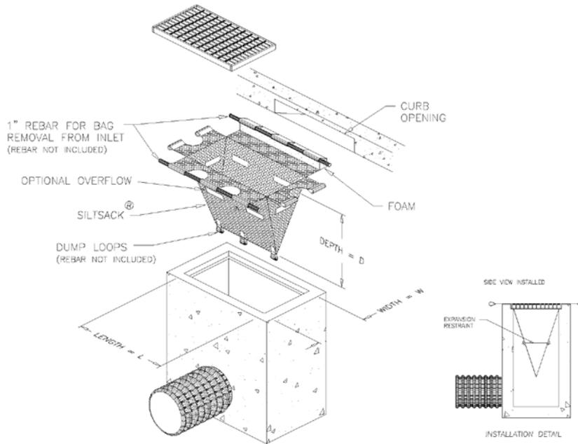
DETAIL OF INLET SEDIMENT CONTROL DEVICE
