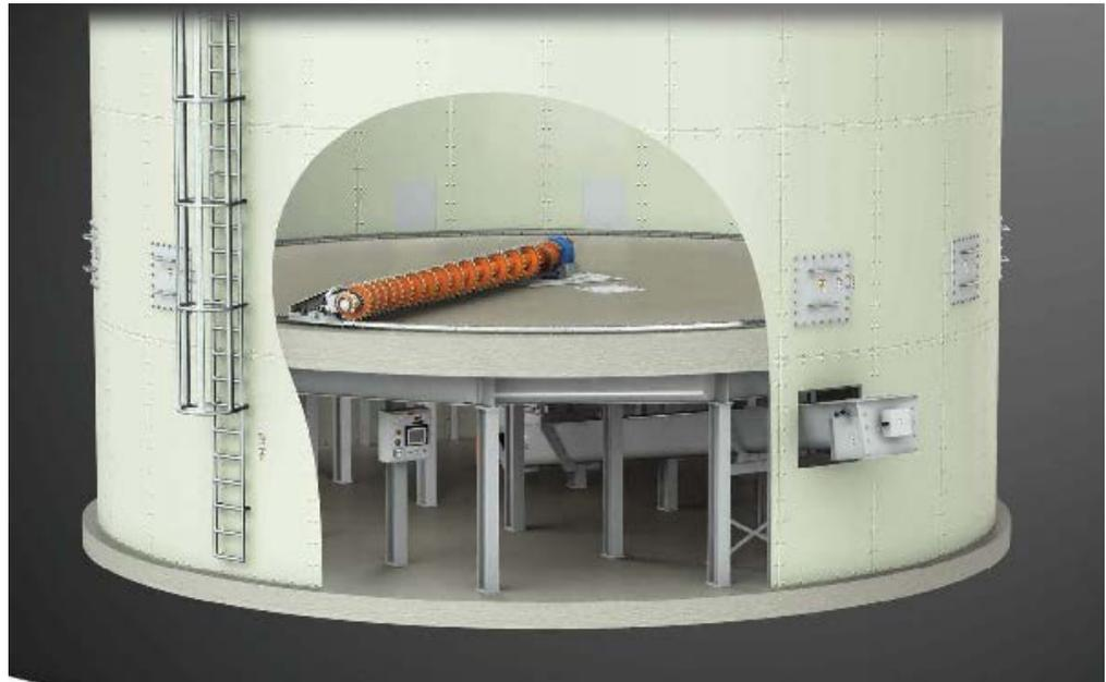
Figure 2. Screw Reclaimer. Note that flights are closer together near the wall and open up toward the center. This ensures that material is drawn from the entire radius of the silo. Also note the metering screw below the silo floor is inclined upward, providing clearance for a receiving conveyor. This is a flat-bottom silo with perimeter-driven screw.
