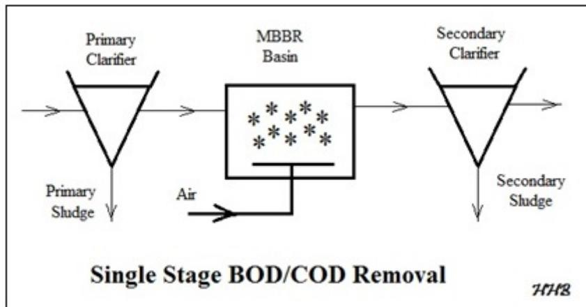
**Figure 5.** Single Stage MBBR Process for BOD/COD Removal
