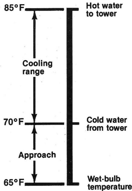
Figure 3: Cooling Tower Range and Approach
