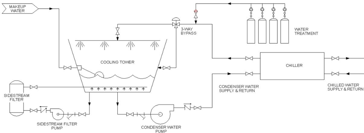
Figure 17: Cooling Tower with Sidestream Filtration and Water Treatment
