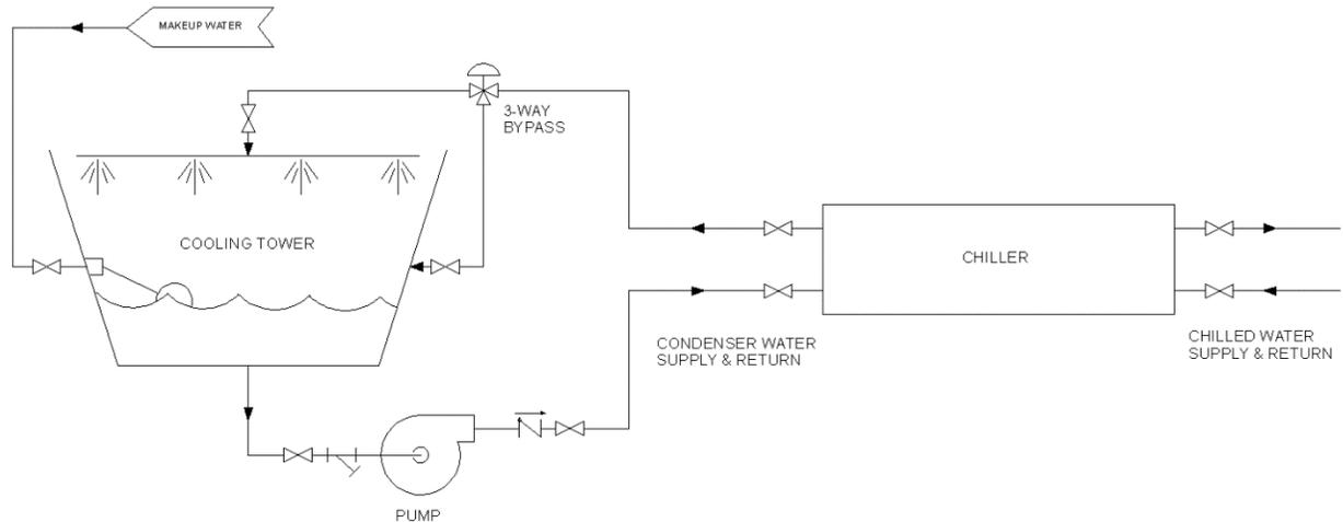
Figure 11: HVAC Cooling Tower Application: Water-Cooled Chiller
