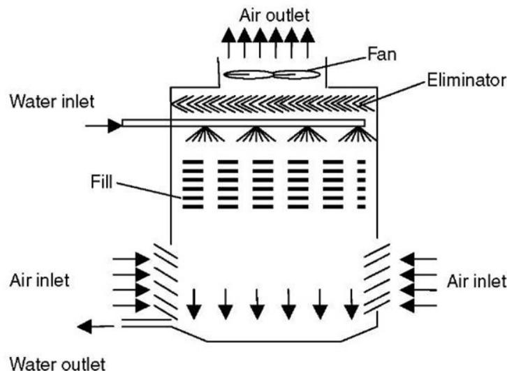
Figure 4: Direct Cooling Tower Diagram
