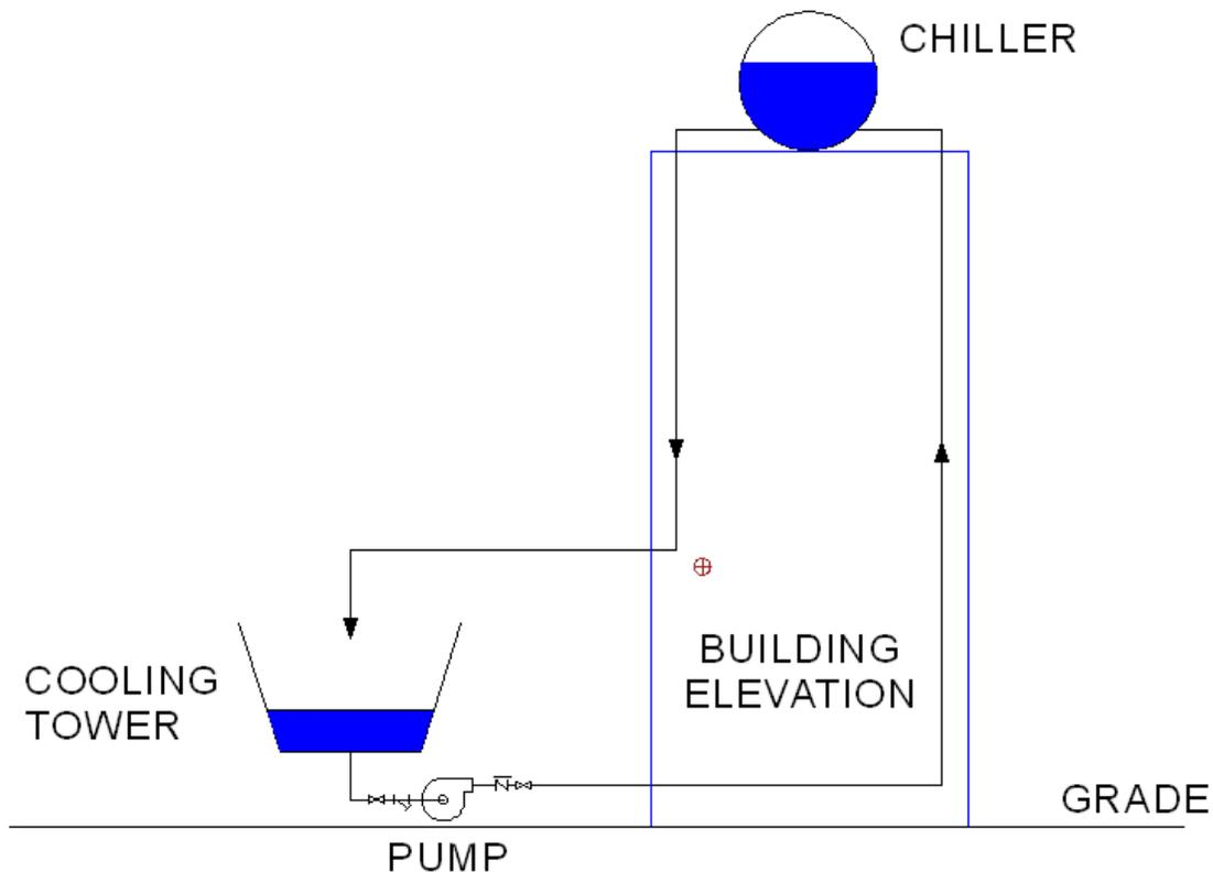
Figure 14: Condenser Water System
