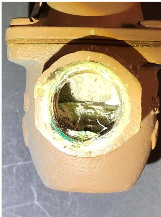
Photo #2 – Debris and corrosion can disrupt performance of a pressure reducing valve. This particular one was not functionally tested.
