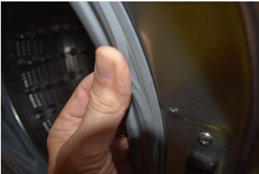
Photo #54 – The spring wire is hidden. There is one on the front panel and another on the drum.
