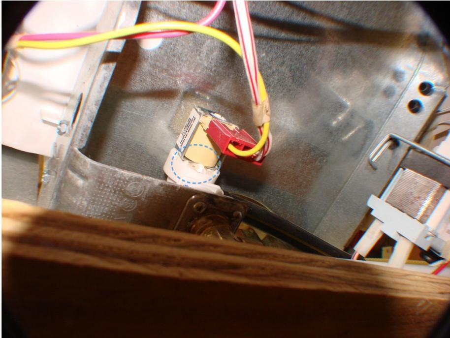
Photo #25 – An inlet valve leak between the solenoid (yellow) and the body (white) of the valve.
