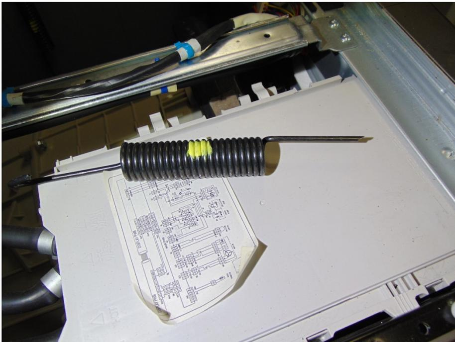
Photo #70 – This is the machine shown in Photo 50. One may have noticed that one of the two drum support springs was missing. It had failed in service.
