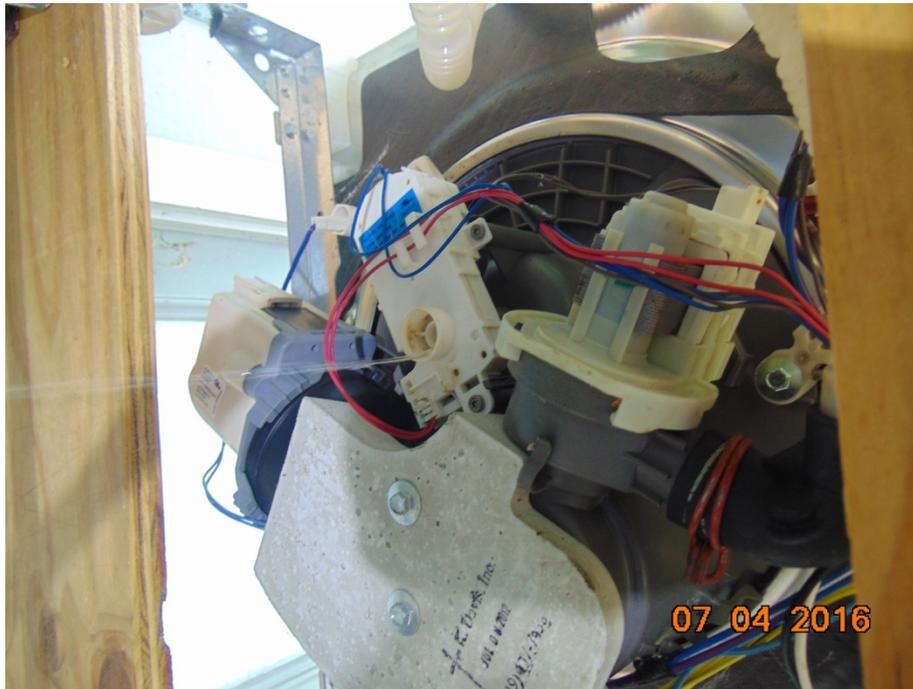
Photo #35 – Another water leak from a diverter.
