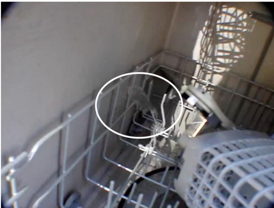
Photo #30 – This is a test in progress where water flowed into the tub when water pressure was applied without powering the machine. This is a bad inlet valve that is stuck open or otherwise damaged.
