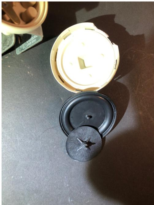
Photo # 43 – The diaphragm and the plunger. The diaphragm moves down as the water fill increases the pressure above the diaphragm to make contact at the adjusted set level of the switch.
