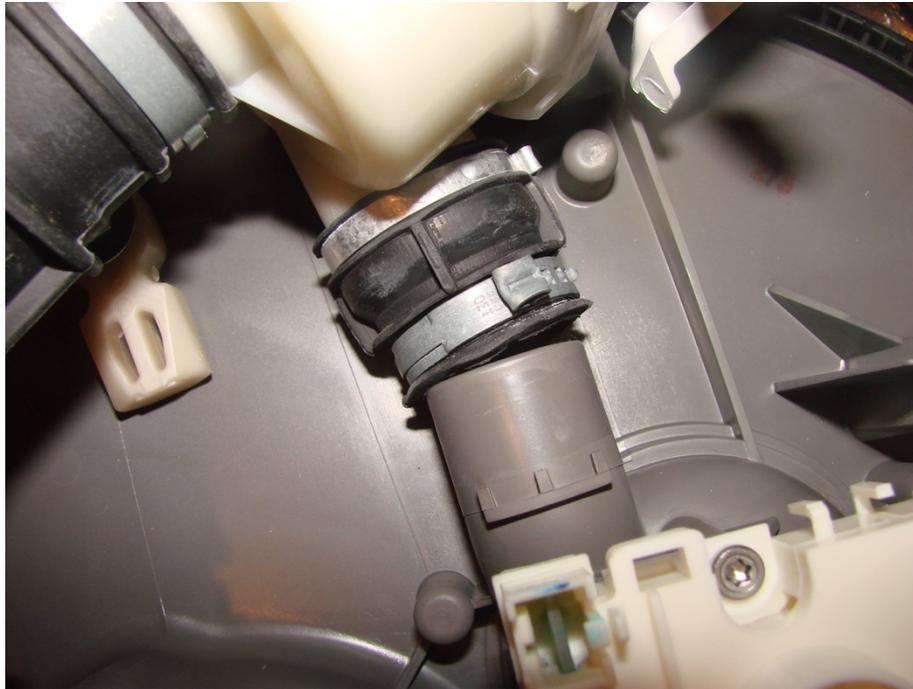
Photo #31 – This separation is a design defect in the connection. There is no resistance to axial movement.
