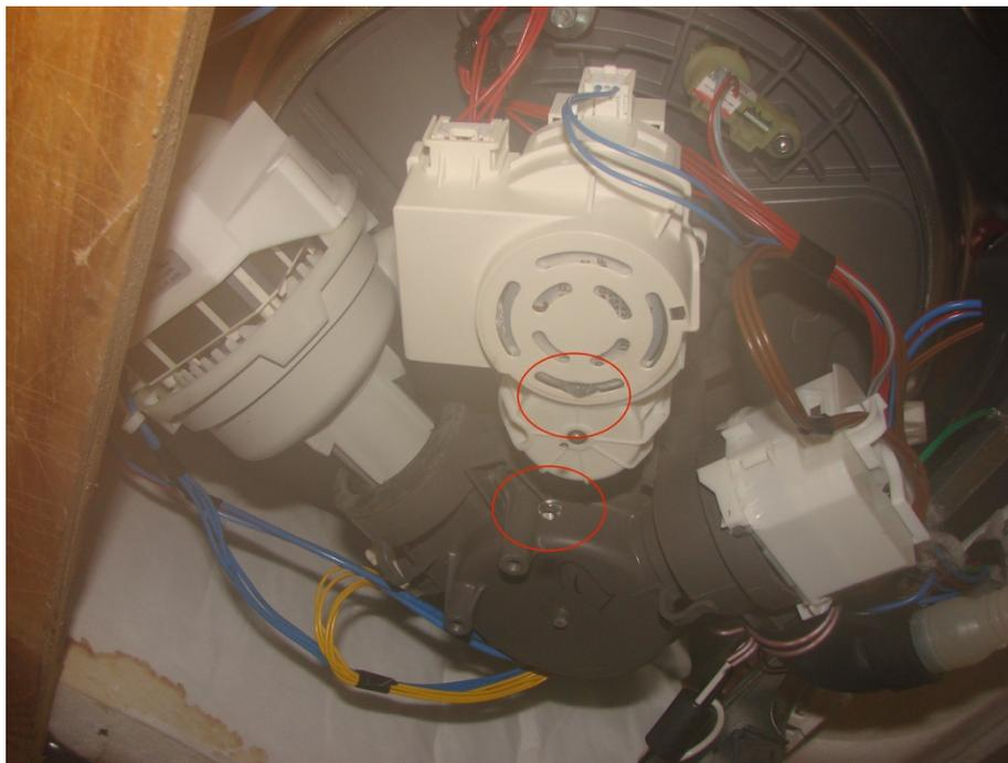
Photo #34 – A water leak from a diverter.
