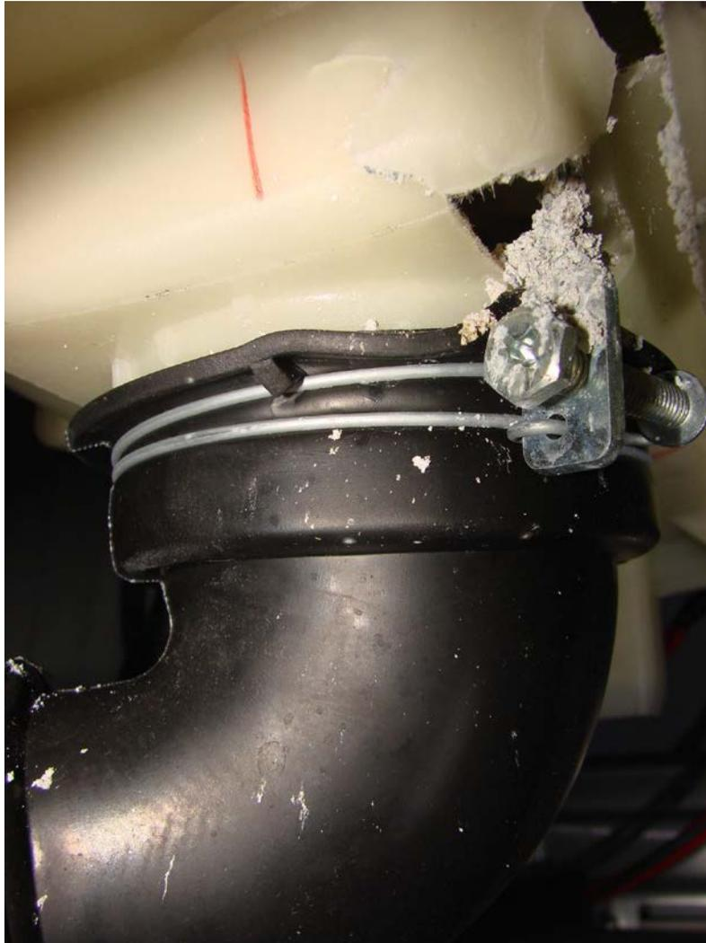
Photo #66 – This sump damage was found in a 4-month old washer.
