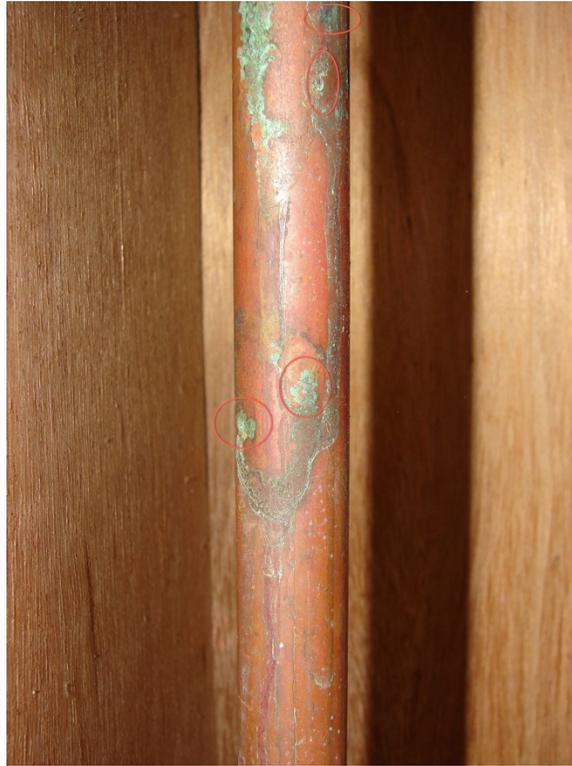
Photo #4 – Pitting corrosion in copper pipe.
