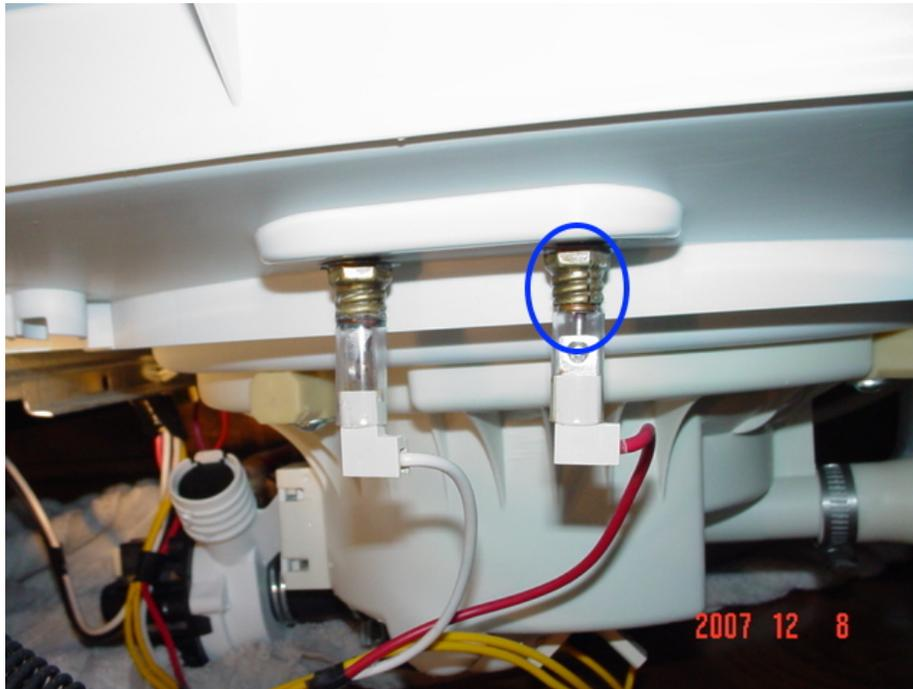
Photo #33 – This heater element penetration did not leak but the nut is cracked. The nut is not very robust.
