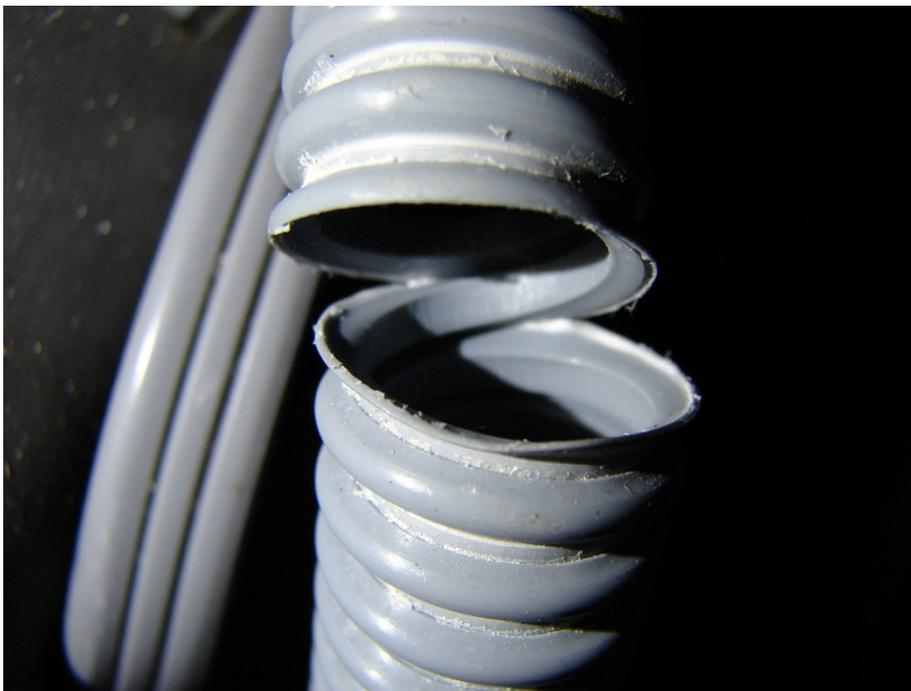
Photo #24 – This drain hose was at first thought to have been improperly run in the cabinet and kinked. Later we found that a caustic substance was likely associated with use of the dishwasher.
