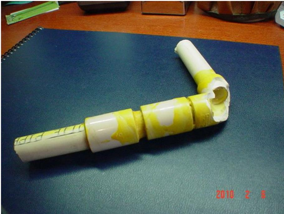
Photo #9 -- This is a section of CPVC pipe that froze in service. You can identify it by the solvent required and by its rigidity. This is not PVC as commonly used in drain lines.
