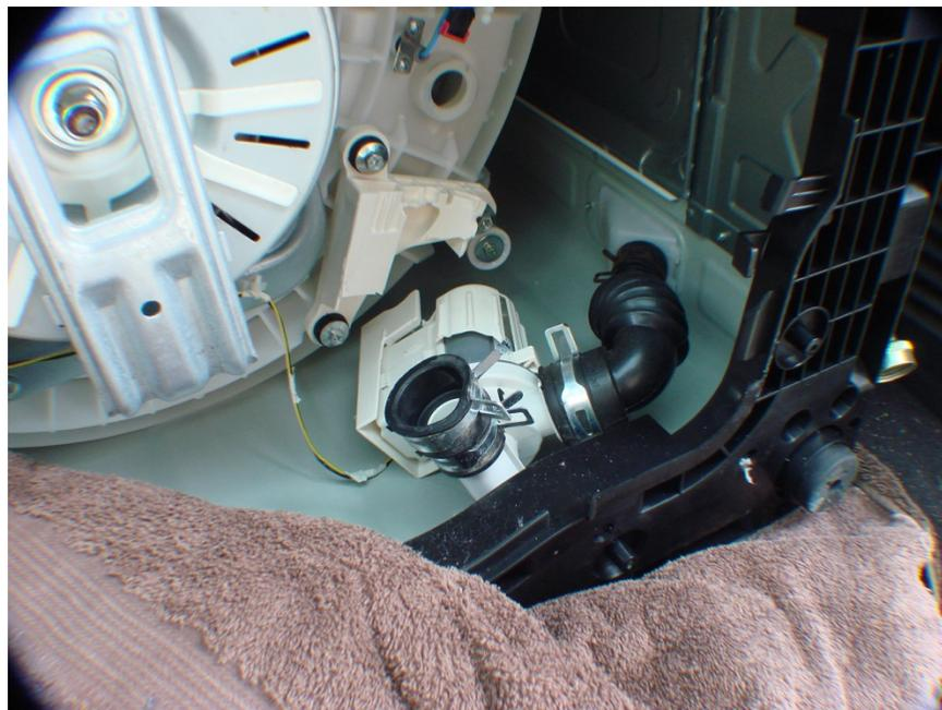
Photo #68 – This is a fractured pump bracket. The manufacturer attached the pump assembly to the tub, which vibrates in use. I have seen 4 cases of this same failure. The fix was to move the pump assembly to be supported on the frame of the machine. At failure, the pump assembly pulled the large hose connection off of the tub. The open nozzle is above at the top center of the photo.
