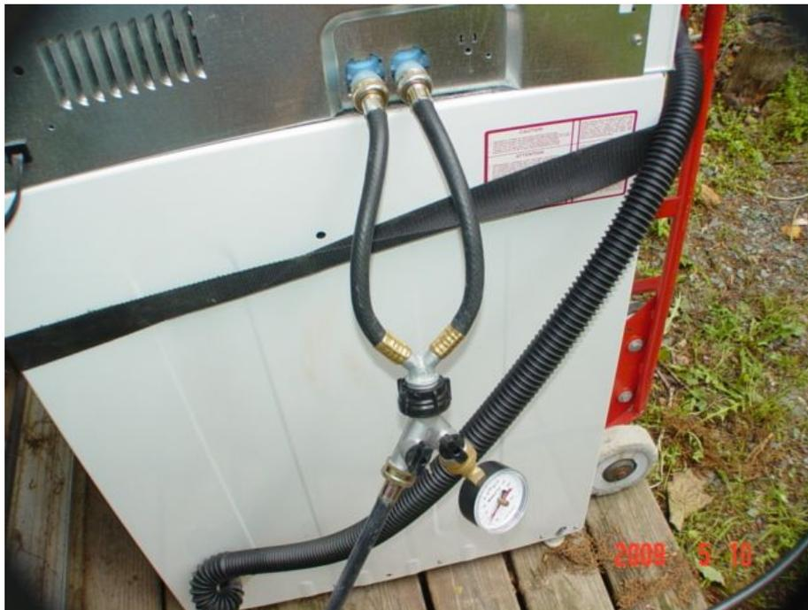
Photo #47 – This is the rig I use to remotely test a washer.
