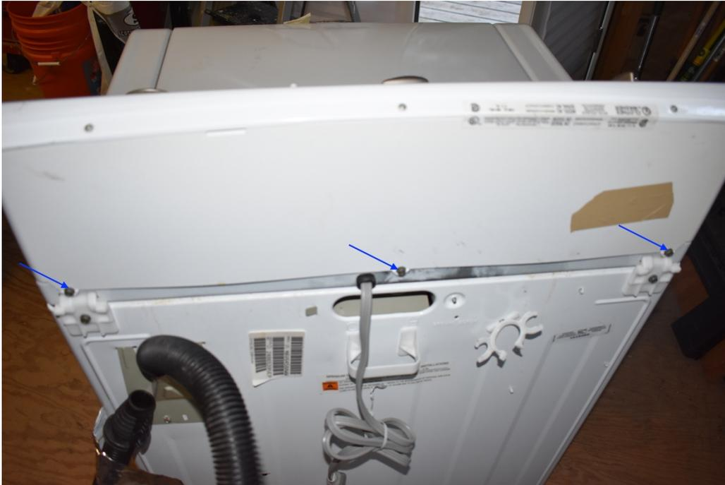
Photo #60 – On the back of the console are three screws. Removing these...
