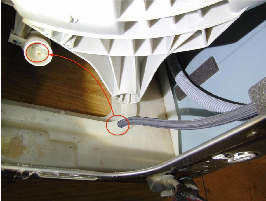
Photo #71 - When it failed, it pulled the pressure sensor air tube off the drum and caused a leak.
