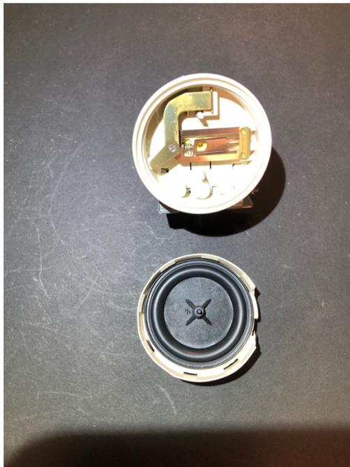
Photo # 41 - The pressure switch internals.
