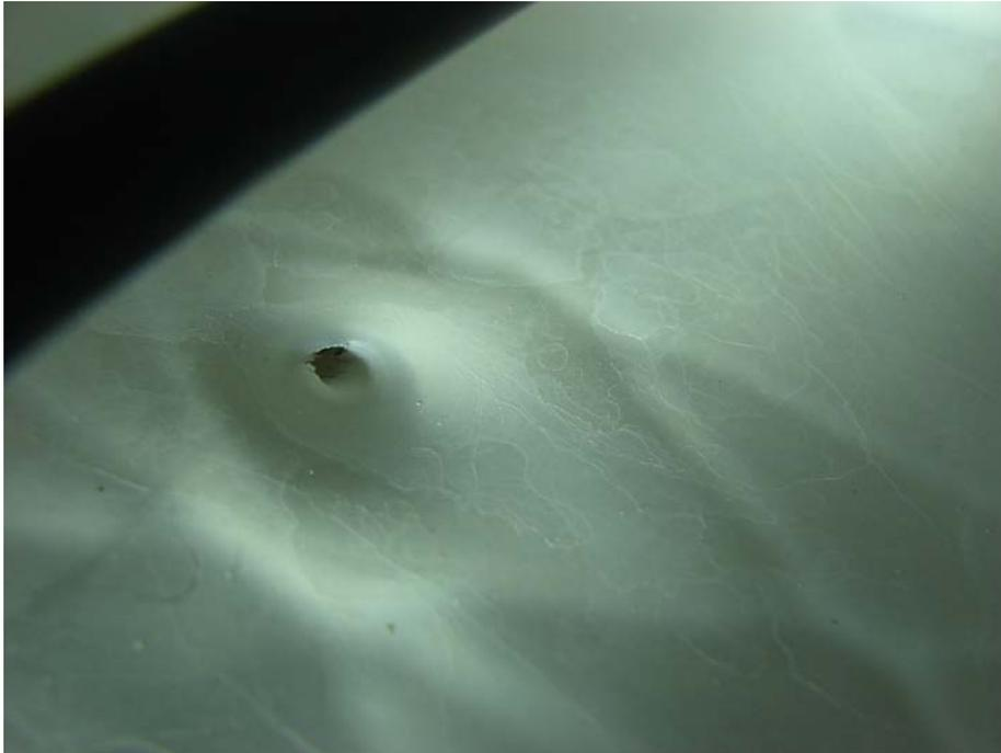
Photo #21 – This hole appeared in the floor of the tub, likely from excess heat from the heating element above. It is possible that a loose utensil contacted the element and the tub.
