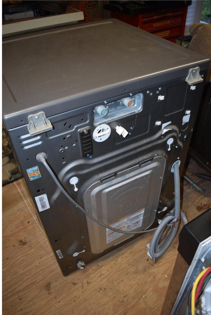
Photo #48 – This view of the rear of a front load machine shows the access panel and the hot/cold water inlet connections.
