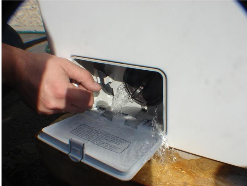
Photo #45 -- On certain front load machines there is a filter housing on the lower front panel. This plastic screw fitting was loosened without draining the sump to show that there is water remaining in the sump after a wash. Note small hose to the left that pulls out and would be used to drain the sump prior to opening the filter.
