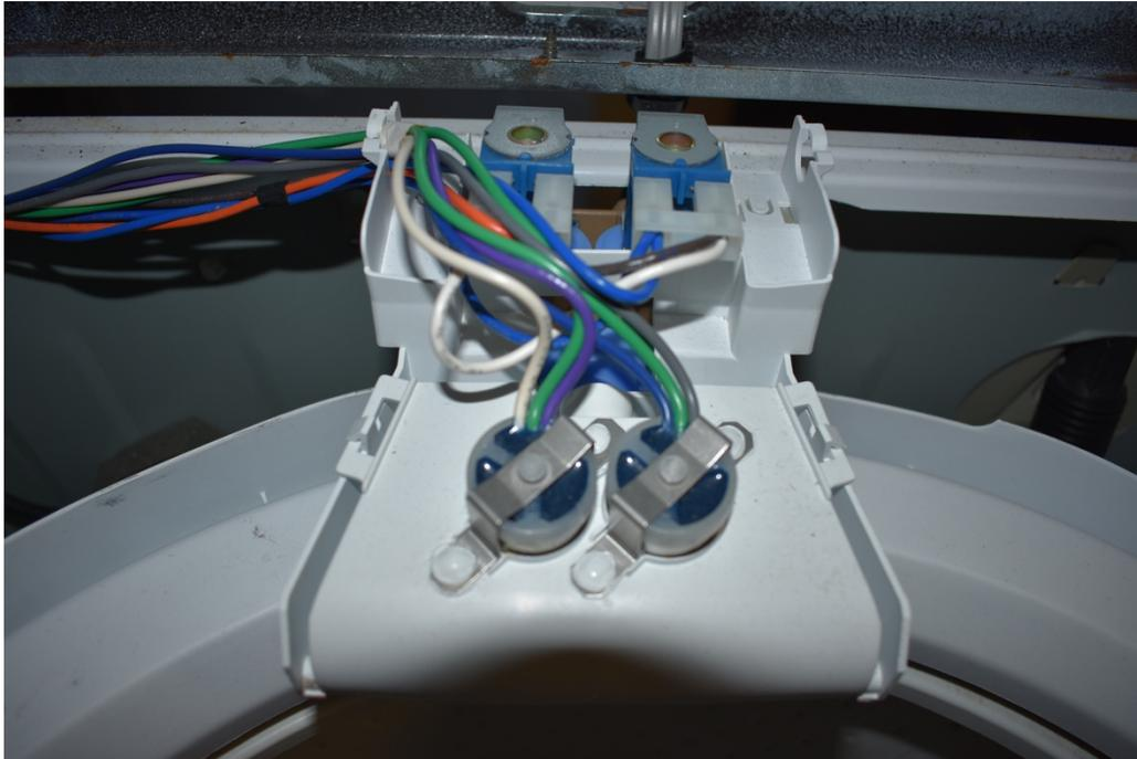
Photo #58 – The inlet valves. The devices to the bottom of the photo are thermostats.
