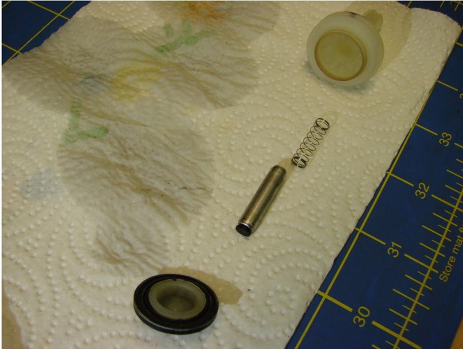
Photo #16 -- The parts of the upper section of the valve, diaphragm, plunger, spring and upper body. The tip of the plunger is rubber and seals the main orifice.
