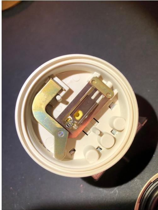
Photo # 42 – The electrical contacts are adjustable.
