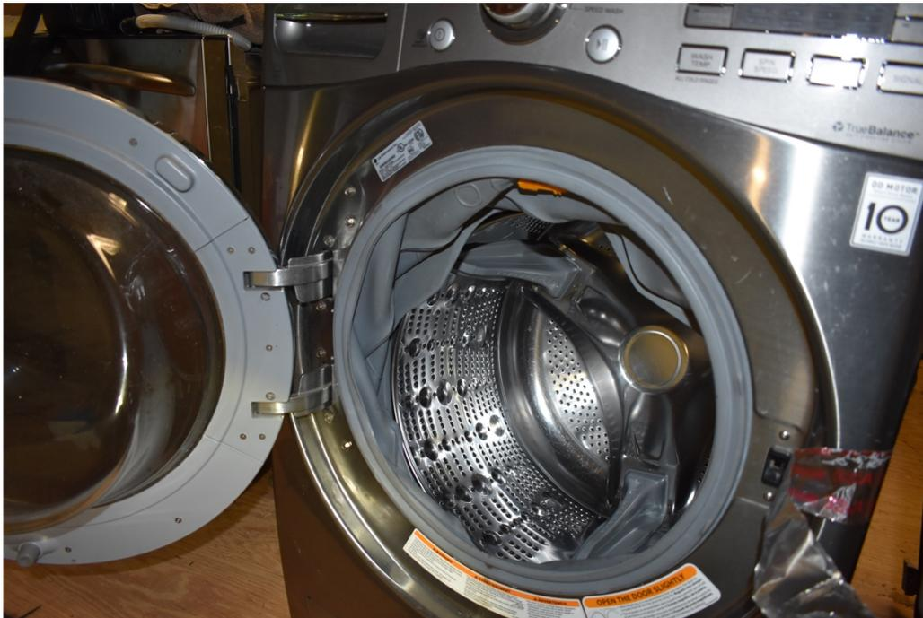
Photo #53 –The gray gasket connects the drum to the front panel of the machine. This can fail due to mechanical damage or the spring wire that attaches it to the machine can fail.
