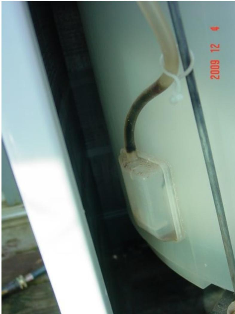
Photo #63 – This air tube is filled with debris and the rising air pressure as the tub fill can't be sensed by the pressure sensor in the console. Therefore, the inlet valve flow will not shut off and an overflow occurs.
