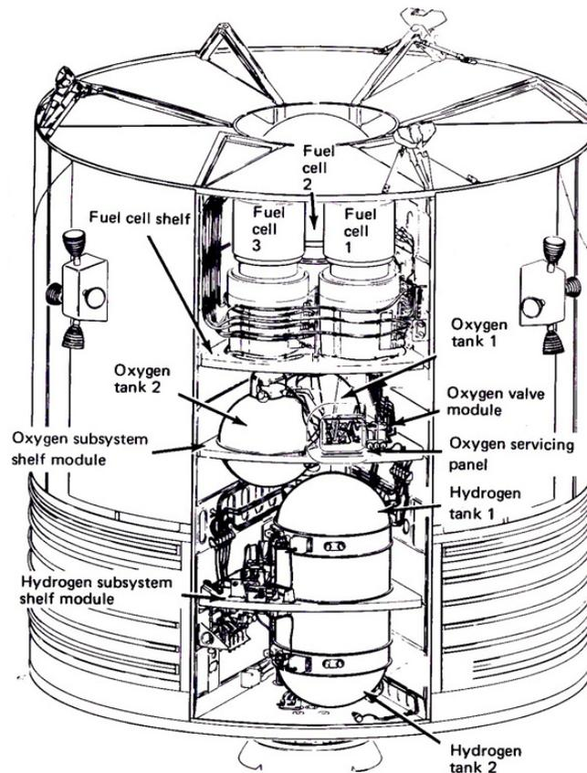
**Figure 2.8: Apollo Oxygen Tanks**
