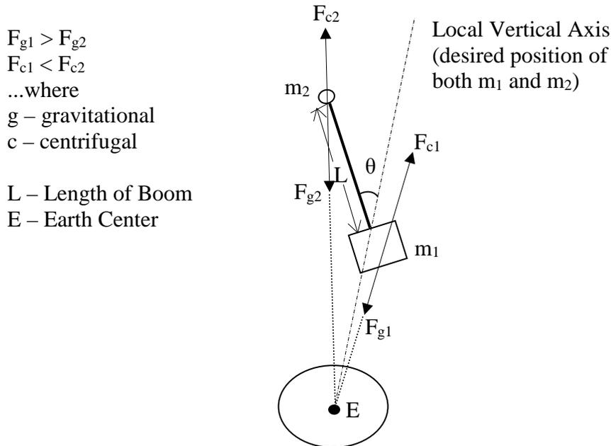
**Figure 2.6: Gravity Gradient Forces**
