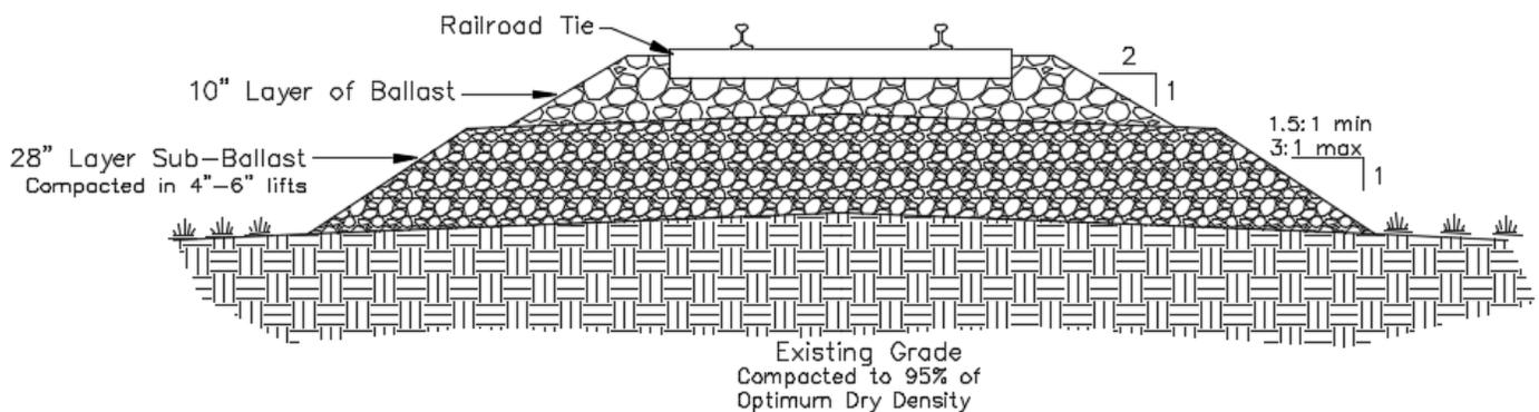
Figure 10 - Example for Heavy-Duty Track Cross-section
