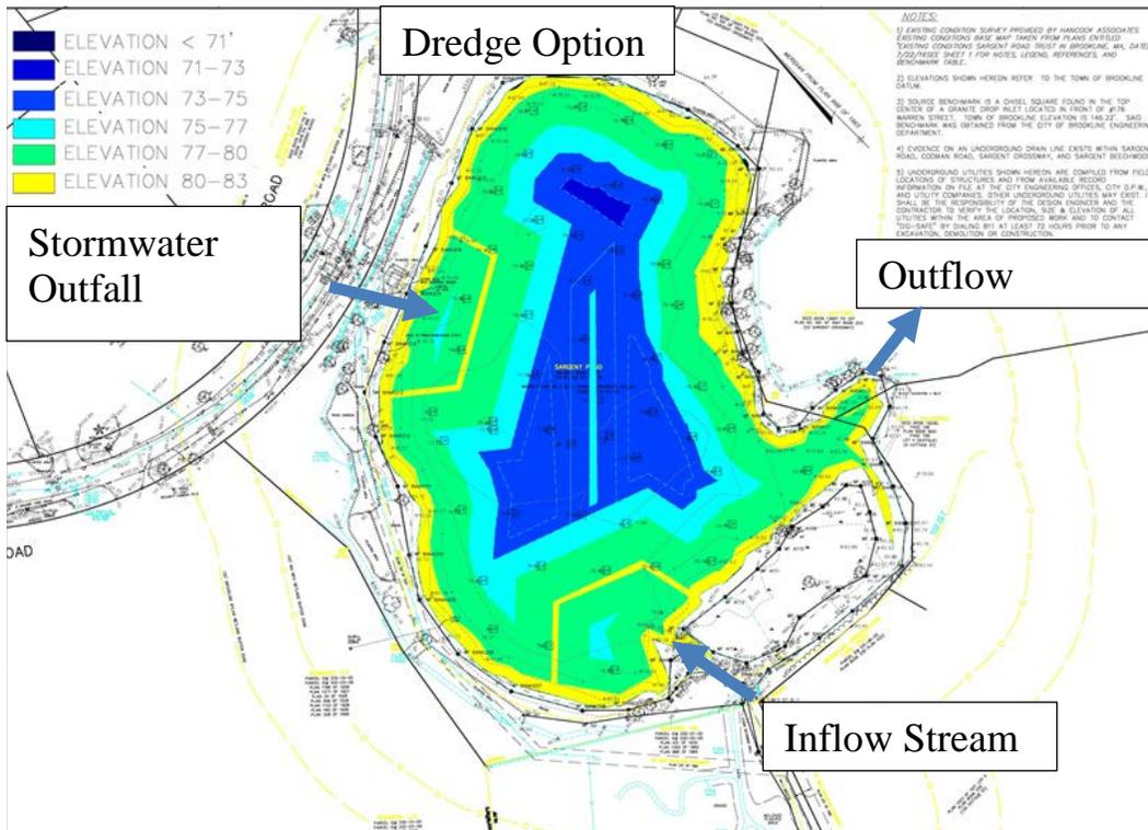
Option 2 still increases your depth in the center of the pond, getting 9 ft water depth in the north and 7-8 feet towards the middle of the pond, excluding the ridge. This option involves removing less volume of sediment than option 1. This option does however help to increase the flow and circulation in the pond towards the north.
