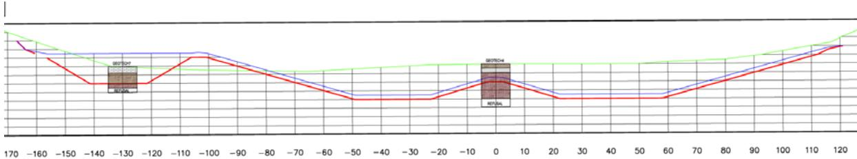
Cross-Section View with Sediment Samples overlain
