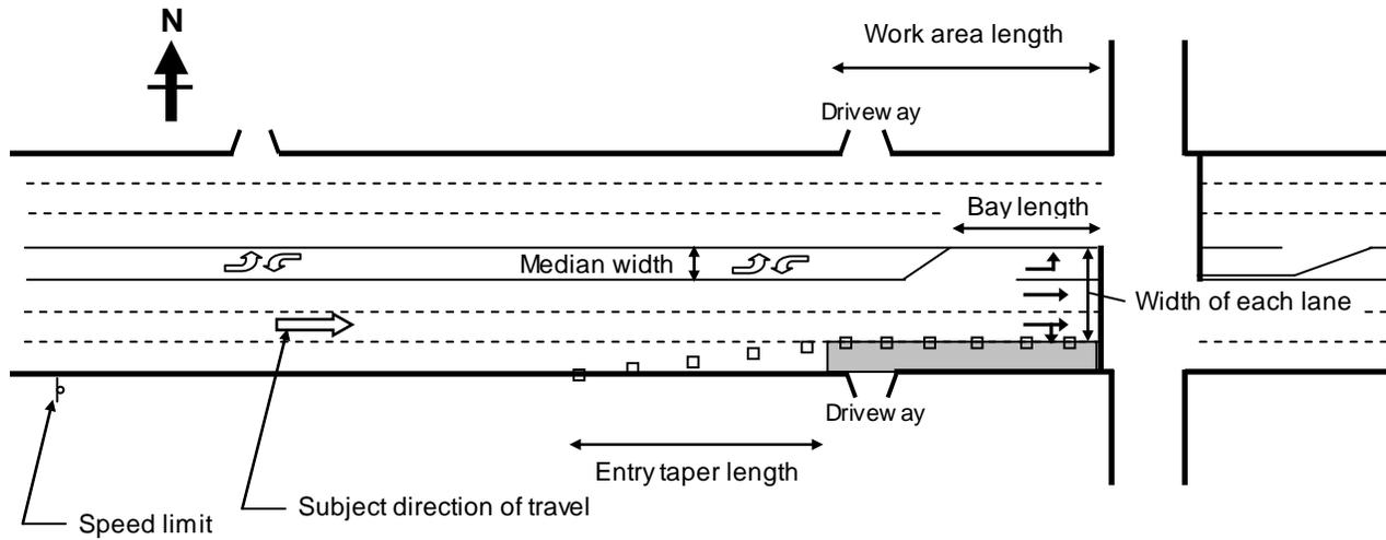
Figure 20. Work zone presence at approach to signalized intersection
