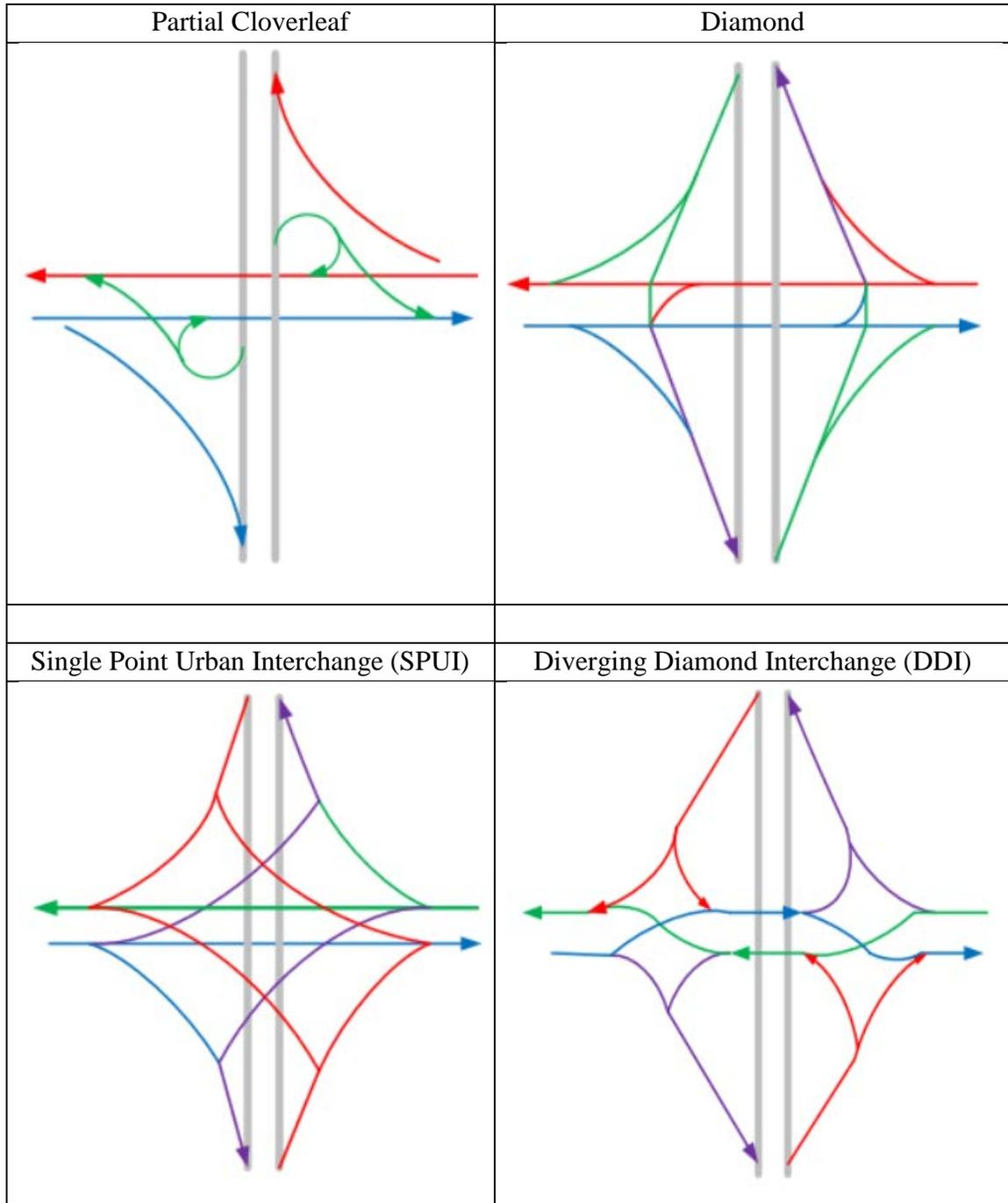
Figure 22. Ramp Terminal Forms
