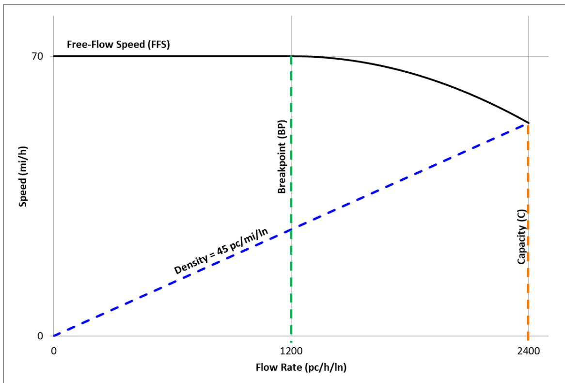
Figure 8. Unified speed-flow equation
