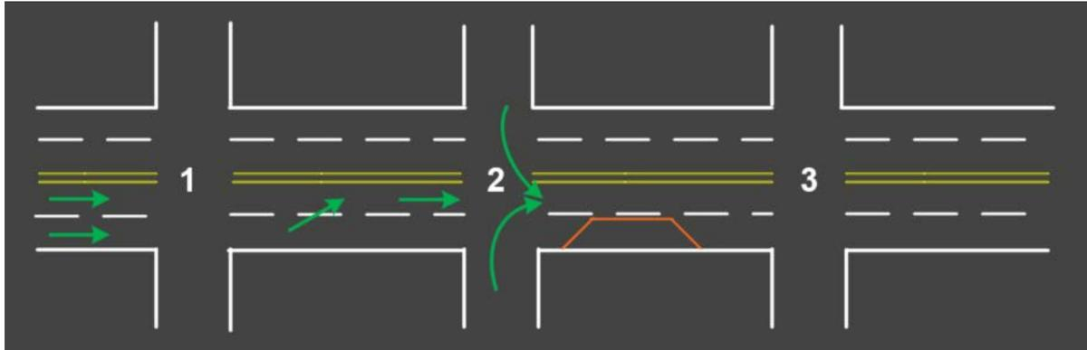
Figure 16. Midsegment Lane Blockage Dipiction
