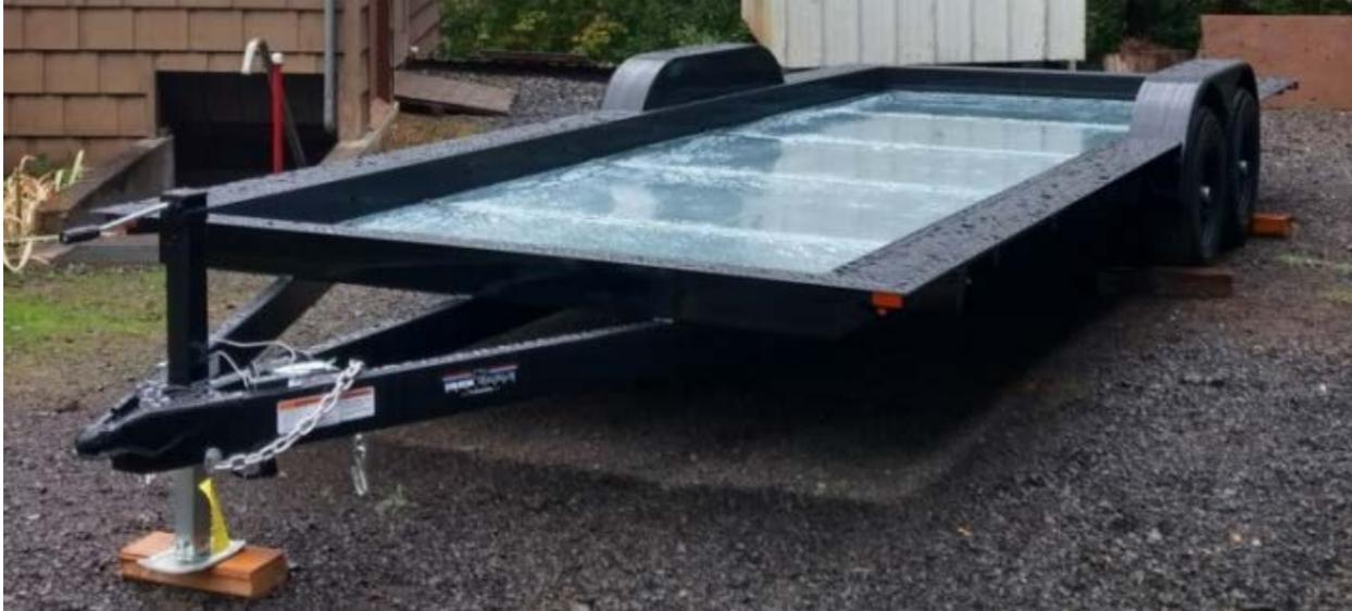
**Tiny house specific trailer with galvanized sheet metal bottom pan to protect the floor assembly from water and insects**
