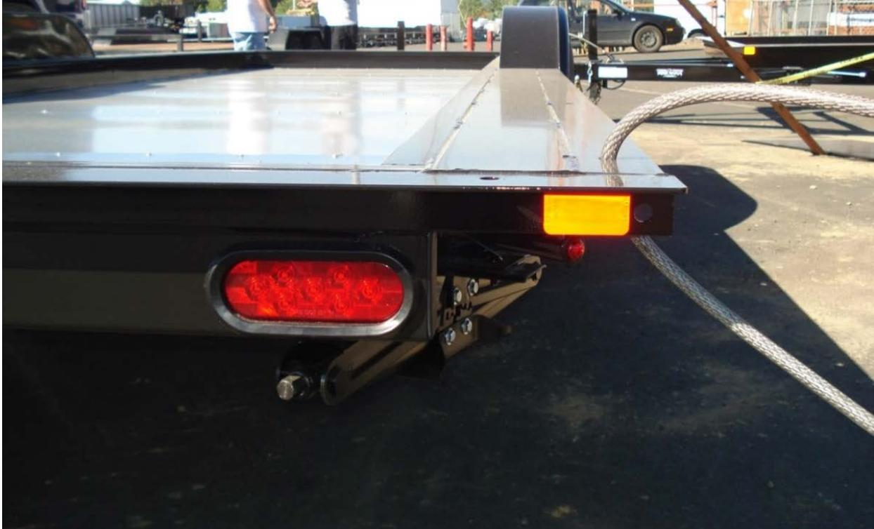
**One of four corner scissor jacks welded to the trailer frame for quicker leveling of the trailer. A nice feature if the THOW will be moved often.**
