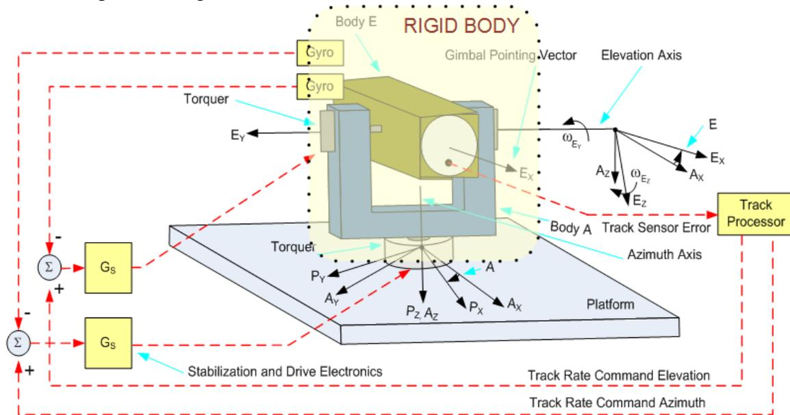
Figure 11.0 the 2-Axis Gimbal Configuration Highlighting Rigid Body Elements
