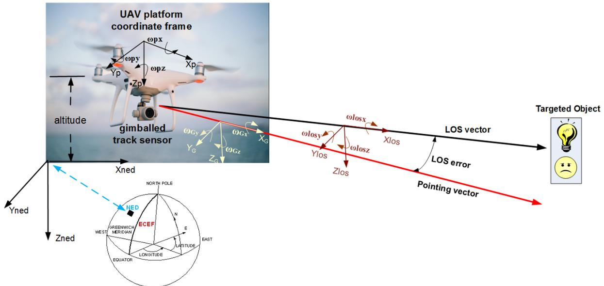
Figure 23.0 Typical coordinate frame geometry for geo-location
