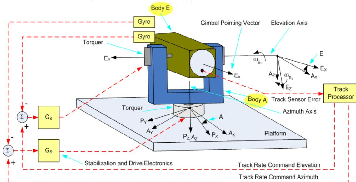
Figure 2.0 Simple 2-axis Elevation over Azimuth Gimbaled Track Sensor Geometry
