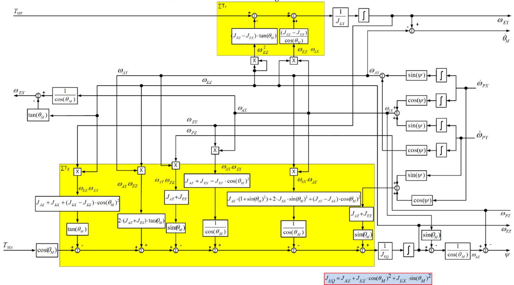
Figure 14.0 Two -Axis RBE Block Diagram
