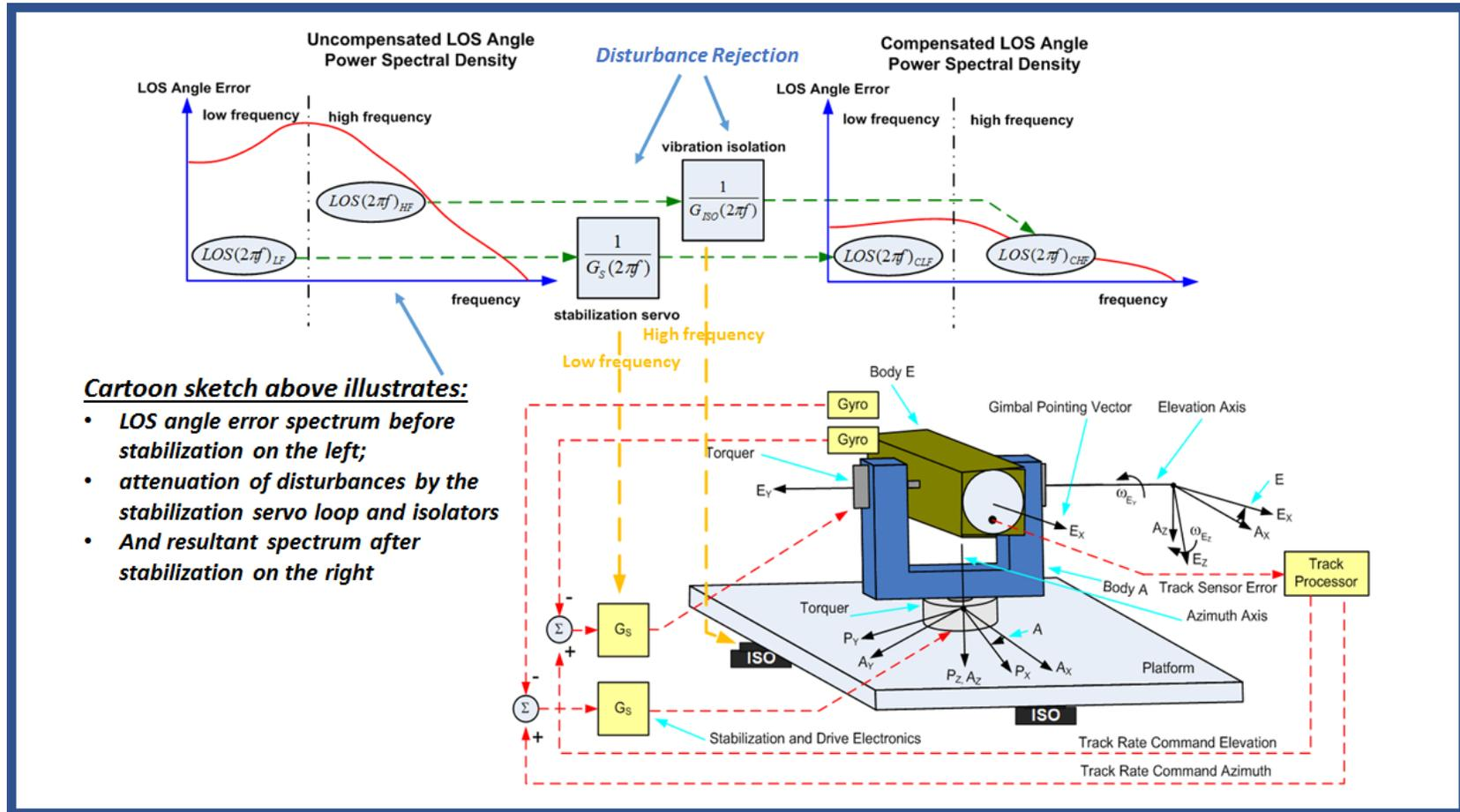
Figure 4.0 SLC System Disturbance Rejection
