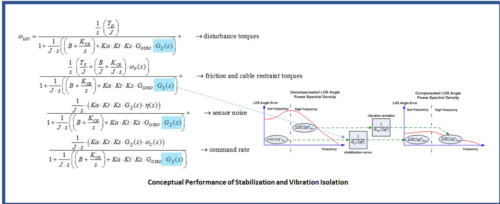
Figure 10.0 SLC LOSR Feedback Equation Mapped back to Disturbance Error
