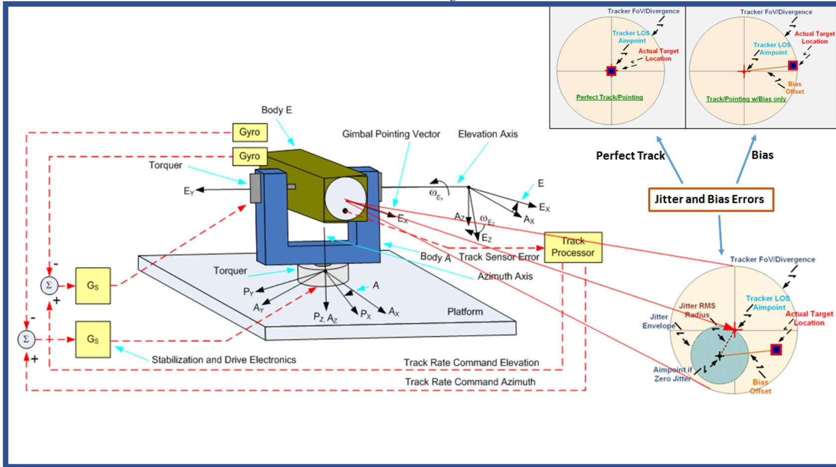
Figure 5.0 Illustration of Jitter and Bias Pointing Error
