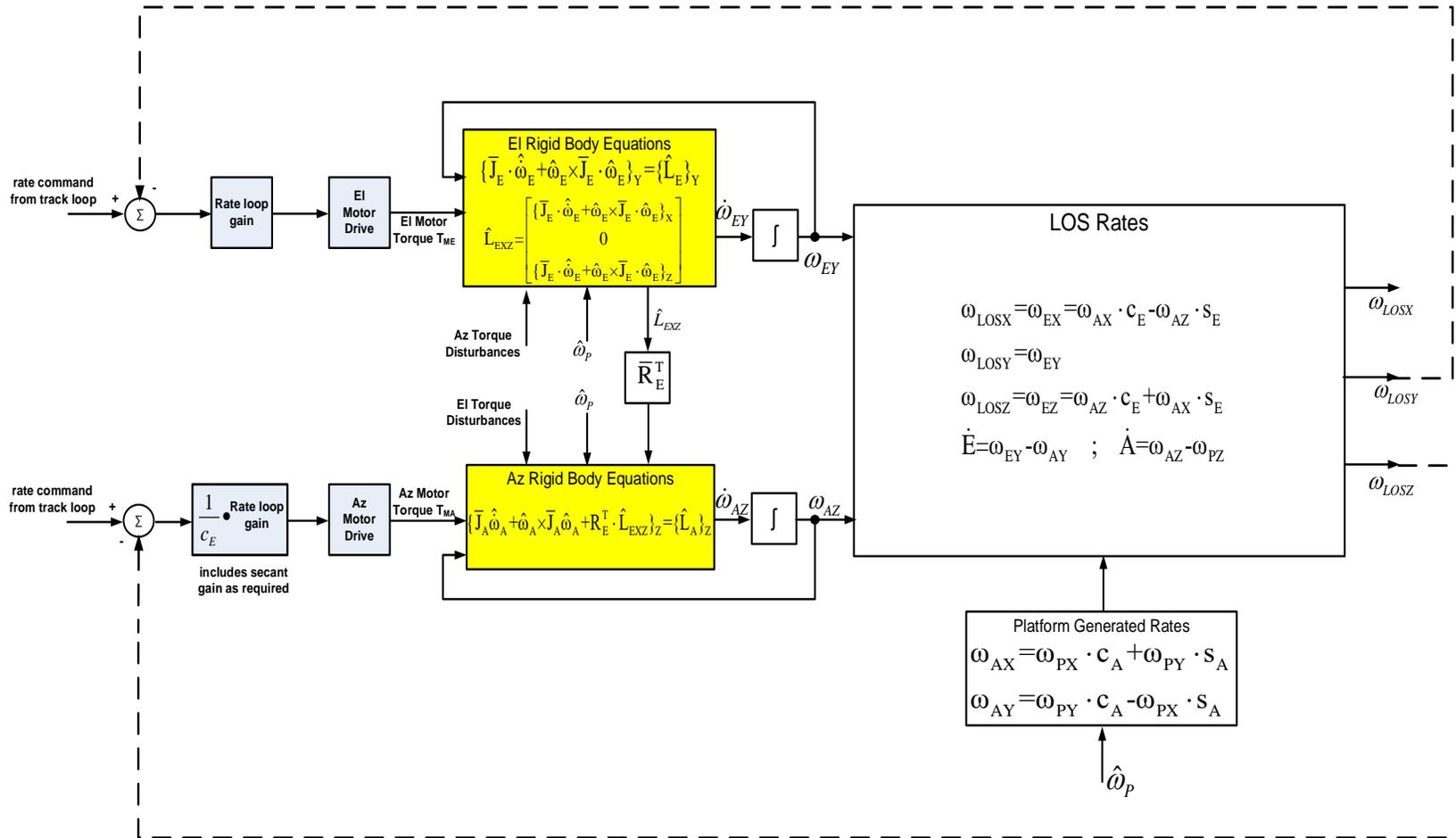
Figure 16.0 Two -Axis Gimbal LOS Rate Feedback Control Loop
