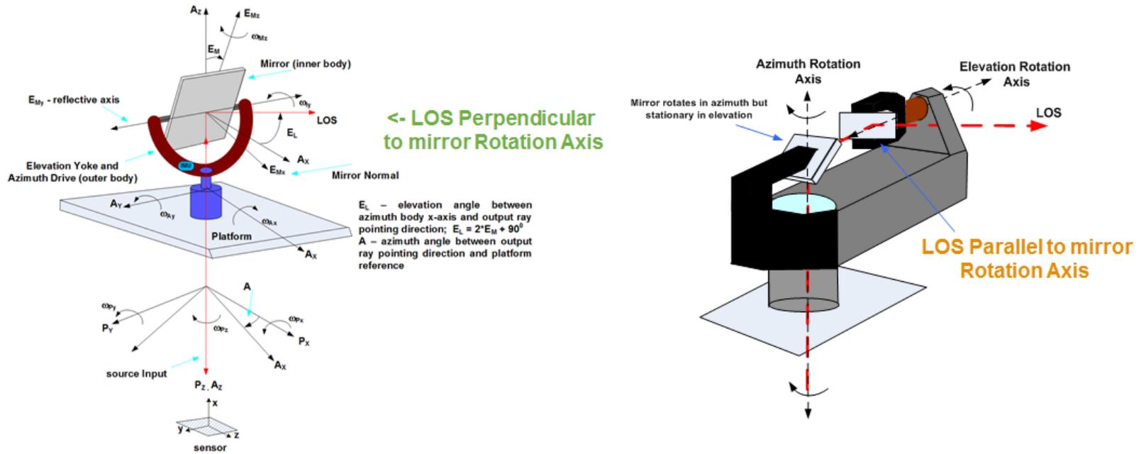
Figure 20.0 Two mirror rotation configurations; Left: simple El/Az with 2:1 OAG; Right: 2 mirror offset without OAG
