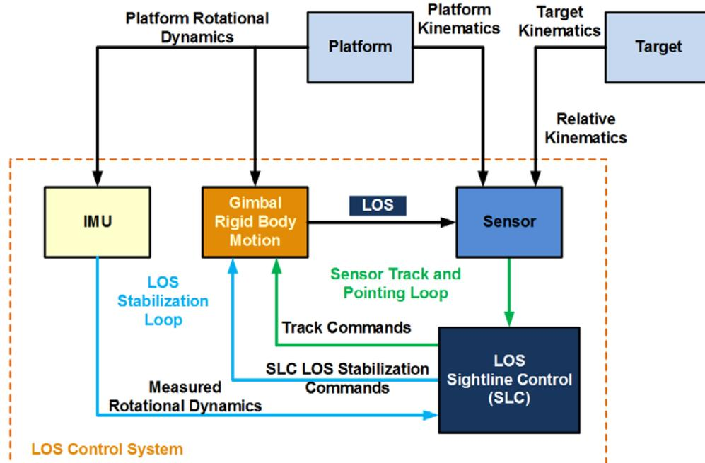
Figure 3.0 High Level SLC System Architecture
