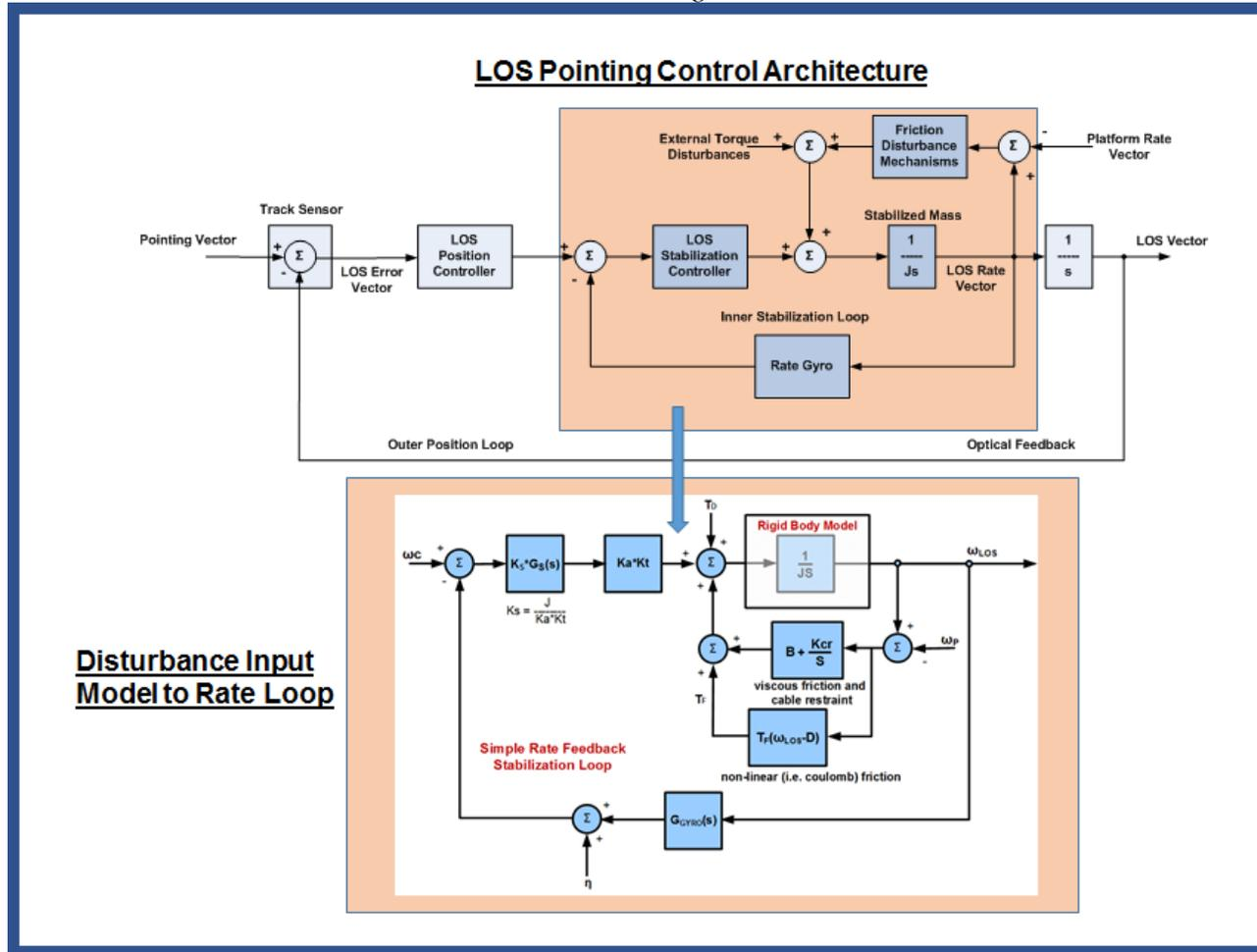
Figure 9.0 SLC Control Configuration and Disturbance Input Model
