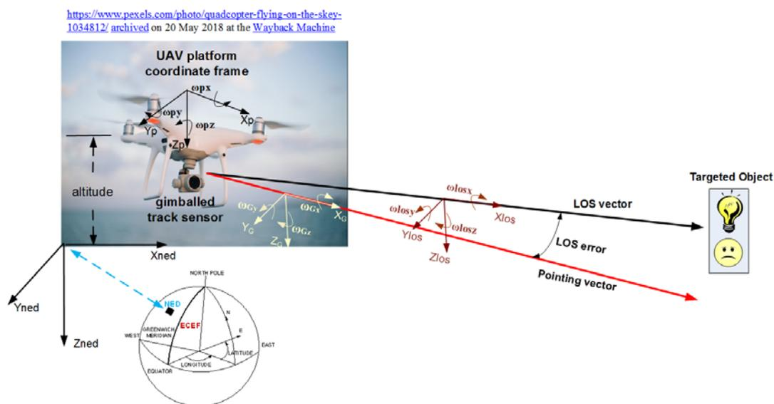
Figure 3.0 Typical coordinate frame geometry for geo-location
