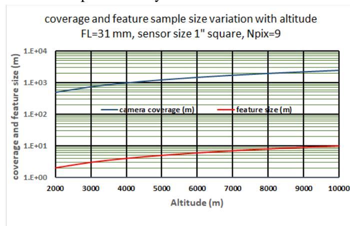
Figure 7.0 Feature sample size (nominal design 2 m) and coverage variation with altitude
