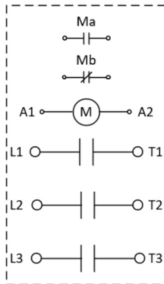
Figure 2: Contactor Terminal Identification
