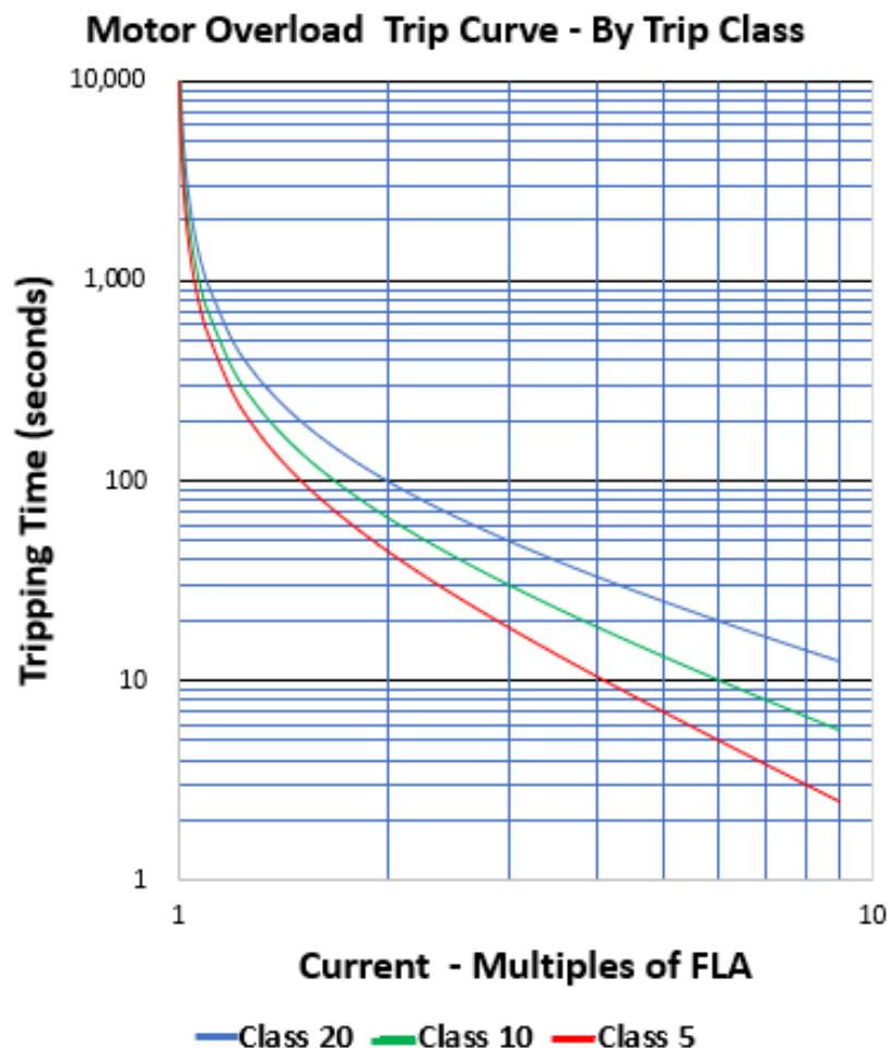
Figure 5: Tripping Class time-current curves
