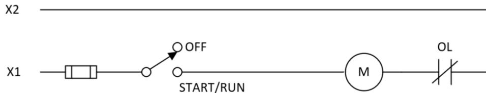
*Figure 3: Two-Wire Control Circuit*
